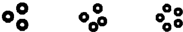
Fig. 2. Optimal configurations with criterion c' for three, four, and five telescopes (see Table 2).
