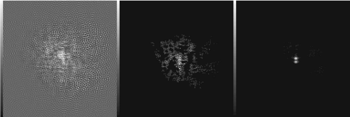
Fig. 6. Restored object with conventional methods: MAP wave-front estimation followed by a multiframe Wiener filter (left); MAP wave-front estimation followed by a quadratic restoration with a positivity constraint (center), to be compared with the object restored by the myopic deconvolution (right), with use of the same quadratic regularization and the same positivity constraint.
