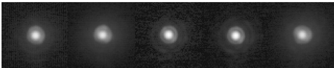
Fig. 1. Five experimental VLT-NAOS-CONICA images of an unresolved bright star recorded on Sep. 29, 2002, at 20:58 UT in the Br \gamma narrow band and used in the simulations (wavelength \lambda = 2.166 \mu\text{m} , exposure time 2 s). The fourth one is used as the true PSF. The estimated Strehl ratios are 57%, 52%, 64%, 66%, and 58%. The corresponding Fried parameters are r_0 = 17.5, 15.6, 20.7, 21.0 and 17.0 cm.
