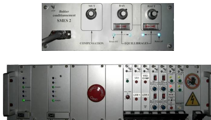
Figure 4-32: Detection bridges (above) and process control device (below)
