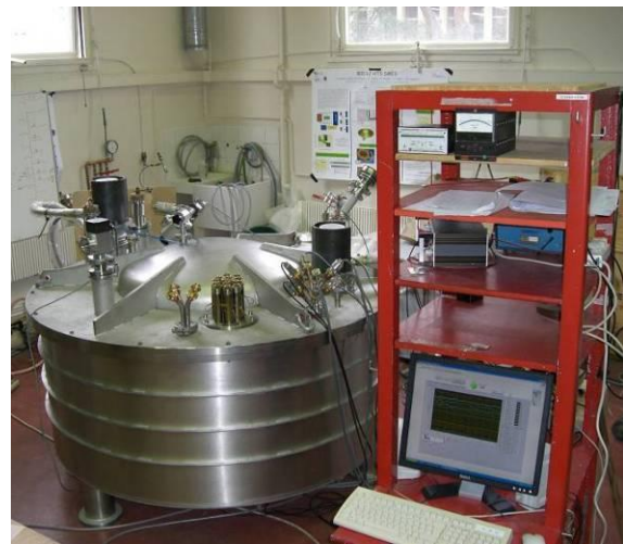
Figure 3-1 : SMES I demonstrator under test
