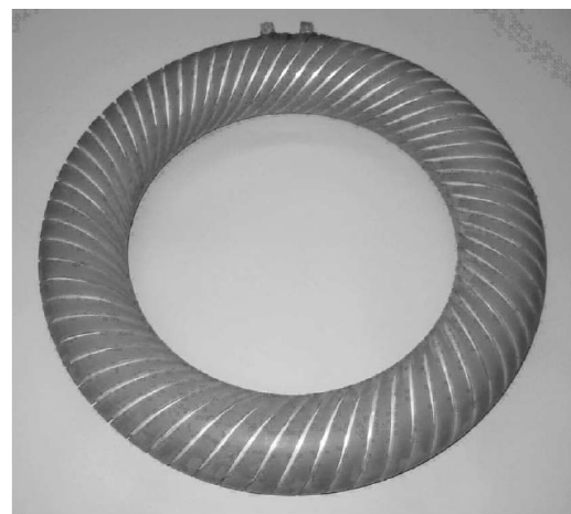
Figure 1-16: Force-balanced toroid with variable pitch winding [NWS+05]
