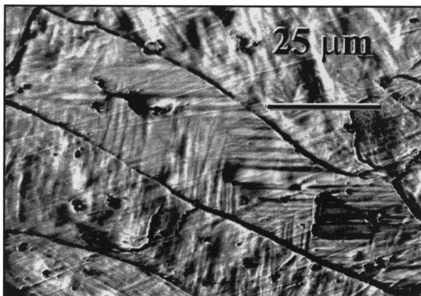
Fig. 12. Micrograph of a cast ZrAu sample. The typical martensitic-like aspect has been revealed after etching in a ( \text{HCl} , \text{HNO}_3 , \text{H}_2\text{O} ) solution.
