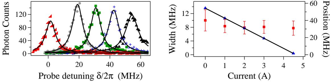
**Figure 5.13: MOT coil calibration.** *left*) Dependence of the number of detected photons on the probe frequency around the  $F=2, m_F=+2 \rightarrow F'=3, m'_F=+3$  transition. The dependence is shown for a current of 0, 1, 2, 3, 4.5 A (from right to left) in the MOT coils. *right*) Center position and width of the atomic distribution versus the MOT current.
