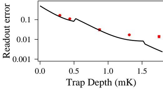
**Figure 7.16: State detection fidelity.** Dependence of the read-out error on the trap depth. As the trap depth increases we can scatter more photons without losing the atom (The atom loss is held constant at 2 %). The black line corresponds to a theoretical model described in the text.
