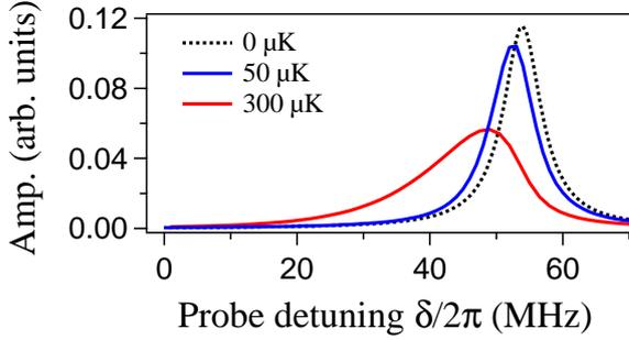
**Figure 5.3: Light-shift distribution  $D_s(\delta)f_{th}(\delta)$  for a thermal atom in a trap of 2.7 mK.** Light shift distribution depending on the potential energy and thus the probe frequency  $\delta/2\pi$ . For an atom at 0  $\mu\text{K}$  it has a Lorentzian shape. For higher temperatures the maximum shifts as  $\frac{3}{2}k_B T$  and broadens. The curves are calculated by using a probe saturation of  $s = 0.3$ .
