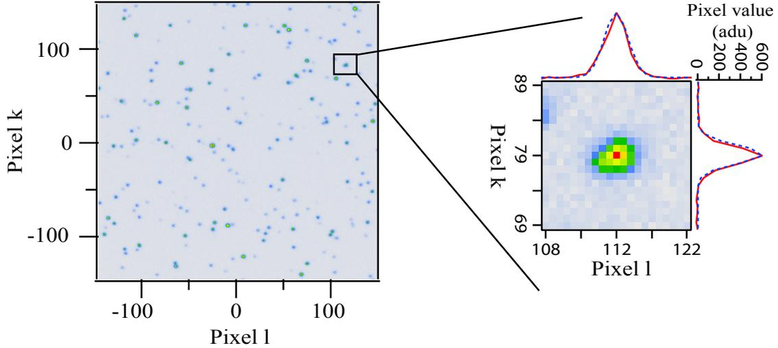
**Figure 4.3: Image showing photon events for a gain of 8.** A typical image showing photon events for a gain 8. The region of interest corresponding to the image size is  $\text{ROI} = 300 \times 300$  pixels. The average number of events per image is  $\bar{N}_{\text{events}} \sim 240$ . Looking at the cross-sections of one event we see that the event is well fitted by a Gaussian function (blue dashed line) with a rms width of  $\sigma = 1.2 \pm 0.2$  pixel.
