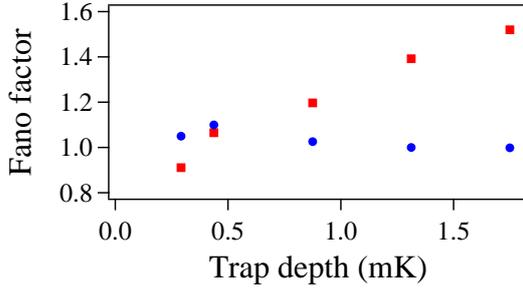
**Figure 7.11: Fano factor.** Fano factor of the bright (red squares) and dark (blue circles) distribution versus the trap depth. The background Fano factor is close to one and compatible with a Poissonian distribution. For the bright distribution it increases linearly indicating a broadening for higher trap depths.
