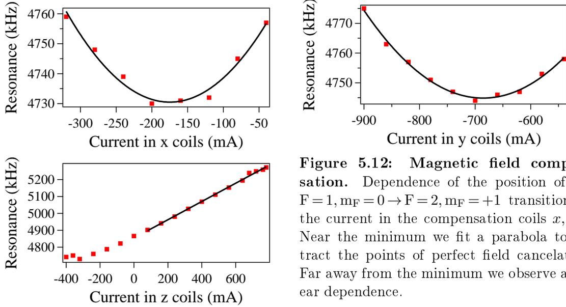
**Figure 5.12: Magnetic field compensation.** Dependence of the position of the  $F = 1, m_F = 0 \rightarrow F = 2, m_F = +1$  transition on the current in the compensation coils  $x, y, z$ . Near the minimum we fit a parabola to extract the points of perfect field cancelation. Far away from the minimum we observe a linear dependence.
