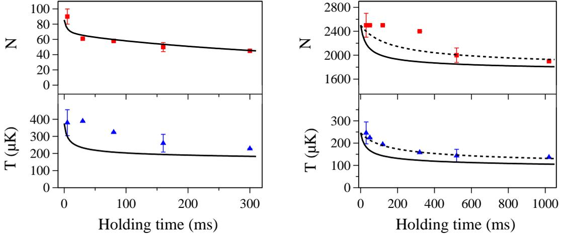
**Figure 10.1: Free evaporation in micro and macro trap.** We show the evolution of the average atom number  $N$  and temperature  $T$  of the atom ensemble loaded directly from the MOT into the *left*) 2.7 mK deep micro and *right*) 1.4 mK deep macro trap. The black solid and dotted curves are a simulation described in the text.
