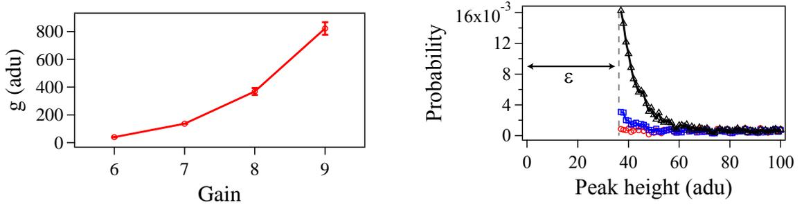
**Figure 4.8: Intensifier gain and beginning of histograms for gain 9.** *left*)  $g$  is plotted for different intensifier gains. The intensifier response is clearly nonlinear. *right*) Initial part of the events histogram for gain 9 in Fig. 4.7. We compare the distributions for isolated (red circles), post-selected (blue squares) and all (black triangles) events for small amplitudes.
