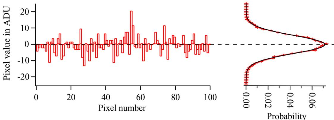
**Figure 4.2: CCD noise characteristics.** Cross-section through a CCD image of  $100 \times 100$  pixels without any incoming photon event. The noise distribution has a Gaussian shape with a rms width of 5.6 adu. It comprises clock induced charges as well as read-out noise. A constant dark current offset of 622 adu has been subtracted.
