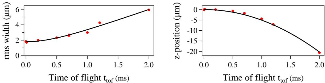
**Figure 11.7: Time-of-flight experiment with an ultra-cold atom cloud.** *left*) We plot the rms width of the cloud dependent of the flight time. We extract a temperature of  $T = 80 \pm 24$  nK. *right*) The cloud center position in  $z$ -direction is shown versus the flight time. We fit the parabola  $z = -\frac{1}{2}g \cdot t^2$  to the data and extract an earth acceleration of  $g = 10.1 \pm 0.3$  m/s<sup>2</sup>.
