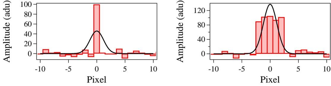
**Figure 4.5: Example of non-Gaussian events.** *left*) A Gaussian fit (with fixed rms width  $\sigma = 1.2$  pixel) of a thin event yields a lower peak height  $H_{0,0}$  than the real pixel value  $H_{k_0,l_0} < D(k_0, l_0)$ . For such peaks the “sharp” value is usually greater than one. *right*) A small “sharp” value  $0 \lesssim \text{“sharp”} \ll 1$  can be found for events that are somewhat broader than the Gaussian function.
