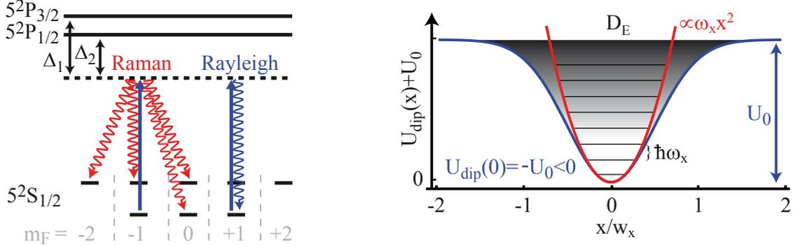
**Figure 1.8: Difference between Raman and Rayleigh scattering.** Gaussian dipole trap potential *left*) Rayleigh scattering does not change the internal state of the atom while Raman scattering changes the internal state. *right*) Gaussian dipole trap profile with harmonic approximation for an attractive potential.
