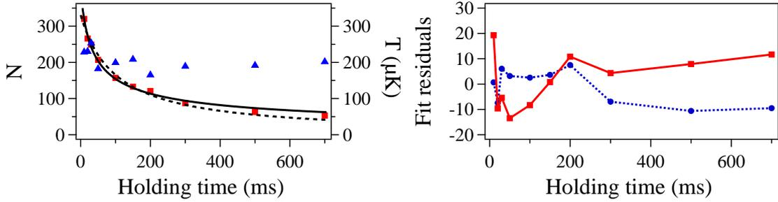
**Figure 10.5: Three body loss rate.** *left*) We plot the number of atoms  $N$  (red squares) and temperature  $T$  (blue triangles) versus the holding time in the micro trap. A two-body (dashed black line) and three-body (solid black line) fit are compared to the data. *right*) We plot the difference between the data and the two-body (red squares) and three-body (blue circles) fit result versus the holding time.
