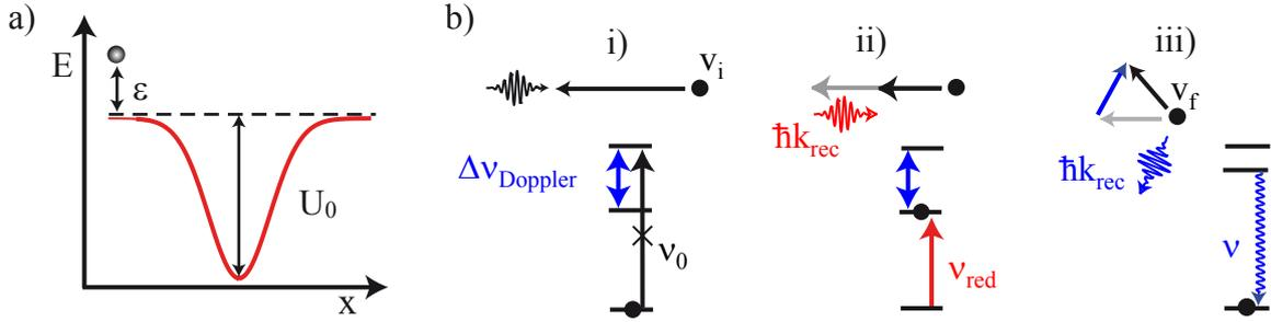
**Figure 3.1: Principle of trap loading and laser cooling.** *a)*  $x$  cross-section of the dipole trap potential. *b)* Principle of laser cooling based on the Doppler-shift, photon absorption and reemission processes.
