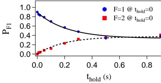
**Figure 5.7: Measurement of the trap-light induced Raman transitions.** The single atom recapture rate is measured versus the holding time  $t_{\text{hold}}$ , during which the trap induces hyperfine changing Raman transitions. A fit is used to extract the Raman transition rates for an initial preparation in  $5^2S_{1/2}F=1$  (blue circles) and  $5^2S_{1/2}F=2$  (red squares).
