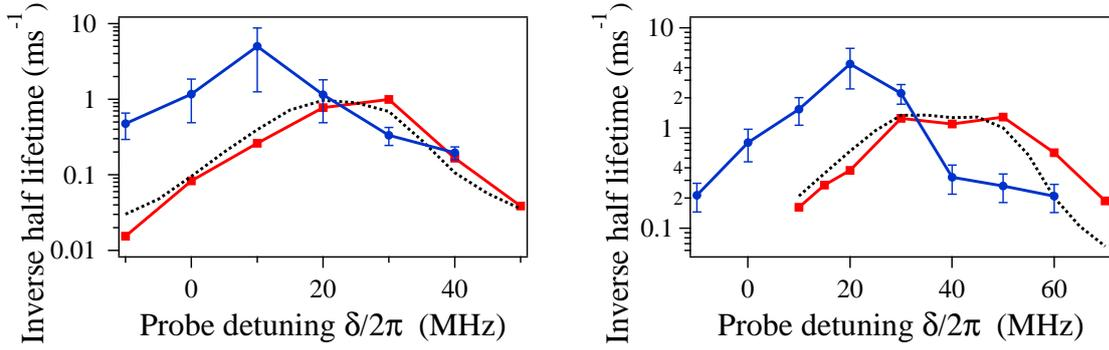
**Figure 9.8: Half life time dependent on the probe frequency.** We compare the inverse half lifetime of a single atom (red squares) and of three atoms (blue circles) versus the probe detuning for a fixed probe saturation  $s \sim 0.5$ . The black dotted line is the single atom result adjusted to the many atom ensemble temperature. The trap depth is *left*) 0.9 mK and *right*) 1.8 mK.
