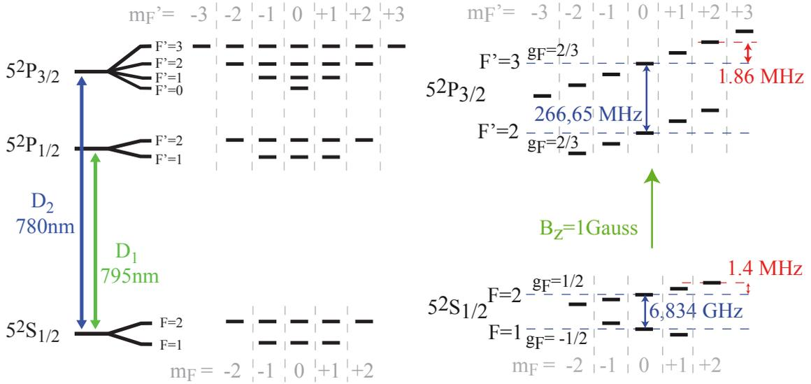
**Figure 1.2: Zeeman sub-structure and magnetic field-induced shifts.** *left)* Hyperfine and Zeeman level structure of the  $D_1$  and  $D_2$  transitions. *right)* Zeeman level shifts induced by a static external magnetic field along the quantization axis  $B_z$ .
