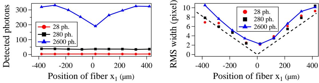
**Figure 4.11: Intensifier nonlinearity.** *left*) Dependence of the detected power on the CCD camera versus the laser fiber coupler position  $x_1$  for three different incident photon number of 28, 280 and 2600 photons during  $2 \mu\text{s}$ . *right*) Laser beam waist as it appears on the CCD camera versus the fiber coupler position. The dashed line corresponds to the expected defocus.
