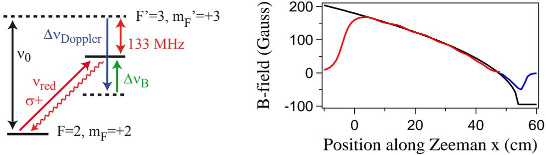
**Figure 3.5: Zeeman slower principle.** *left*)  $^{87}\text{Rb}$  levels considered in the Zeeman slower. *right*) Theoretical magnetic field (black line) versus the position inside the Zeeman tube. Two arrays of solenoids are adjusted to create a magnetic field (red and blue line) that matches the theoretically calculated field.
