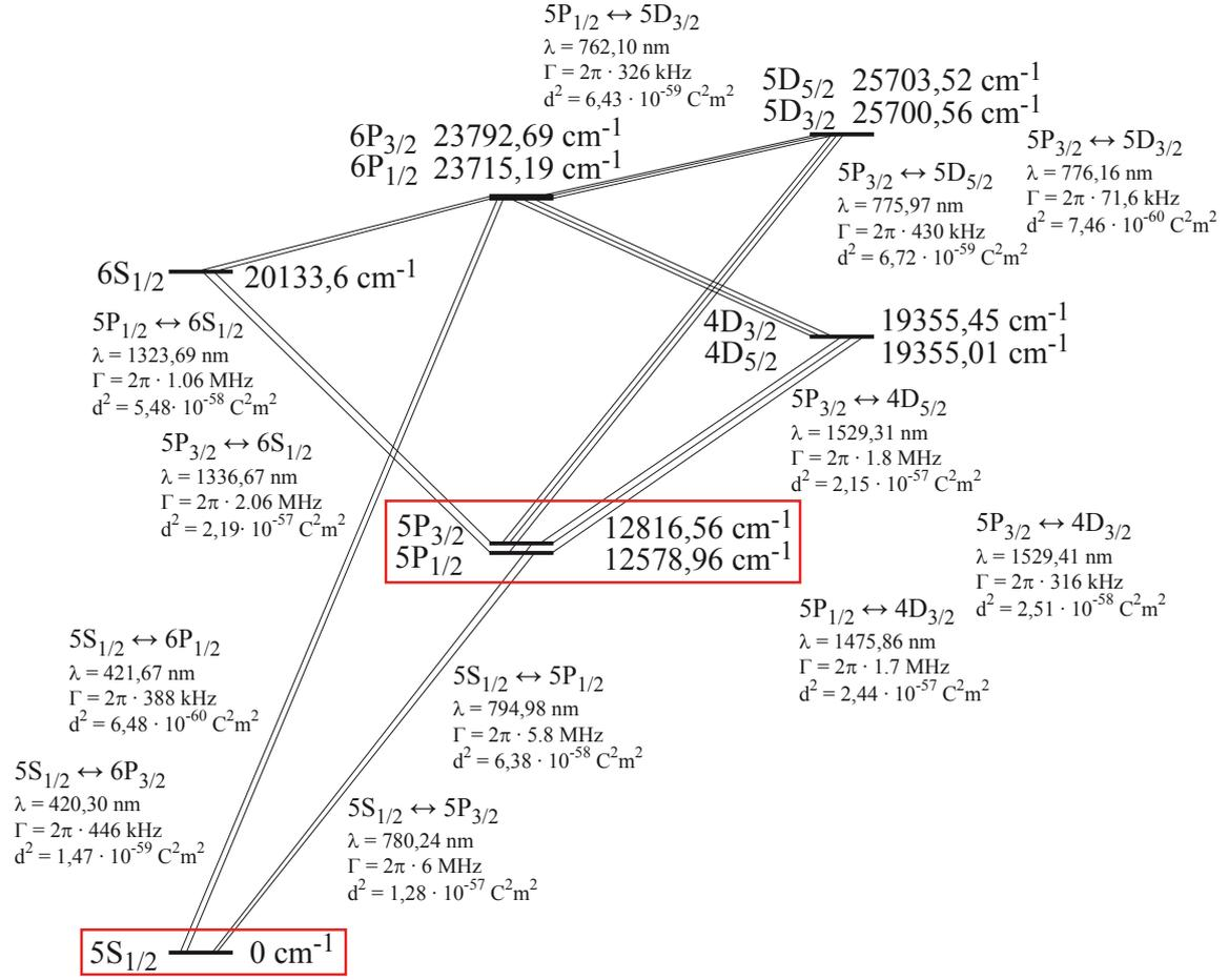
**Figure 1.1: Rubidium level structure.** The fine-structure of rubidium is shown for the first excited levels. The dipole moment  $d$  of each level can be calculated by using the Wigner-Weisskopf formula  $d_{J,J'}^2 = |\langle J || e\mathbf{r} || J' \rangle|^2 = \frac{2J'+1}{2J+1} \frac{3}{8\pi^2} \epsilon_0 \hbar \lambda_{JJ'}^3 \Gamma_{JJ'}$ . The red-framed states are used for our optical transitions.
