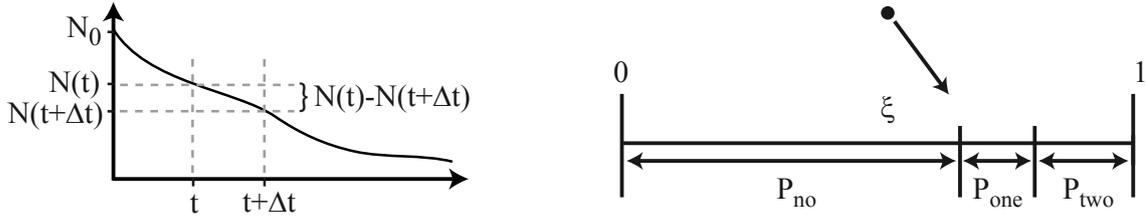
**Figure 9.7: Simulation procedure.** *left*) Atom number  $N(t)$  versus time. During the time step  $\Delta t$  the atom number decreases from  $N(t)$  to  $N(t + \Delta t)$ . *right*) The decision of how to proceed with the atom depends on which case the random number  $\xi$  falls in. One- and two-body as well as no loss are possible outcomes, each having probabilities  $P_{\text{one}}$ ,  $P_{\text{two}}$  and  $P_{\text{no}}$ .
