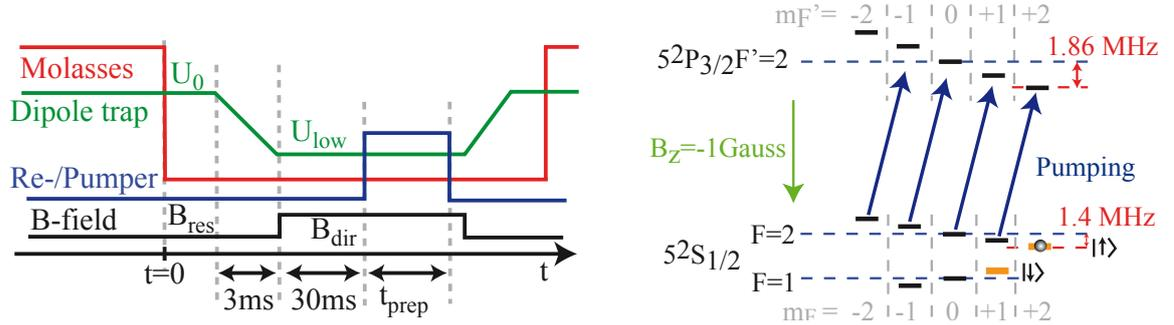
**Figure 7.2: Single atom optical pumping sequence.** *left*) Experimental sequence used to prepare a single atom in the state  $5^2S_{1/2}F=2, m_F=+2$ . *right*) Rb level scheme under a magnetic bias field  $B_z = -1$  Gauss. The pumper laser drives the atom into state  $|\uparrow\rangle$ . The linear trap polarization points in  $z$ -direction and is thus parallel to the magnetic bias field.
