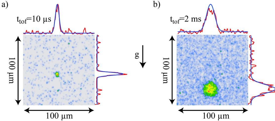
**Figure 11.6: Raw images of cold atom cloud.** We show raw images of an ultra-cold atom cloud containing 8 atoms on average. The cloud is imaged using the probe and repumper probe laser for  $10\mu\text{s}$  with  $s \sim 5$  after a time of flight of *a*)  $100\mu\text{s}$  and *b*)  $2\text{ms}$ . The cross-sections (red lines) are fitted by using a Gaussian model (blue lines). For long time of flights gravity leads to a shift of the atom cloud center.
