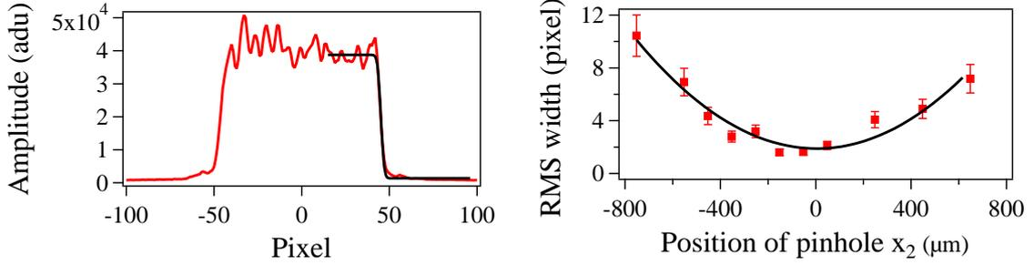
**Figure 4.12: Intensifier resolution.** *left*) Cross section of the edge as it appears on the CCD camera with the erf-function used as a fit in red. The rms width of the erf-function, corresponds to the effective PSF. *right*) Dependence of the rms width versus the distance  $x_2$  of the sharp edge with respect to object plane. At the minimum the edge is conjugated with the intensifier and has a rms width of  $1.9 \pm 0.3$  pixel.
