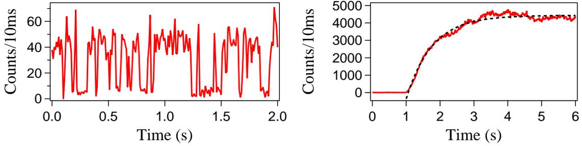
**Figure 3.10: Atom and MOT fluorescence on the APD.** *left*) The molasses-induced single atom fluorescence shows characteristic intensity jumps between  $\sim 5$  and  $\sim 45$  photon counts/10 ms over time. Each data point is averaged over 10 ms. *right*) Starting the MOT loading at  $t=1$  s the fluorescence shows an exponential increase over time. The loading time is 1.3 s after which the fluorescence level can reach values 100 times higher than for the single atom.
