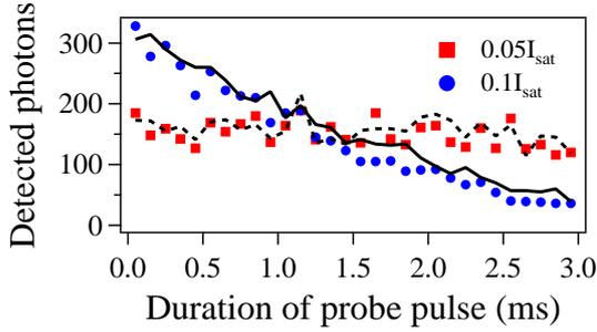
**Figure 7.9: Probe-induced depump probability.** Fluorescence of a single atom averaged over 500 sequences with two different probe pulse powers of  $0.05 I_{sat}$  and  $0.1 I_{sat}$ . The black curves correspond to the fluorescence when the repumper probe laser is additionally switched on. The recapture rate over 500 sequences is 99 % and 70 %, respectively.
