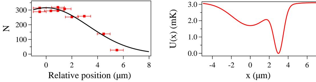
**Figure 10.2: Position dependent macro-micro trap atom transfer.** *left*) Number of atoms in the micro trap (2.7 mK) versus the relative position between both traps. A Gaussian fit (black curve) yields a rms width of  $3.3 \pm 0.3 \mu\text{m}$ . *right*) Trap profile for a combination of the 1.4 mK deep macro and 2.7 mK deep micro trap displaced by  $3 \mu\text{m}$  from each other.
