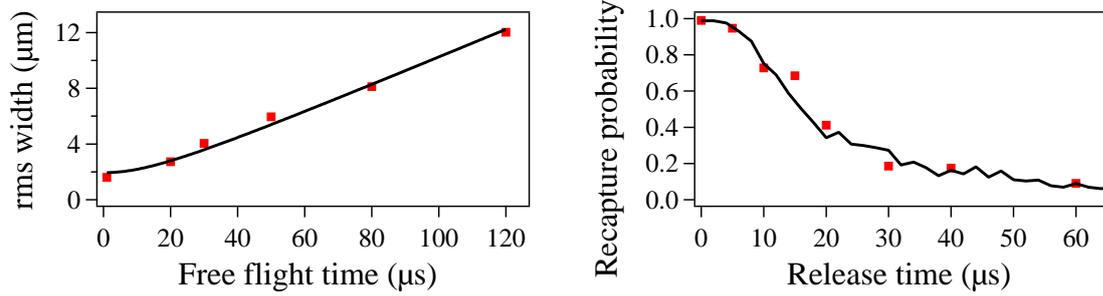
**Figure 10.4: Time-of-flight vs release and recapture method for dense clouds.** *left)* We show the evolution of the atom cloud rms width with the time in free flight. A fit of Eq. 6.1 yields  $87.5 \pm 5 \mu\text{K}$ . *right)* We plot the atom recapture probability versus the release time. A Monte-Carlo simulation to fit the data yields a temperature  $80 \pm 10 \mu\text{K}$ .
