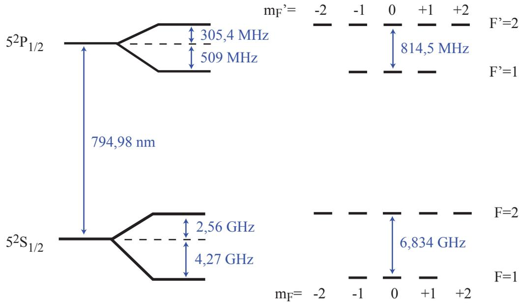
**Figure A.1: Rubidium  $D_2$  transition ( $5^2S_{1/2} \rightarrow 5^2P_{1/2}$ ).** Hyperfine structure of the rubidium ground state  $5^2S_{1/2}$  and the excited state  $5^2P_{1/2}$  with its magnetic components  $m_F$ .
