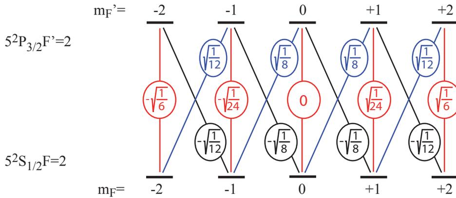
**Figure A.4:** Clebsch-Gordan coefficients  $C_{F,m_F,F',m_{F'}}^{J,J',I}$  for the transition  $5^2S_{1/2} F=2 \rightarrow 5^2P_{3/2} F'=2$ . Coefficients  $C_{2,m_F,2,m_{F'}}^{1/2,3/2,3/2}$  for the  $\sigma^+$  transition  $m_{F'} = m_F + 1$  (blue),  $\pi$  transition  $m_{F'} = m_F$  (red) and  $\sigma^-$  transition  $m_{F'} = m_F - 1$  (black).
