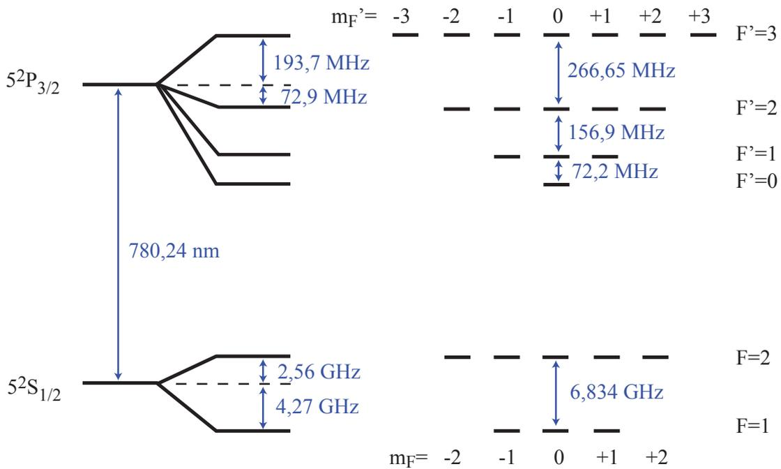
**Figure A.2: Rubidium  $D_2$  transition ( $5^2S_{1/2} \rightarrow 5^2P_{3/2}$ ).** Hyperfine structure of the rubidium ground state  $5^2S_{1/2}$  and the excited state  $5^2P_{3/2}$  with its magnetic components  $m_F$ .
