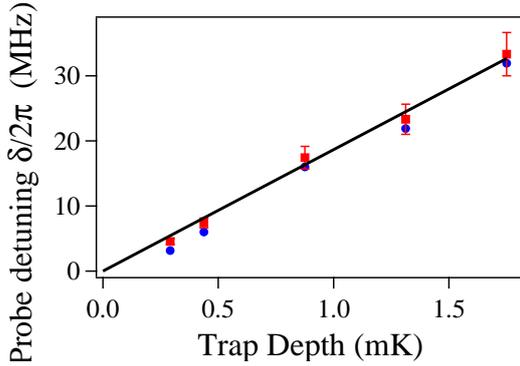
**Figure 7.14: Probe laser frequency.** We plot the probe laser detuning  $\delta$  versus the trap depth. For each trap depth the probe laser frequency needs to be adjusted to stay on resonance with the light-shifted atom. The linear fit through the origin has a slope of  $18.6 \pm 0.4$  MHz/mK and indicates that the probe laser is slightly red-detuned with the light-shifted atom, see text.
