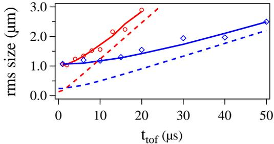
**Figure 6.5: Time-of-flight measurement of a single atom.** We show the time-of-flight measurements with corresponding simulation for two different temperatures:  $T = 20 \pm 2 \mu\text{K}$  (blue diamonds) and  $T = 150 \pm 16 \mu\text{K}$  (red circles). The dashed lines (respectively blue and red) show the results of Eq. 6.1 for the same temperatures and  $\sigma_0 = \sigma_{\perp}(0)$ .
