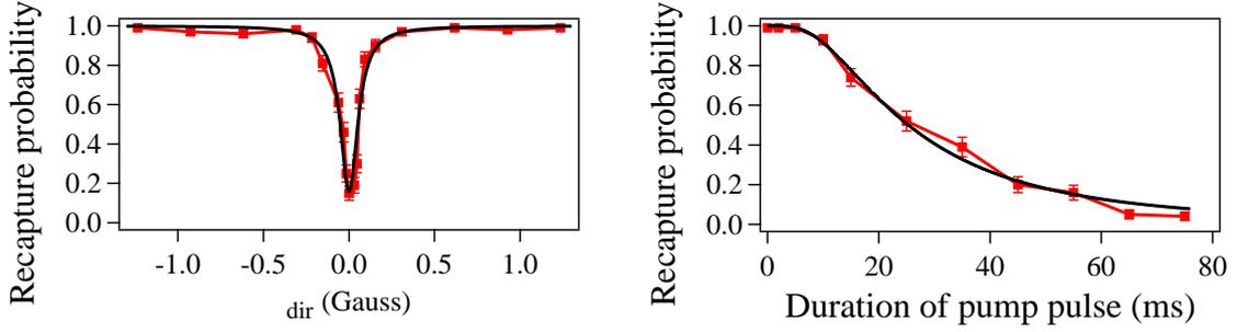
**Figure 7.5: Single atom state preparation.** *left*) Single atom recapture rate versus the magnetic field imposed by the  $z$ -compensation (blue circles) coils for a duration of the pumper pulse of 2 ms. The black line is a lorentzian fit. *right*) Dependence of the recapture rate versus the duration of the pumper pulse for a bias magnetic field  $B_{dir} = -1$  Gauss. The black line is a fit of Eq. 5.5.
