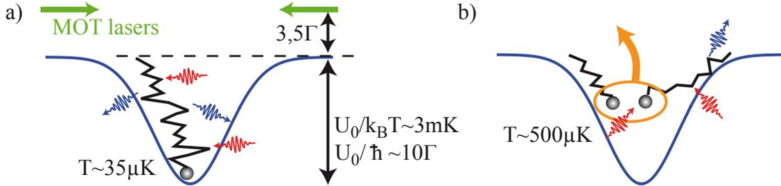
**Figure 9.2: Atom cooling inside the dipole trap.** a) A single atom can be laser-cooled to the bottom of the trap  $U_0$ . Temperatures as low as 35  $\mu\text{K}$  have been measured for  $U_0/k_B = 2.7$  mK. b) Cooling of many atoms is hampered by light-assisted collisions. Before being cooled to the bottom of the trap both atoms are ejected from the trap.
