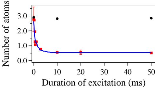
**Figure 9.3: MOT-induced two-body loss.** Atom number versus excitation light duration for which the MOT lasers have been used. The collisional loss rate  $\beta' = 0.5 \text{ ms}^{-1}$  is extracted from a simulation. The black circles indicate the one-body losses.
