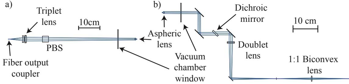
**Figure 3.8: Micro trap beam path and imaging system.** a) Beam path of the micro trap laser between the optical fiber and the aspheric lens. The calculated axial magnification is  $g_x = 1/g_y^2 = 1/4.2^2$ . b) Imaging system used to collect atom fluorescence by the aspheric lens and detect it on a CCD and APD. The calculated radial magnification is  $g_y = 26 \pm 2$ .
