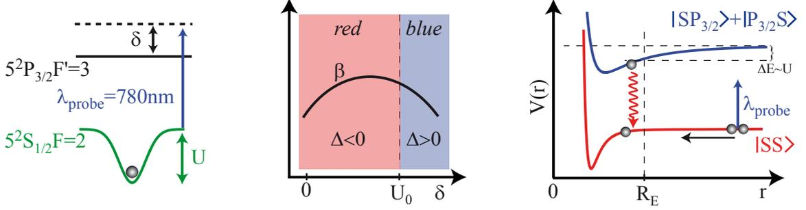
**Figure 9.10: Definition of the probe laser detuning.** We define the probe detuning  $\delta$  with respect to the atomic transition  $F=2 \rightarrow F'=3$  in free space. We define blue-detuned probe light by  $\delta > U/\hbar$  ( $\Delta = \delta - U/\hbar > 0$ ) and red-detuned probe light by  $\delta < U/\hbar$  ( $\Delta = \delta - U/\hbar < 0$ ).
