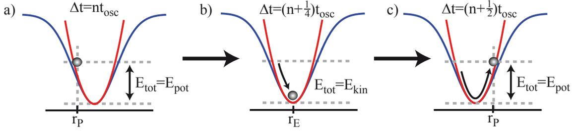
**Figure 5.4: Idea of measuring the trap frequencies.** a) The atom's total energy is in form of potential energy. b) After one fourth oscillation it converts the potential energy into kinetic one. c) The atom reaches another point where its total energy corresponds to the potential energy.
