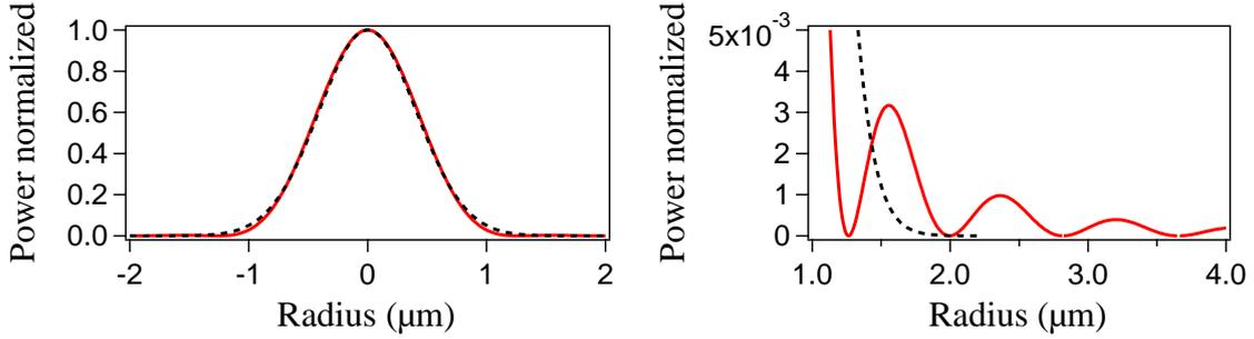
**Figure 3.9: Micro trap profile.** *left*) The normalized intensity created by the dipole trap in the focal plane of the aspheric lens. *right*) A zoom onto the wings of the profile shows the presence of Airy rings. These are very small and have a height of only  $\sim 3 \cdot 10^{-3}$ .
