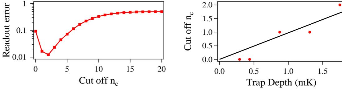
**Figure 7.15: Cut off parameter  $n_c$ .** *left*) Dependence of the state detection fidelity on the cut off parameter  $n_c$  for the photons detected by atoms in a 1.4 mK trap depth and a probe pulse length of 1.5 ms. *right*) Cut off parameter  $n_{c,min}$  that minimizes the read-out error versus the dipole trap depth.
