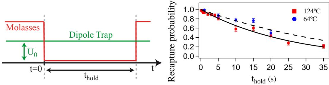
**Figure 5.8: Single atom trap lifetime.** *left*) At  $t=0$  we trigger on a single atom in a dipole trap with wavelength 850 nm and a trap depth  $U_0/k_B = 2.7$  mK. After the holding time  $t_{\text{hold}}$  we check if the atom is still trapped. *right*) Recapture probability versus holding time. We repeat the measurement for two different oven temperatures 64°C and 124°C and find lifetimes of  $\tau = 1/\gamma = 36$  s and  $\tau = 24$  s, respectively.
