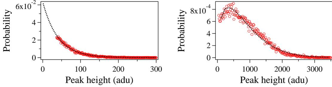
**Figure 4.7: Peak histogram for gain 6 and 9.** Amplitude distributions for a gain of *left*) 6 and *right*) 9 for isolated events (group 3). The data for gain 9 is binned by 15. The black line corresponds to the theoretical prediction. All events smaller than the threshold  $\varepsilon$  are not counted.
