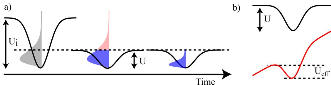
**Figure 11.1: Evaporative cooling.** *a)* The atoms occupy the trap energy levels according to a Boltzmann distribution for temperatures  $T_i \gg 0$ . Lowering the trap depth from  $U_i$  to  $U$  all atoms belonging to the grey shaded part of the distribution are lost and colder atoms remain trapped. After thermalization, the temperature of the gas is lowered to  $T = T_i \cdot U/U_i$ . *b)* A possibility to lower the effective trap depth without changing the oscillation frequency.
