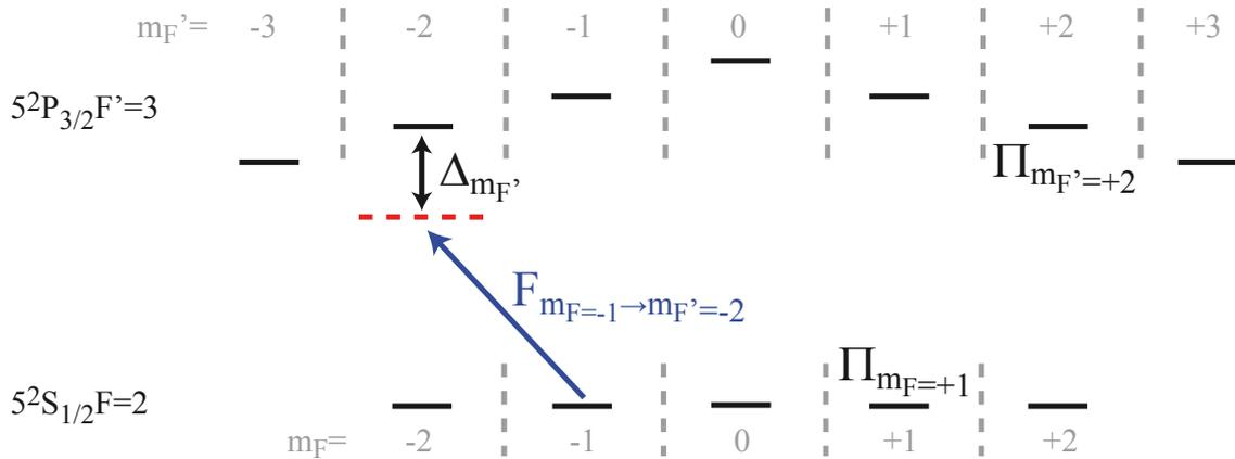
**Figure C.1:** Off-resonant probe laser driving the transition  $5^2S_{1/2}F=2 \rightarrow 5^2P_{3/2}F'=3$ . The probe laser (blue arrow) drives any transition between  $5^2S_{1/2}F=2 \rightarrow 5^2P_{3/2}F'=3$  with coupling  $F_{m_F \rightarrow m_{F'}}$  and alters the population in each level  $\Pi_{m_F}$ . Its frequency detuning with respect to a certain Zeeman level  $5^2P_{3/2}F'=3m_{F'}$  is denoted as  $\Delta_{m_{F'}}$ .
