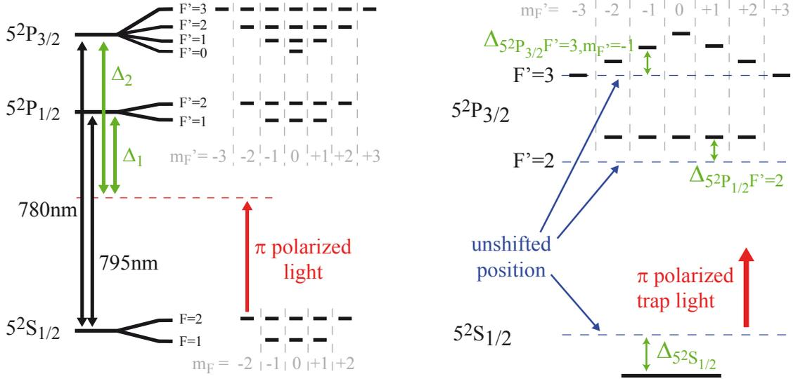
**Figure 1.7: Light shifts for far-off resonance detuned  $\pi$ -polarized light.** *left*) Far-off resonance detuned laser light can couple different Zeeman sub-levels with each other. The laser detuning is denoted as  $\Delta_1$  and  $\Delta_2$  for the  $D_1$  and  $D_2$  transition, respectively. *right*) We illustrate the light-shift on each Zeeman sub-level of the  $5^2P_{3/2} F'=2$  and  $F'=3$  hyperfine levels. All Zeeman sub-levels of  $5^2S_{1/2}$  are shifted by the same quantity.
