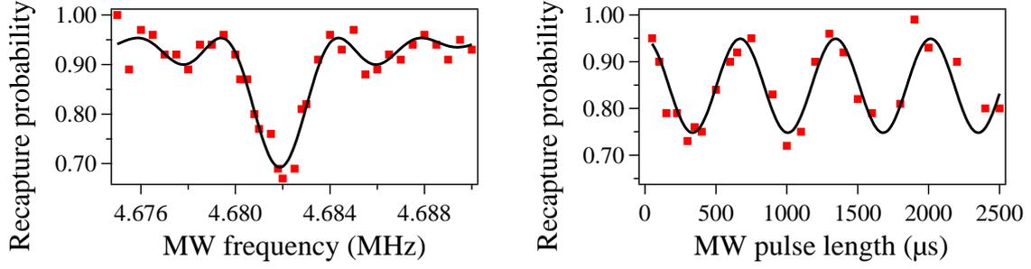
**Figure 5.10:** MW induced hyperfine transition  $F = 1, m_F = 0 \rightarrow F = 2, m_F = 0$ . *left*) Dependence of the single atom recapture rate on the MW frequency for a MW pulse duration of  $350 \mu\text{s}$ . The black line is a fit to the hyperfine transition spectral line. *right*) Dependence of the single atom recapture rate on the MW pulse duration for a MW frequency of  $\nu_0 = 6.834682 \text{ GHz}$ .
