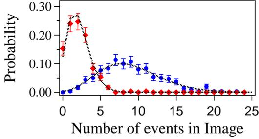
**Figure 8.5: Event histogram for  $\sim 6$  atoms on average.** Probability distribution of the number of detected events when the dipole trap is filled with 6.3 atoms on average (blue circles). It is well fitted by Eq. 8.2 for a probe duration of 20  $\mu\text{s}$  corresponding to an average number of detected photons scattered per atom  $\bar{n}_{\text{at}} = 1.1$ . The background distribution (red diamonds) is of Poisson type ( $\bar{n}_{\text{bg}} = 2.1$ ).
