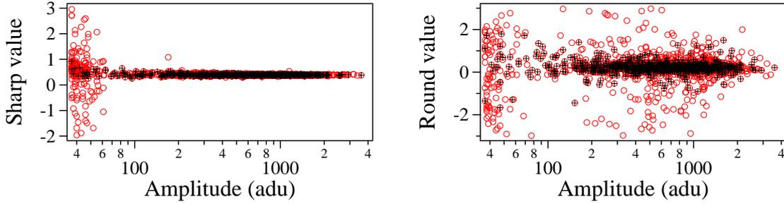
**Figure 4.6:** “Sharp” and “round” values for gain 9. *left*) We plot the dependence of the “sharp” parameter on the peak amplitude, where we use an area of  $3 \times 3$  ( $u = 1$ ) pixels around the peak center for the calculation. Isolated events are highlighted as red crosses. *right*) We show the same for the “round” parameter using a  $7 \times 7$  ( $u = 3$ ) pixels around the peak center.
