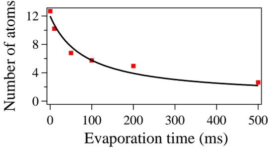
**Figure 9.11: Hyperfine changing collisions.** We show the atom number versus the holding time at a fixed trap depth of 1.8 mK. The atoms have an initial temperature of 400  $\mu$ K. The 10 % population in  $F = 2$  as well as the trap-induced Raman transitions lead to a constant loss due to hyperfine changing collisions. A fit of Eq. 9.4 yields a loss constant  $\beta'_{\text{dark}} = 1\text{s}^{-1}$ .
