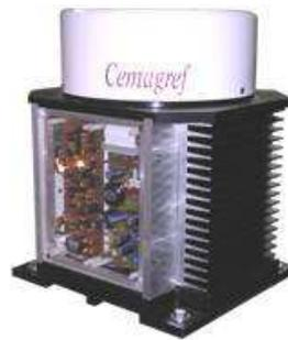
FIGURE 2.12 – Radar FMCW K2Pi.
