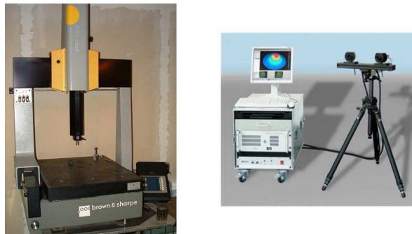
Figure 4.1: Coordinate-measuring machine (left) and Aramis' 3D optical system (right) [Image sources: starequipment.net; uakroncivil.com]
