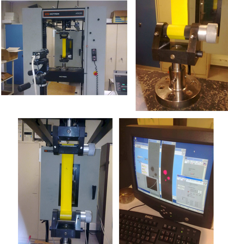
Figure 5.4: 3-spot local measuring system setup
