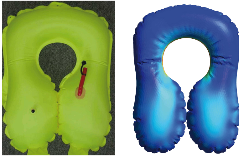
Figure 7.4: Comparison between a real inflated lifejacket (left) and the field of displacement resulting of the simulation (right)
