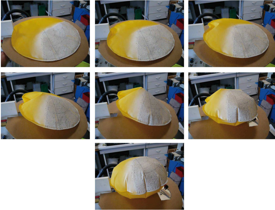
Figure 4.13: Captures of the air bag inflation sequence, where the apparition of a big wrinkle can be observed
