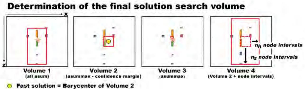
FIGURE 5.3: MAXI 2.0 scheme representing volumes 1, 2, 3 and the final search volume 4 (called V1, V2, V3 and V4 respectively). V1 includes all SPRED nodes. V3 includes SPRED nodes intersected by the maximum number of EDTs after stacking (value named *asummax*). V2 includes SPRED nodes with a value of EDT intersections ranging between *asummax* and (*asummax* - confidence margin). V4 is the search area.
