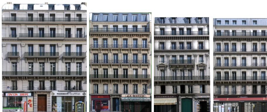
Figure 5.11: Perspective rectification is obtained using an orthographic rendering of a 3D facade with projective texture mapping. From left to right the real-world dimensions are: 17.6x24.4m, 13.5x22.2m, 12.6x20.9m and 15.1x20.6m and the pixel image resolutions are: 333x465, 487x799, 392x642 and 372x519.
