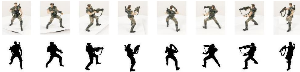
Figure 4.1: A sample data set: Our system takes as input a set of calibrated images and silhouettes and produces a textured polygonal model. [VGG 2008b]
