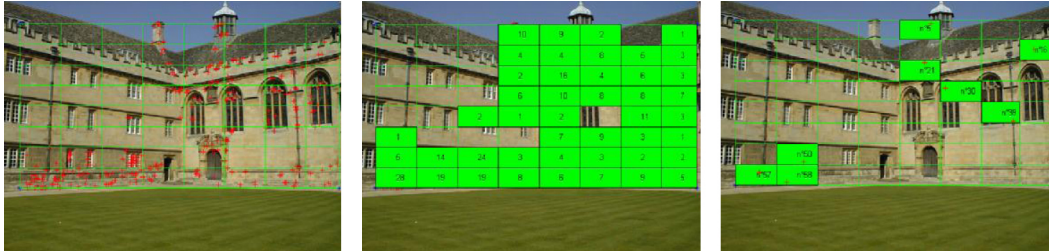
Figure 2.6: Principle of the bucketing technique for selecting candidate points : (left) cut the region into 8 \times 8 buckets, (middle) buckets with no points are removed, (right) select s = 8 buckets.
