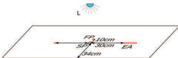
Fig. 3 Exp. B set up: Subjects sat in front of the device. They performed free movements with the right arm above the pointing surface. The starting point was an invisible tactile landmark. Targets were red LEDs under a homogeneous translucent screen. An ambient light could be turned-on/off to allow/prevent vision of the hand. Free index fingertip trajectory was recorded with an Optotrak system. DC horizontal eye movements were recorded with EOG electrodes. All devices were driven by a real-time OS. EA incremental exposure area, FP fixation point, L light, SP tactile starting point
