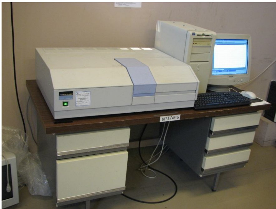
Figure 31: Photo of PerkinElmer Lambda 19 spectrometer
