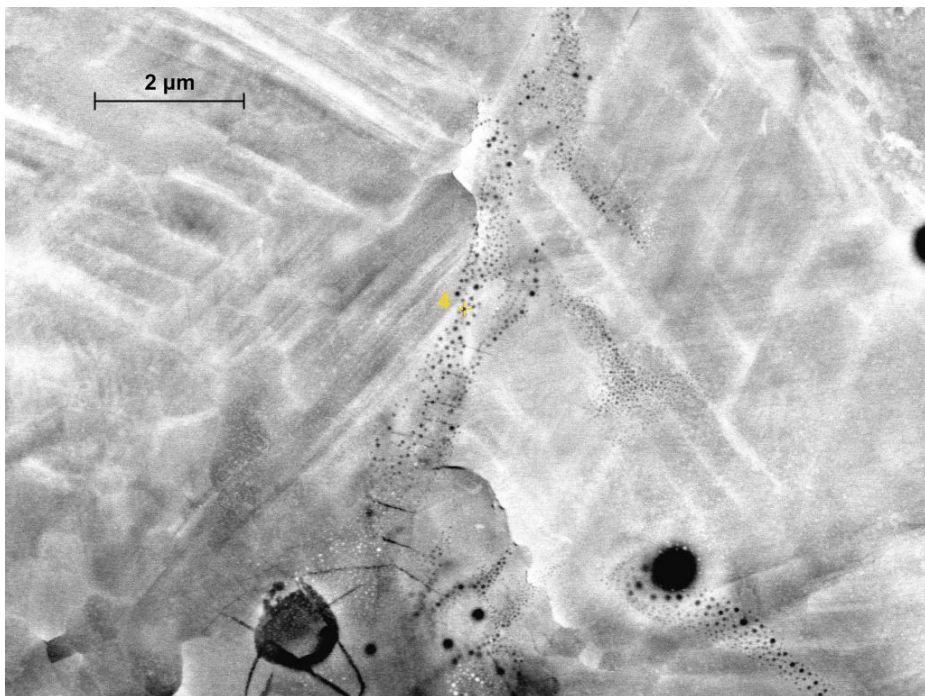
Figure 74: Stainless steel mirror. Close view of the inner part of the crater. Measured with SEM. Magnification: 10000x.
