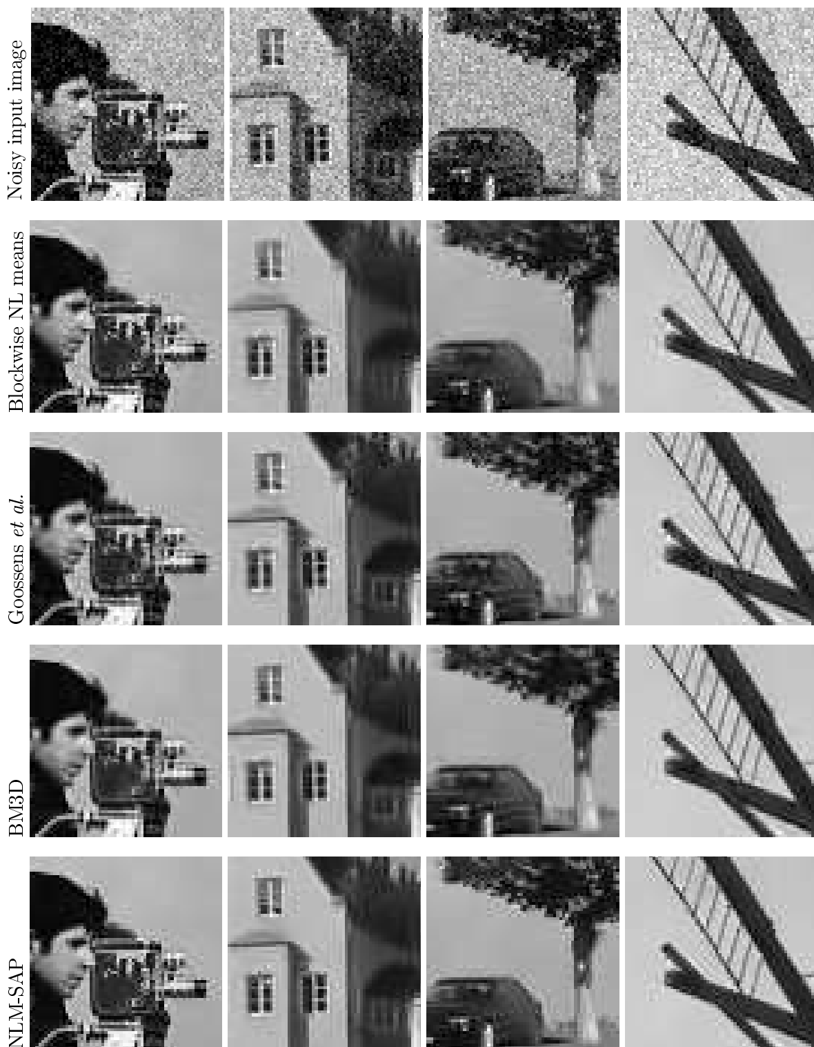
Figure 7.12: Comparisons of the visual denoising performance of the proposed NLM-SAP approach and other state-of-the-art methodologies ( \sigma = 20 ). From top to bottom, the input noisy images, the results obtained by the classical (pixelwise) NL means (Buades et al. , 2005), the blockwise NL means for square patches the BM3D denoiser (Dabov et al. , 2007), and our proposed NLM-SAP approach.
