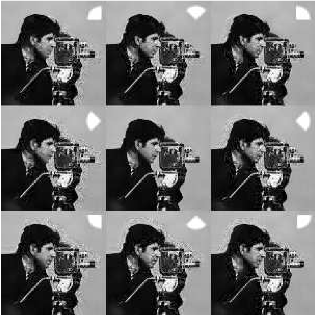
Figure 7.8: Eight denoised images obtained for different oriented patch shapes. The proposed final aggregate is in the center. Each denoiser provides good performance in a specific target direction but suffers from noise halos in the other directions. The final (central) aggregate takes advantage of every oriented-denoiser to provide high quality restored edges. The patch shape used is indicated in white.
