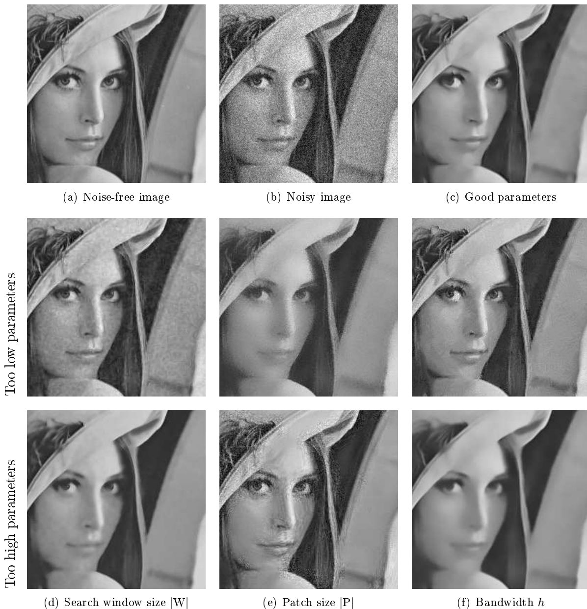
Figure 2.9: Influence of the three main parameters of the NL means on the solution.
