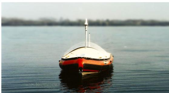
FIGURE 2.9 – *New Hydrographic Automated Vehicle* (Bordeaux, France)
