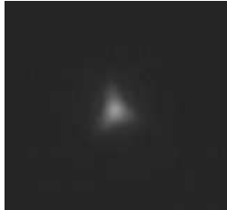
Fig. 2: Near field of the chalcogenide fiber.
