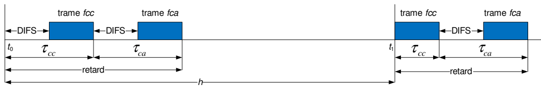
FIGURE 5.2 – DCF-WiFi : transfert de trames des flux f_{cc} et f_{ca} .
