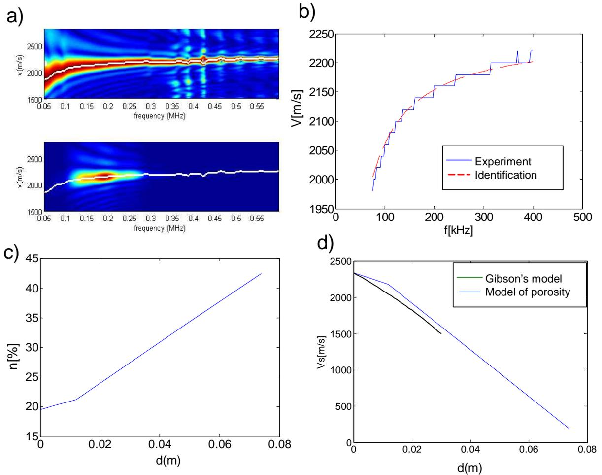
Figure V.11 The data and results of parameter identification of cement mortar sample with the use of the Gibson's model, a) one of the  $V$ - $f$  experimental map (shown in different sensitivity scale), b) the dispersion characteristics obtained by the measurements and identification, c) the distribution of porosity as a function of depth, d) the profile of transverse wave velocity obtained by the identification and by the model of porosity.
