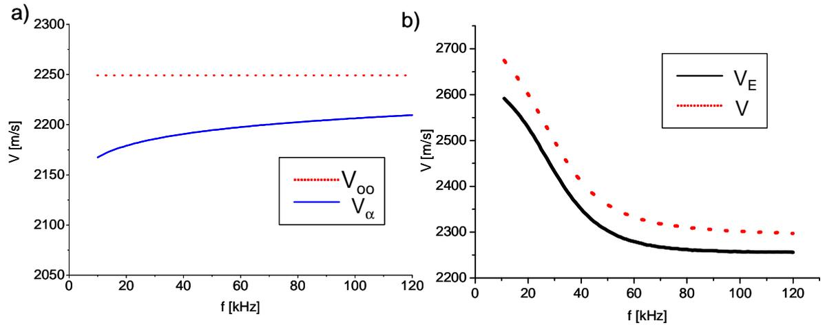
Figure II.13 Taking into account the dispersion caused by the attenuation: a) the  $V_\infty$  and  $V_\alpha$  curves, b) the dispersion characteristics with and without attenuation influence ( $V_E$  and  $V$  curves respectively).
