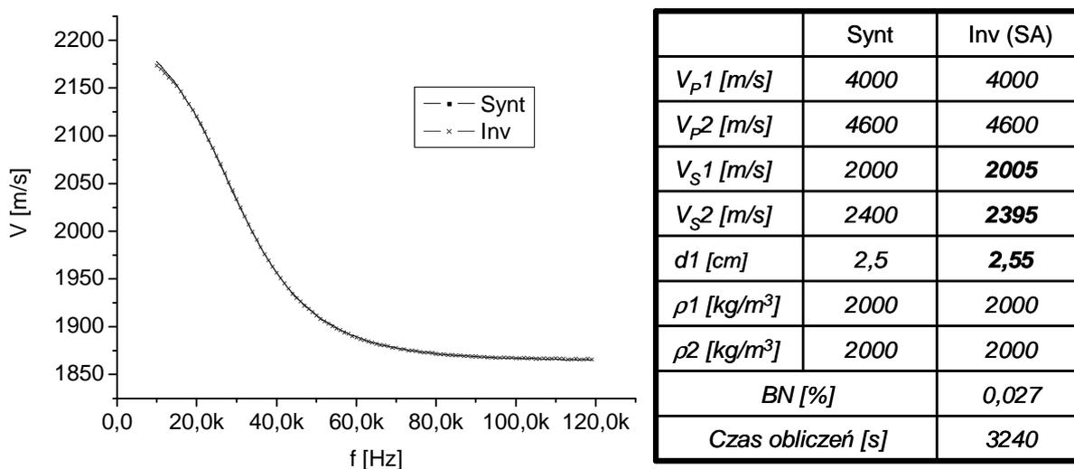
Figure A2.2 The example of identification procedure with SA method for the model in a configuration: 2 layers 3 parameters (2w3p).
