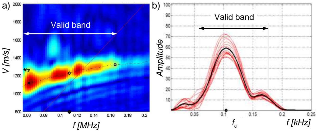
Figure III.11 The example of the dispersion map obtained from the SL and the Fourier transforms (a) and the example of spectral characteristics of received signals (b).
