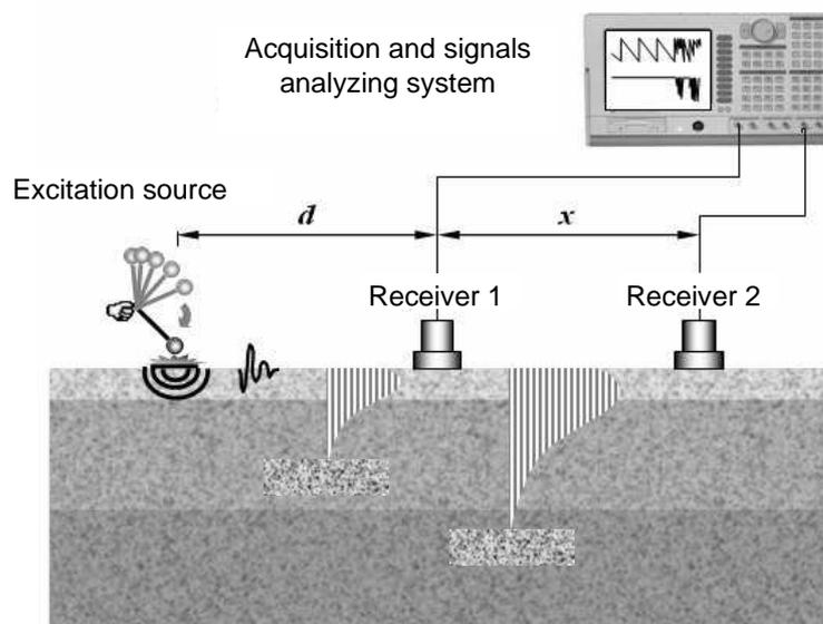
Figure III.1 Method of generation and measurement of surface waves [Wardany 2005].
