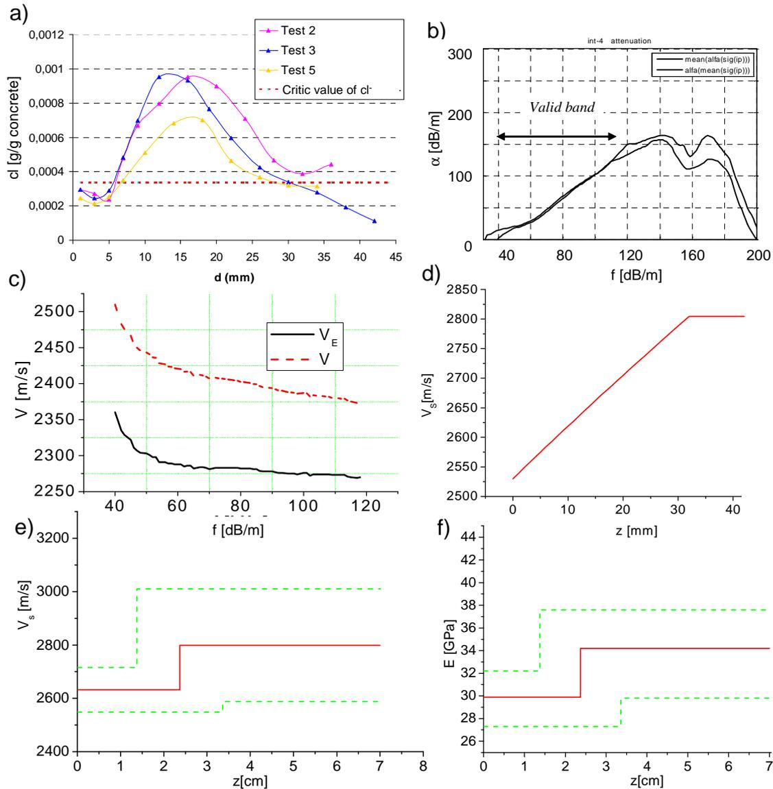
Figure V.12 The results of research for the concrete of port ramp in St. Nazaire; a) the distribution of the chloride ions content, b) the attenuation characteristics, c) the dispersion characteristics with and without an attenuation effect, d) the velocity profile  $V_s$  determined by the DDS program, e) the velocity profile  $V_s$  determined by the Cloud Point program (green dotted lines indicate the limits of standard deviation, red solid line indicates the average parameter value)..
