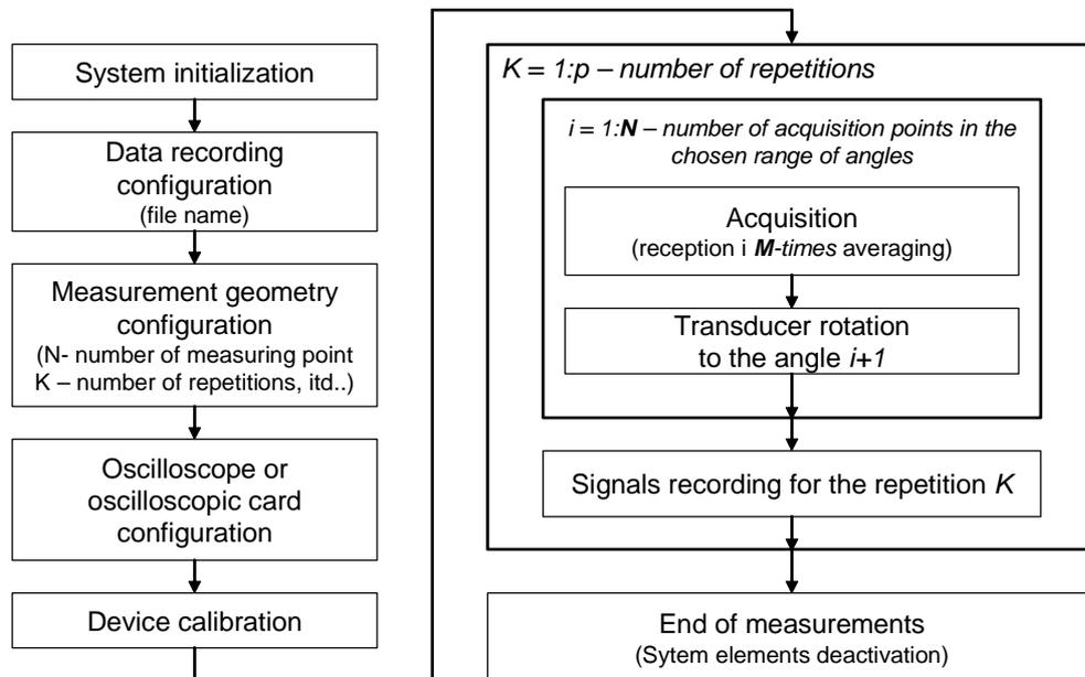
Figure III.20 The block diagram of the REFLECTO operating.
