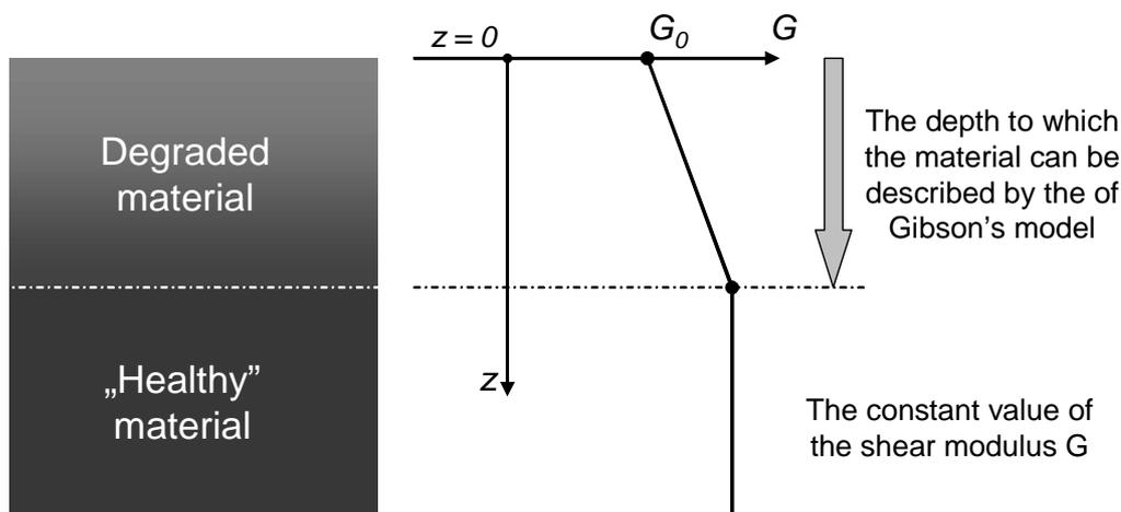
Figure IV.6 The illustration of a partially degraded material ( $G$  - shear module,  $z$  - depth).
