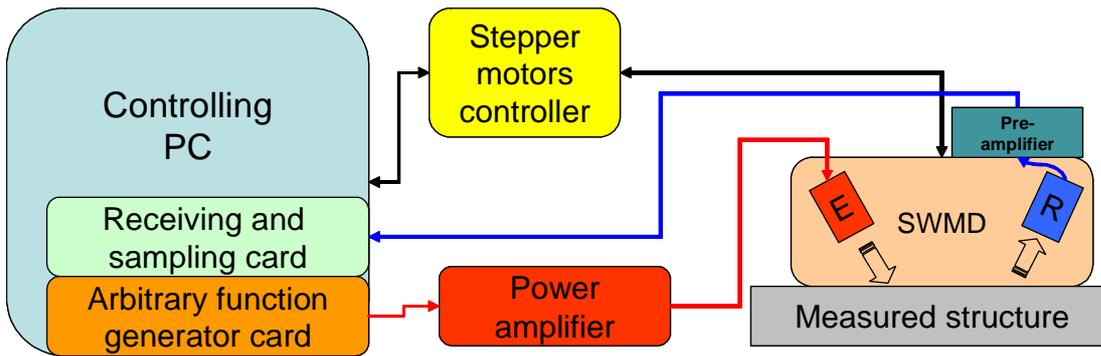
Figure III.4 The block diagram of SWMD system for surface waves measurement, SWMD – measuring device, E – emitter, R – receiver.
