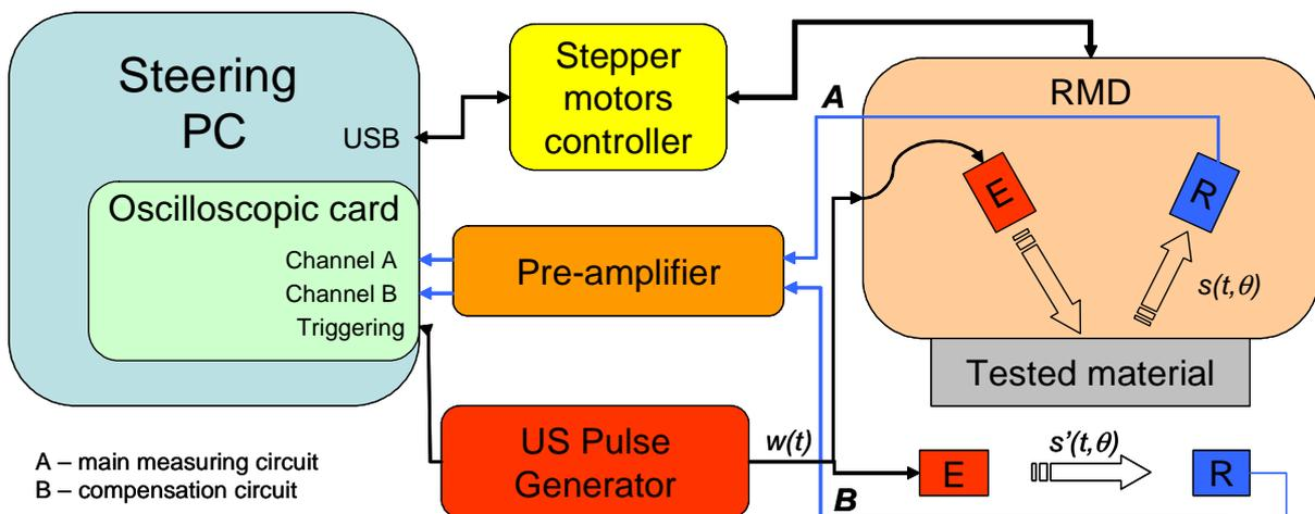
Figure III.18 The block diagram of the RMD system.
