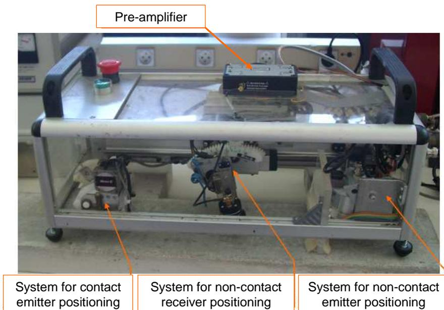
Figure III.6 SWMD during measurement of concrete sample.
