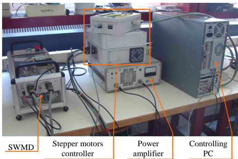
Figure III.5 The measuring system ready to work.
