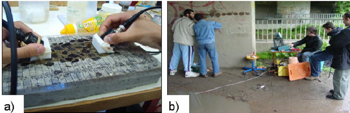
Figure III.2 Manual measurements of surface wave propagation; a) in the laboratory, b) in the field .
