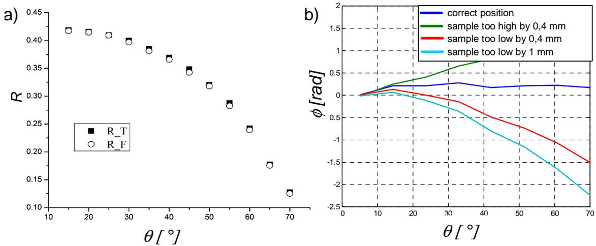
Figure III.21 a) The reflection coefficient characteristic  $R$  as a function of the angle  $\theta$ ,  $R_T$  – curve calculated from the amplitudes of signals in time domain,  $R_F$  – curve calculated on the basis of spectra, b) the phase characteristics of the signals  $e(t, \theta)$  for glass sample placed with an error of a vertical position.
