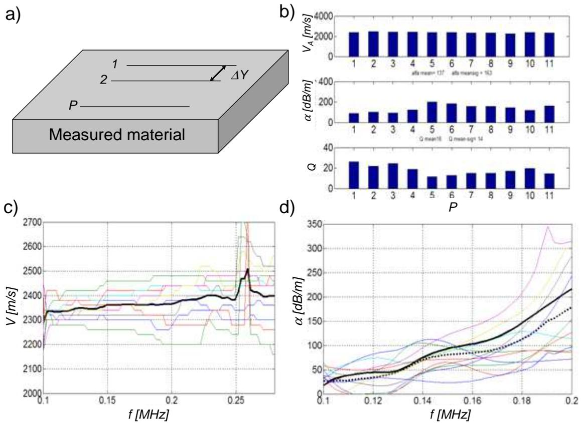
Figure III.12 The example of the measured profiles arranged on the measured surface (a), the results of measurements realized for 10 profiles (from top: velocity, attenuation, quality factor, 11<sup>th</sup> value in each row is a mean value) (b), the dispersion curves (bold line is a mean value) (c), the attenuation curves (bold line is a mean value) (d).
