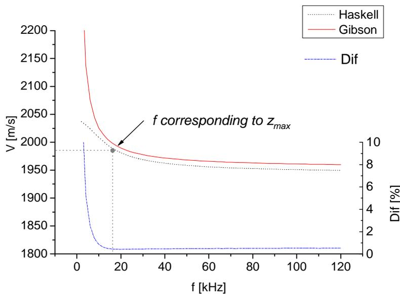
Figure II.12 The comparison of the dispersion characteristics obtained from Gibson's model (red continues line), and from Haskell's model (black dotted line). The differences  $Dif$  between characteristics (the blue dotted line).
