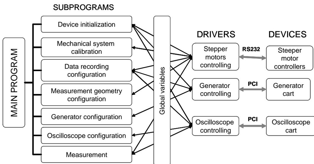
Figure III.7 The block diagram of controlling software..
