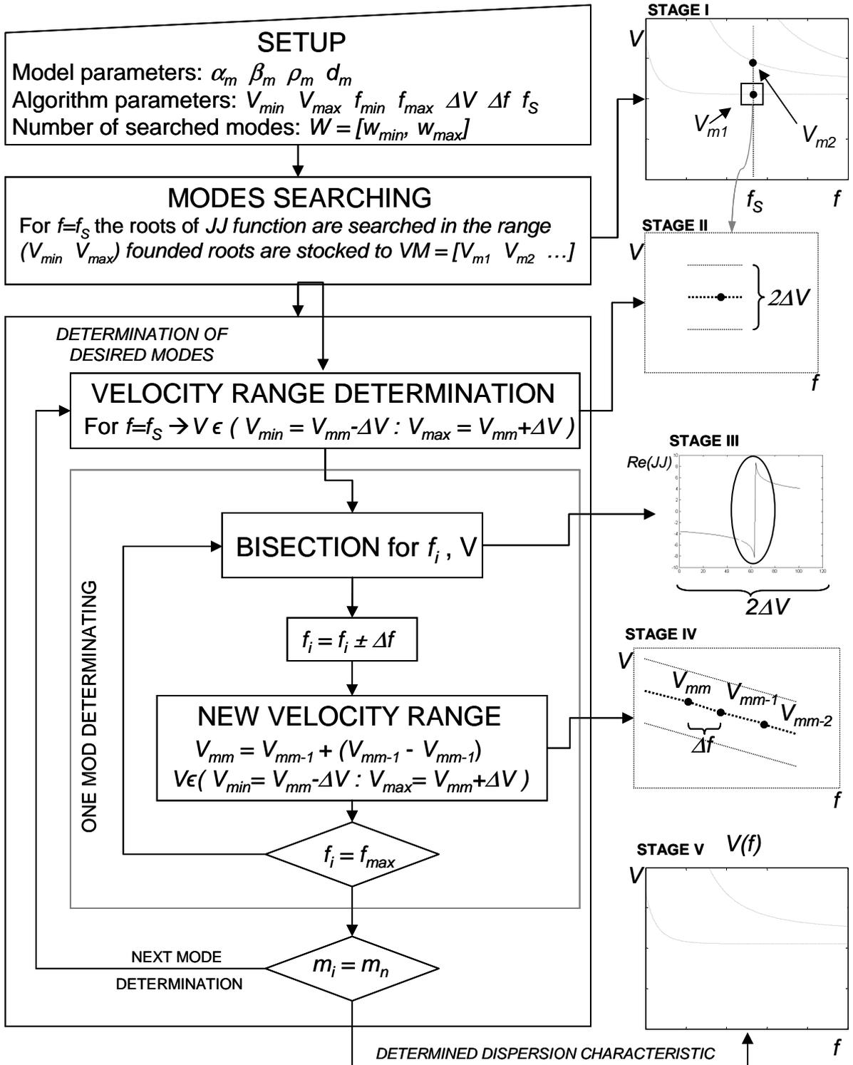
Figure II.5 The diagram of HASK program operating used for roots of dispersion equation determination based on Haskell model.
