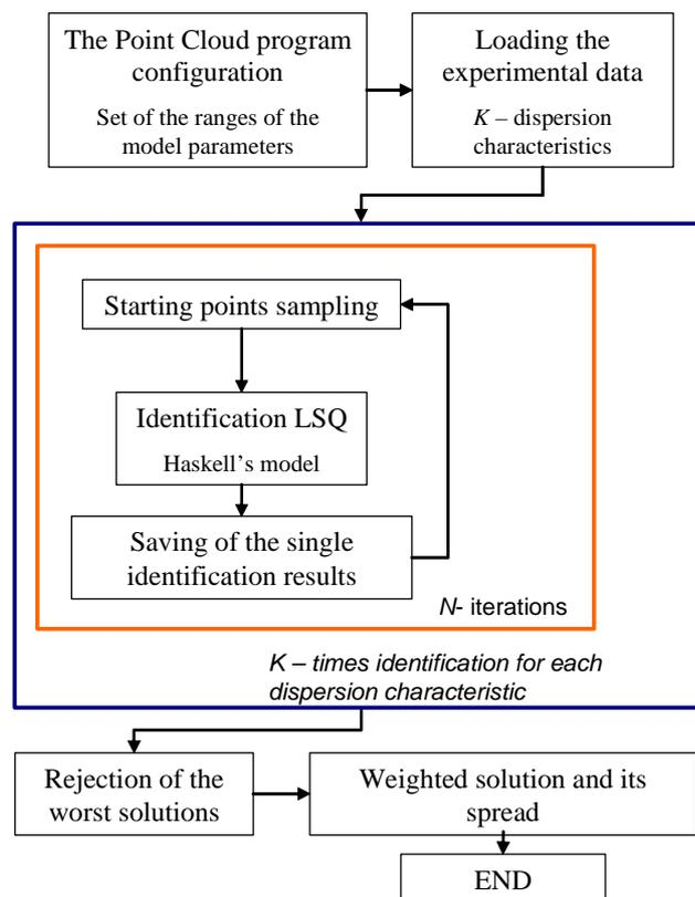
Figure IV.11 The flowchart of the Point Cloud procedure.
