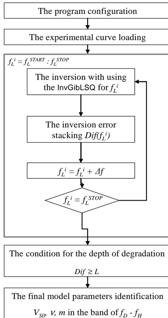
Figure IV.8 The block diagram of the DDS program.
