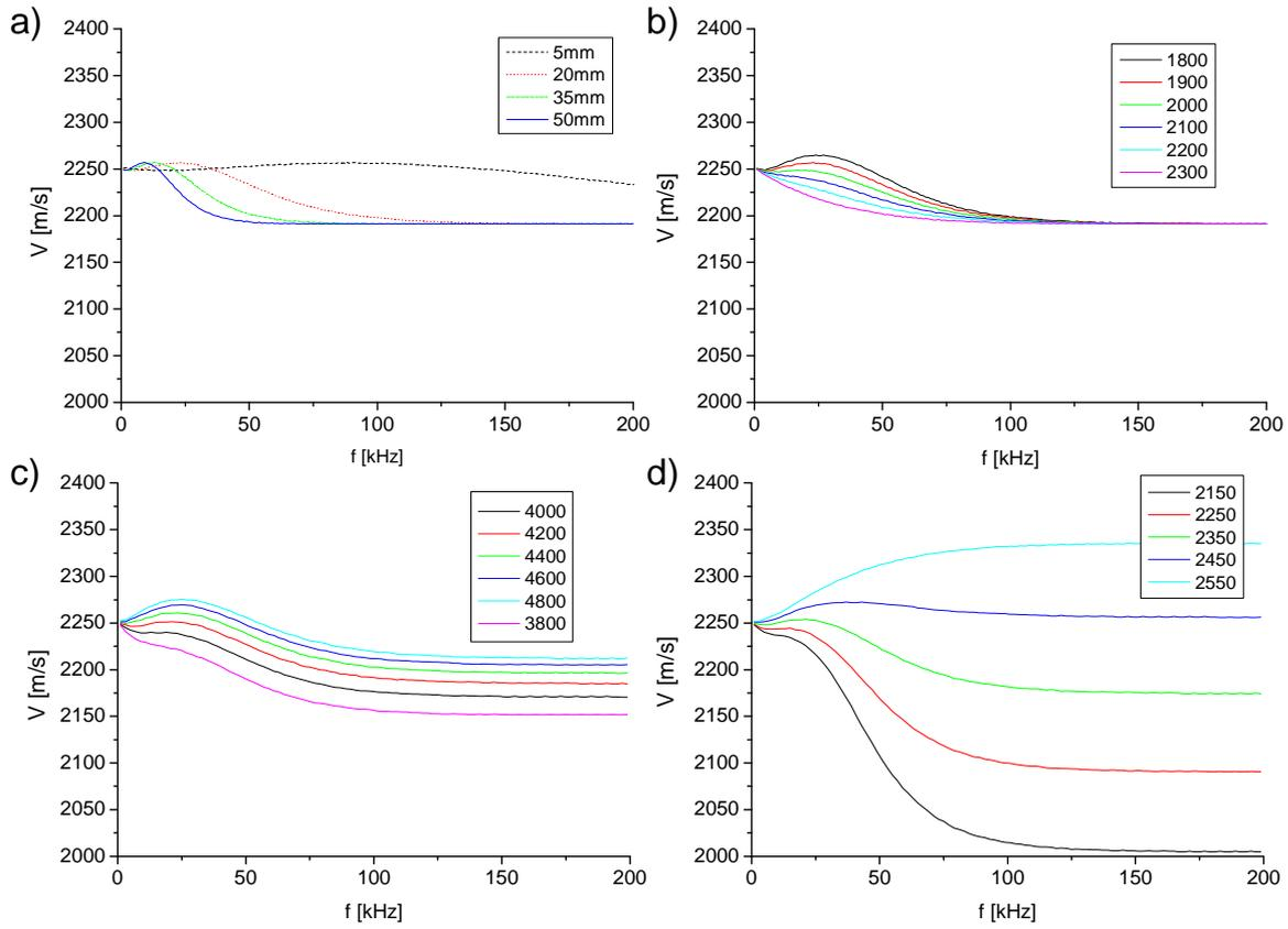
Figure II.7 Dispersion characteristic for two layers Haskell model for the case in which first layer parameters are changed a) the thickness  $d$ , b) the density  $\rho$ , c)  $V_P$  velocity, d)  $V_S$  velocity.
