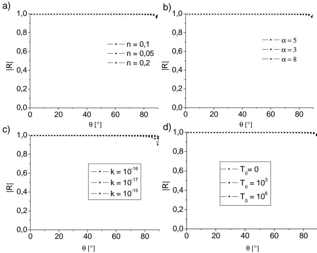
Figure II.16 The evaluation of  $R$  characteristic in the range of low porosity caused by the changes of a) porosity, b) tortuosity, c) permeability, d) surface flow impedance.
