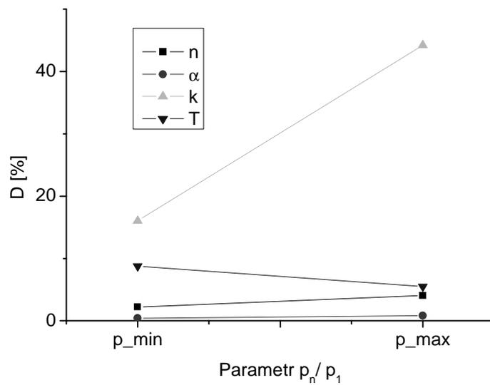
Figure II.18 The quantitative comparison of  $R$  characteristic evaluation caused by model parameters, where:  $n$  – porosity,  $\alpha$  – tortuosity,  $k_0$  – permeability and  $T$  – surface flow impedance.
