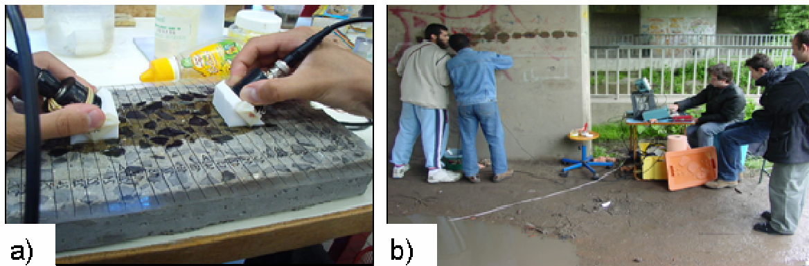
Figure III.2 Manual measurements of surface wave propagation; a) in the laboratory, b) in the field .
