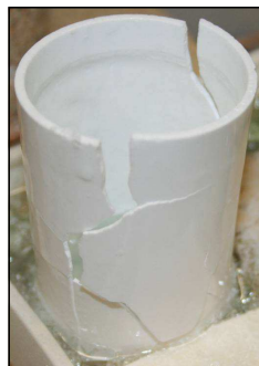
Figure 4.11: Opaque wall of crystallized silica crucible.
