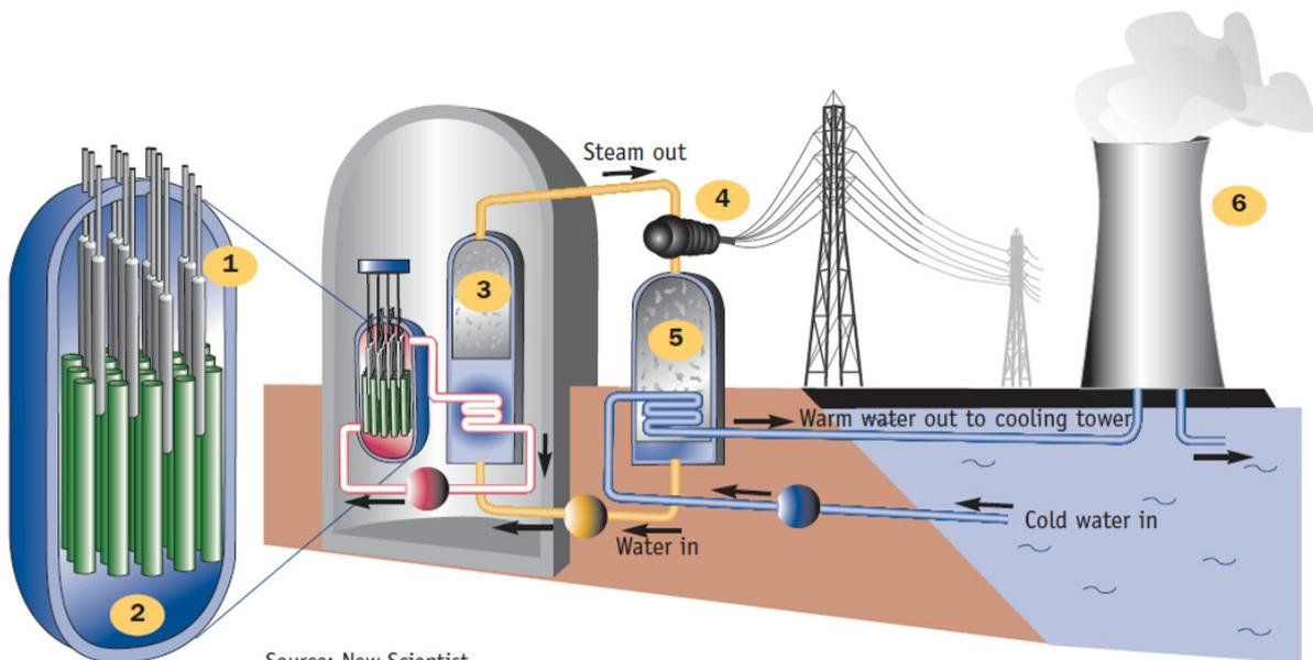
Figure 1.2. Basic components of a pressurized water reactor (from [12])
