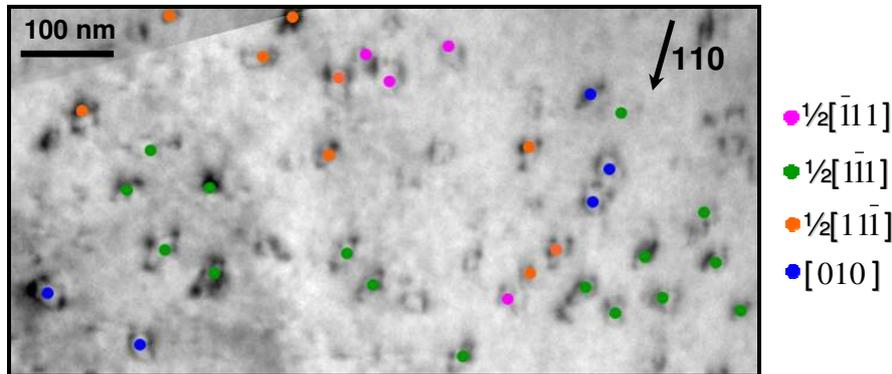
Figure 4.7. Dislocation loops in Fe-12%Cr model alloy irradiated with 150keV  $Fe^+$  ions to a dose of 1.5dpa at 500°C. The micrograph was taken under two beam conditions, zone axis  $(111)$ ,  $g = \bar{1}10$ . The dislocations are marked by circle the colour of which depends on the determined Burgers vectors. Some groups of neighbor dislocation loops have identical orientation and Burgers vectors. Details of analysis are given in the Chapter 5.
