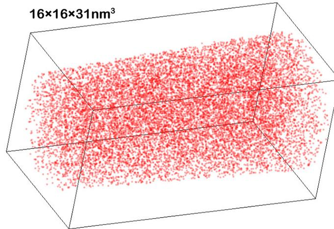
Figure 3.3 3D distribution of chromium atoms in the as-received Fe-5at% Cr model alloy. Each dot represents one atom. For clarity only chromium atoms are represented. Chromium atoms are homogeneously distributed.
