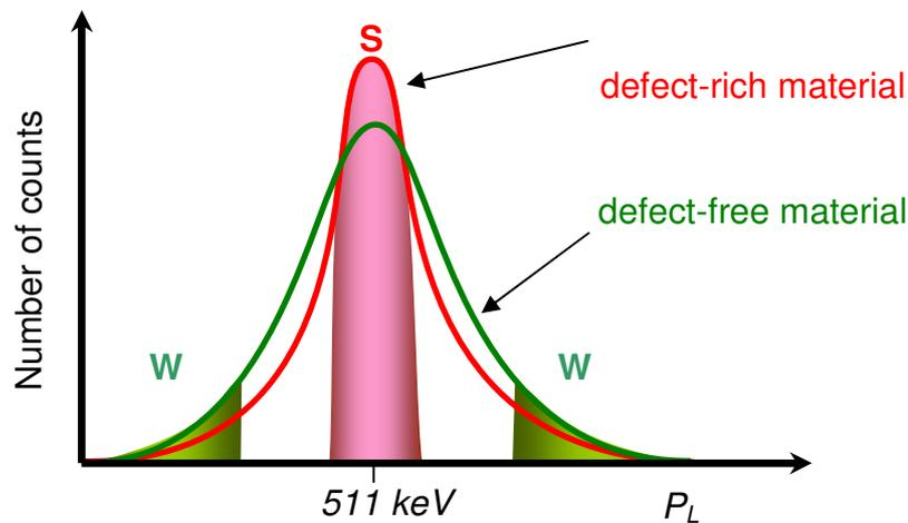
Figure 2.25. Doppler broadening spectra of defect free and defect rich materials. The definition of the S and W parameters in the Doppler-broadening spectra S-parameter corresponds to positron annihilation with the valence electrons and W-parameter corresponds to positron annihilation with the core electrons.
