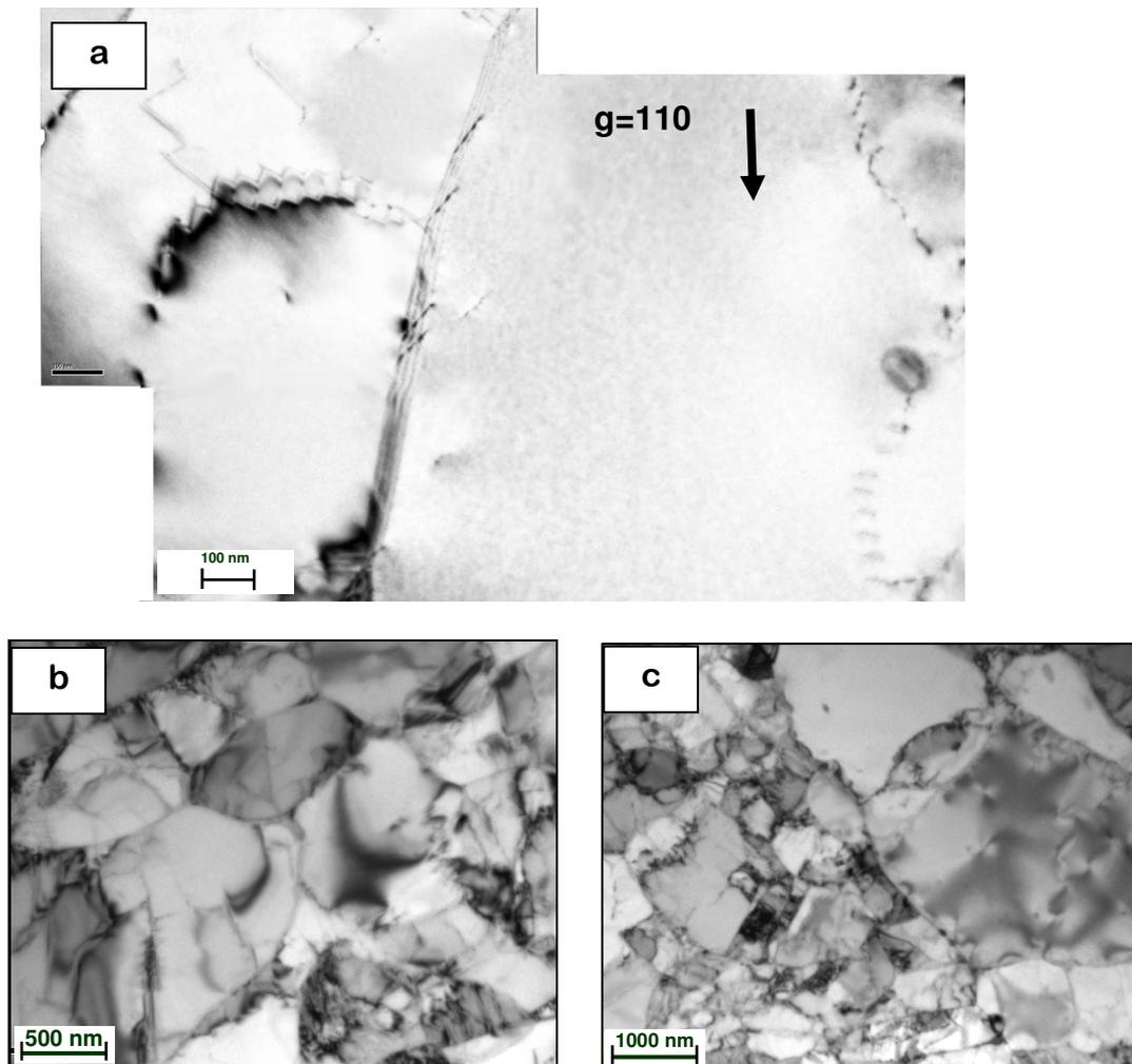
Figure 3.14. Bright field images obtained by TEM on the Fe-12%Cr alloy
