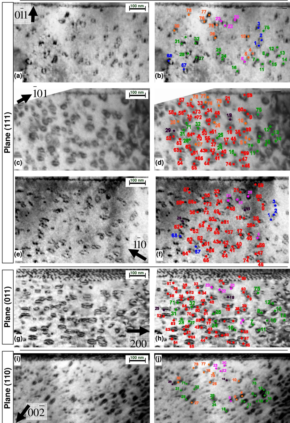
Figure 5.13. Bright field micrographs of the thin foil the Fe-12%Cr model alloy irradiated with 150 keV  $Fe^+$  ions at 500°C up to 1.5 dpa with different orientations imaged in five reflection conditions. Dislocations in the selected area have been numbered and identified on each micrograph (see Table 5.4).
