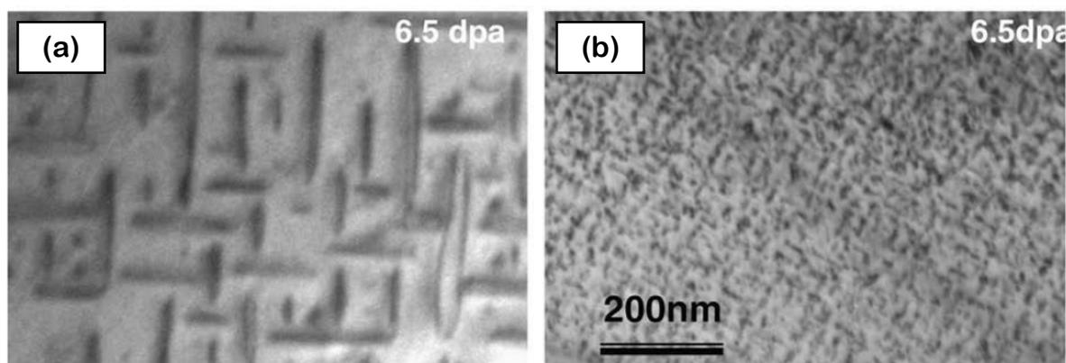
Figure 1.19. Comparison of high dose damage structures in ultra High purity Fe (a) and Fe–8%Cr (b) at irradiated with 100–150 keV  $\text{Fe}^+$  and  $\text{Xe}^+$  ion irradiation at 500 °C to 6.5dpa (from [69])
