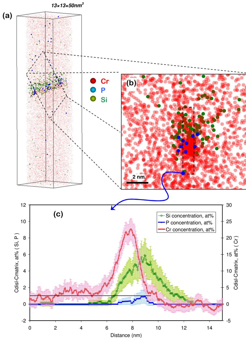
Figure 4.19. (a) 3D map of the analyzed volume of the Fe-5%Cr model alloy after neutron irradiation up to 0.6 dpa at 300°C. Only Cr, P and Si atoms are presented (b) Shift of Cr, Si and P enriched atmospheres with respect to the core of the dislocation; (c) concentration profile of the relative increase of Cr, Si and P drawn perpendicularly to the dislocation line through the core. Sampling box:  $15 \times 1 \times 1 \text{ nm}^3$ .
