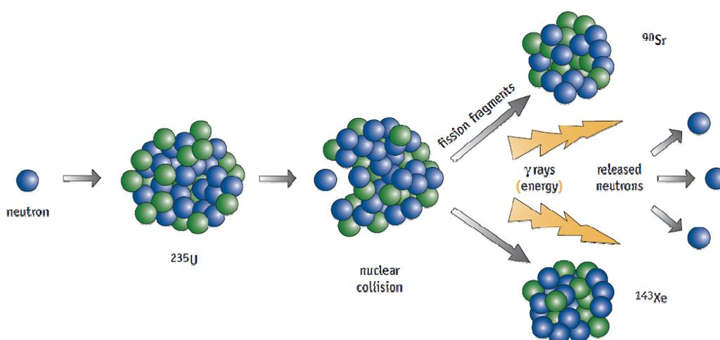
Figure 1.1. A typical fission reaction. When the nucleus of  $^{235}\text{U}$  absorbs an emitted neutron, it can fission or split into two fragments, releasing at the same time two or three neutrons and energy (from [7])
