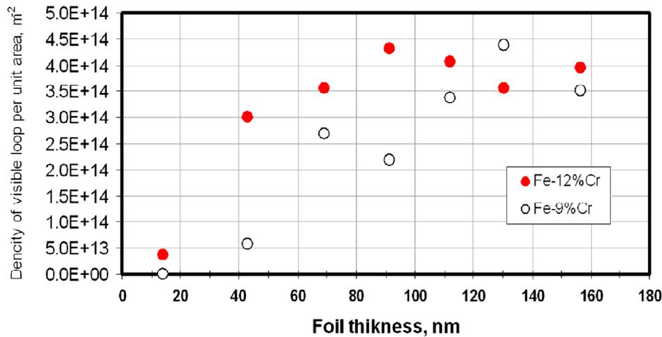
Figure 5.9. The density of visible loops per unit area as a function of foil thickness in the Fe-9%Cr and Fe-12%Cr alloys irradiated at 500°C with 150 keV Fe<sup>+</sup> ions up to 1.5 dpa. Measurements were made in a wedge-shaped foil imaged two-beam conditions using  $g=(\bar{1}\bar{1}0)$  in a foil oriented close to (111).
