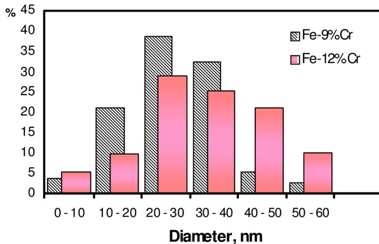
*Figure 5.11. The size distributions of visible dislocation loops in the Fe-9%Cr and Fe-12%Cr alloys irradiated at 500°C with 150 keV Fe<sup>+</sup> ions up to 1.5 dpa. Sizes have been deduced as a mean value of two measurements performed under two-beam conditions in the opposite g (( $\bar{1}\bar{1}0$ ) and ( $\bar{1}10$ )) in foils oriented close to (111). The results are based on measurements of 180 loops for the Fe-9%Cr alloy and 191 loops for the Fe-12%Cr alloy.*
