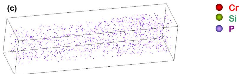
Figure 5.18. 3D distribution of chromium (a), silicon (b) and phosphorous (c) atoms in the Fe-9%Cr model alloy irradiated up to 1.5 dpa by  $Fe^+$  ions with energy 150keV at 500°C. All chemical species are homogeneously distributed after irradiation exposure
