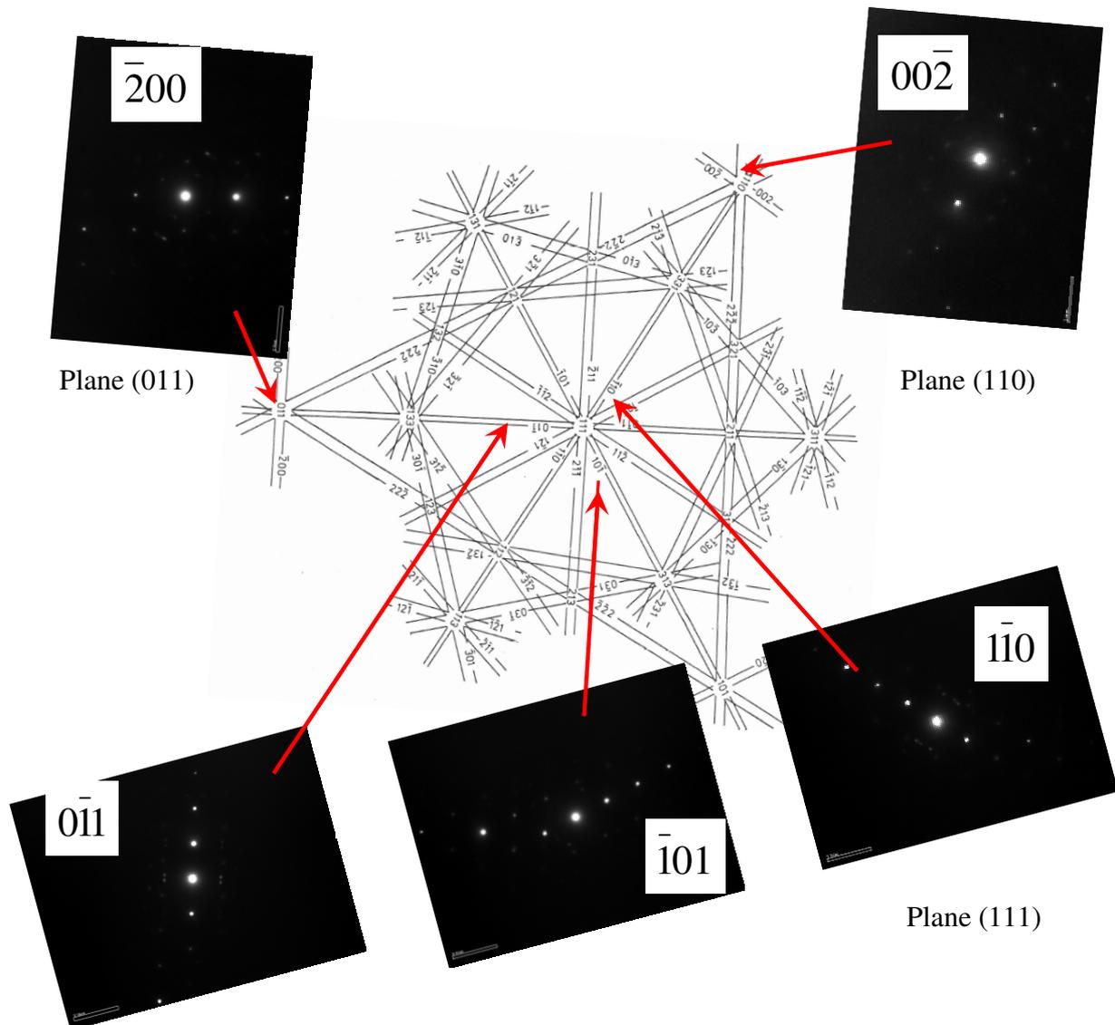
Figure 5.12. Schematic Kikuchi map for a b.c.c. Fe crystal centred on  $[111]$  direction. In order to determine the Burgers vectors of the loops in the Fe-12% Cr model alloys irradiated with 150 keV  $Fe^+$  ions at  $500^\circ C$  up to 1.5 dpa, 5 micrographs of dislocations have been taken in various reflection conditions which are presented on the diffraction patterns.
