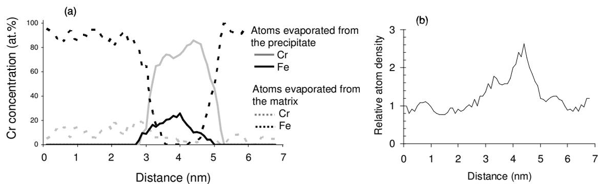
Figure 4.17. Concentration profile drawn through a precipitate of 1nm in radius which has been evaporated owing to a model that reproduces the field evaporation of an APT sample [23]. The actual Cr concentration of the simulated precipitate was 80%. It was placed in an Fe rich matrix which contains 14% of Cr atoms (after [16]).
