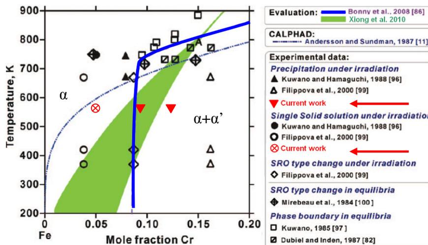
Figure 4.15. Low Cr part of the  $\alpha$ - $\alpha'$  miscibility gap (after [21]); the position of the  $\alpha$  domain limit, proposed by Bonny et al. is shown in blue [20]; the possible location for Fe-rich solvus determined by Xiong et al. [21] is presented by the green area. The results of the current research are shown by red marks (see explanation in the legend).
