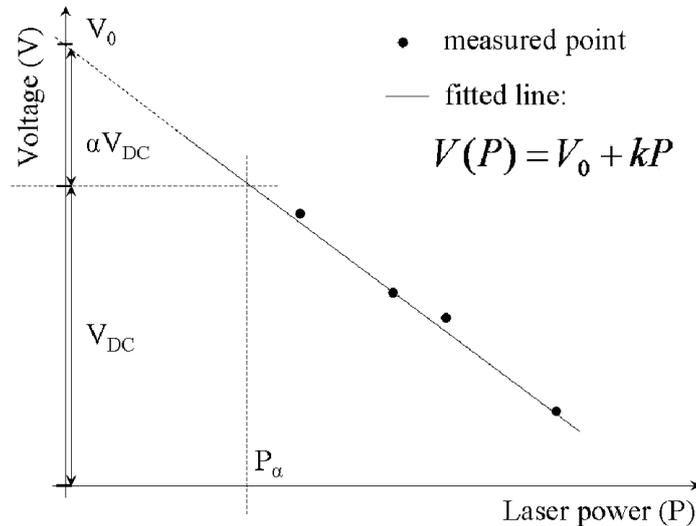
Figure 2.12. An example of equivalent pulse-fraction measurements.
