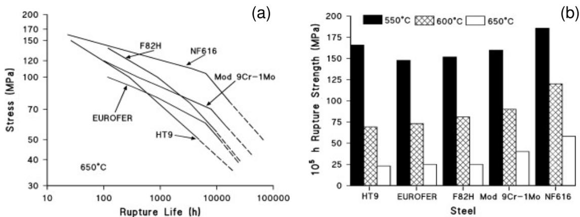
Figure 1.7. Comparison of the creep-rupture properties for commercial steels Sandvik HT9 (Gen - 1), modified 9Cr–1Mo(T91) (Gen - 2), NF616 (Gen - III), F82H (Gen - 1...2), and EUROFER (Gen - 1...2) (from [32])
