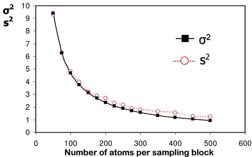
Figure 3.4. Comparison of the standard error ( $s$ ) of the experimental Cr-concentration frequency distribution with the standard deviation ( $\sigma$ ) of the binomial distribution in the un-irradiated Fe-5%Cr model alloy for sampling volume of different size. Experimental distribution almost coincides with the binomial one. Chromium atoms are homogeneously distributed.
