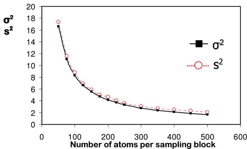
Figure 3.11. Comparison of the standard error ( $s$ ) with the standard deviation ( $\sigma$ ) in the as-received Fe-9%Cr model alloy. Experimental distribution almost coincides with the binomial one. Chromium atoms are homogeneously distributed.
