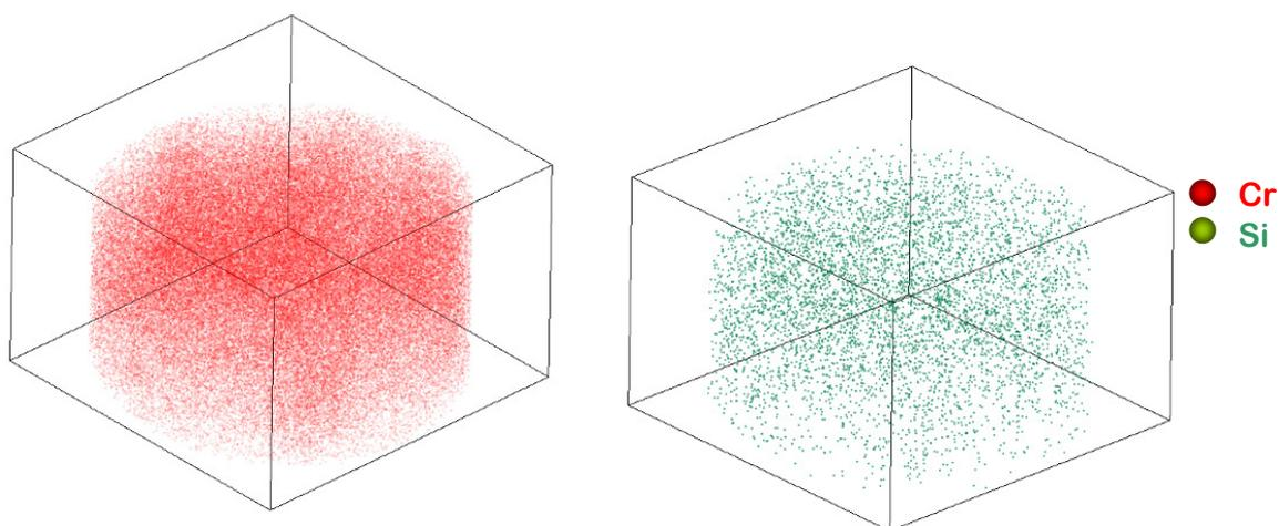
*Figure 5.17. 3D distribution of chromium (a) and silicon (b) atoms in the Fe-9%Cr model alloy irradiated up to 1.5 dpa by Fe<sup>+</sup> ions with energy 150keV at 300°C. Chemical species are homogeneously distributed after irradiation exposure*
