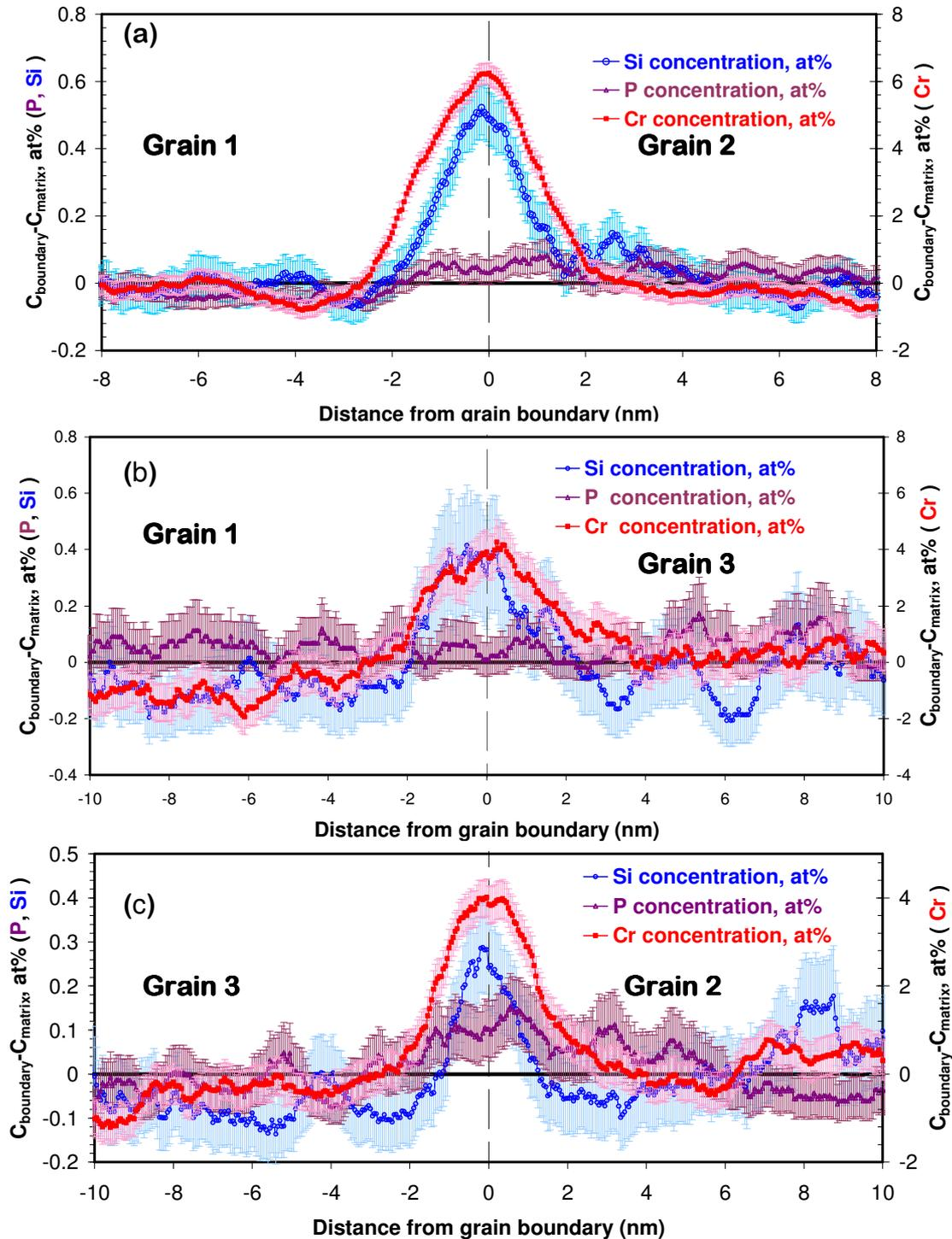
Figure 4.33. Variation of  $C_{\text{boundary}} - C_{\text{matrix}}$  measured across 3 grain boundary planes: (a) – from the grain No 1 to No 2, sampling volume ( $20 \times 30 \times 1 \text{ nm}^3$ ), (b) – from the grain No 1 to No 3, sampling volume ( $10 \times 10 \times 1 \text{ nm}^3$ ); (c) – from the grain No 3 to No 2, sampling volume ( $15 \times 15 \times 1 \text{ nm}^3$ ). The numbers of grains corresponds to the numbers in Figure 4.29
