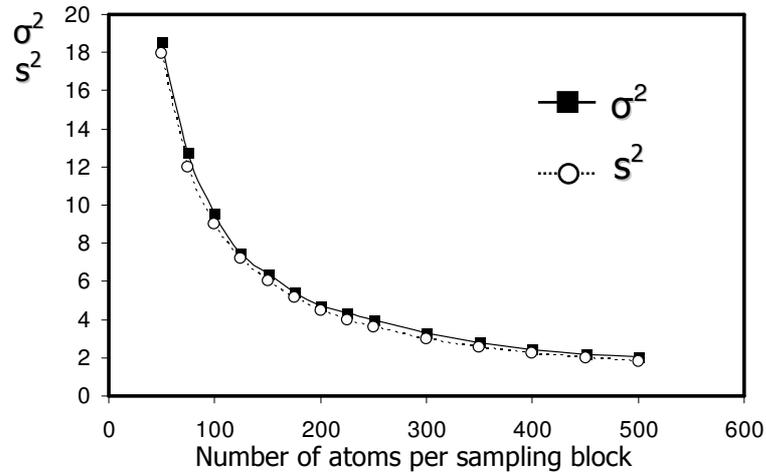
Figure 2.22. Comparison of the standard error ( $s$ ) of the experimental Cr-concentration frequency distribution with the standard deviation ( $\sigma$ ) of the binomial distribution in the un-irradiated Fe-12at%Cr model alloy for sampling volume of different size. Experimental distribution almost coincides with the binomial one. Chromium atoms are homogeneously distributed.
