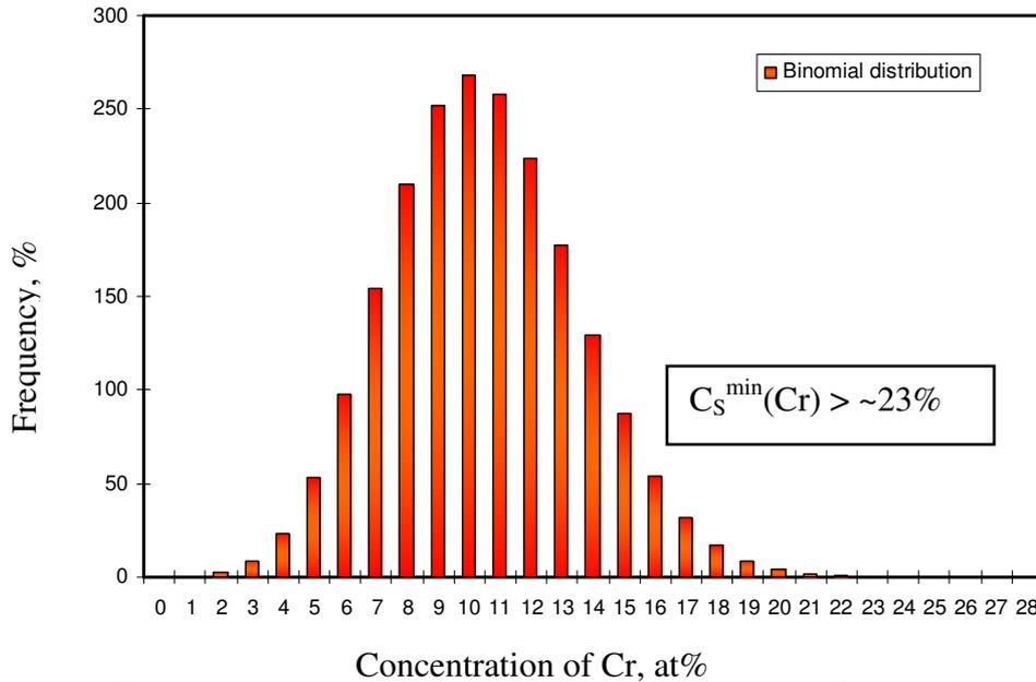
Figure 2.19. Frequency distribution of Cr atoms in the random Fe-10%Cr alloy. Sampling size:  $1.3 \times 1.3 \times 1.3 \text{ nm}^3$  (corresponds to about 200 atoms).
