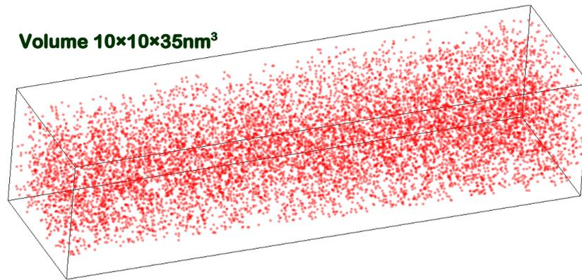
Figure 3.17. 3D distribution of chromium atoms in the as-received Fe-12Cr% model alloy. Each dot represents one atom. For clarity only chromium atoms are represented. Chromium atoms are homogeneously distributed before aging.
