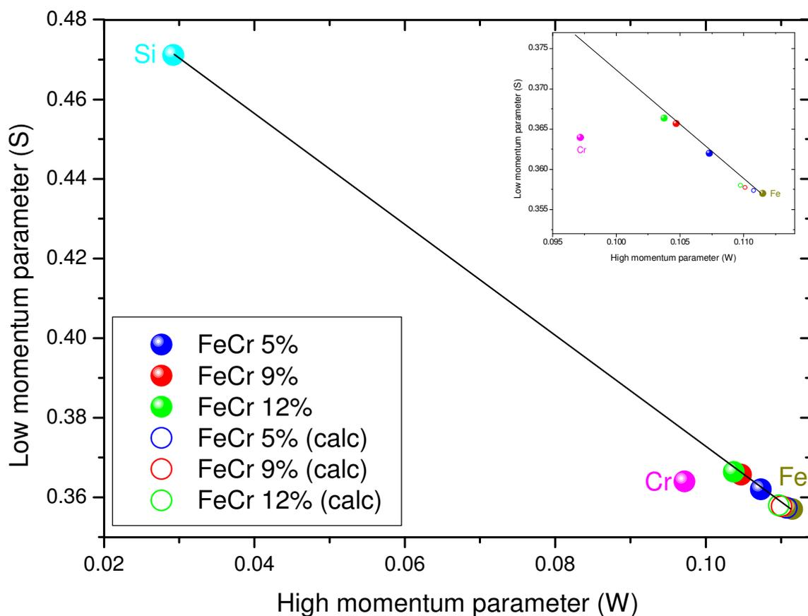
Figure 3.20. Evolution low momentum fraction ( $S$ ) as a function of the high momentum fraction ( $W$ ) for the second (bulk) layer in the un-irradiated Fe-5, 9 and 12%Cr model alloy.  $S(W)$  characteristic points of pure iron, chromium and silicon are also plotted. Empty circles represent the calculated  $S$  and  $W$  characteristic values for each model alloy considering their chemical compositions
