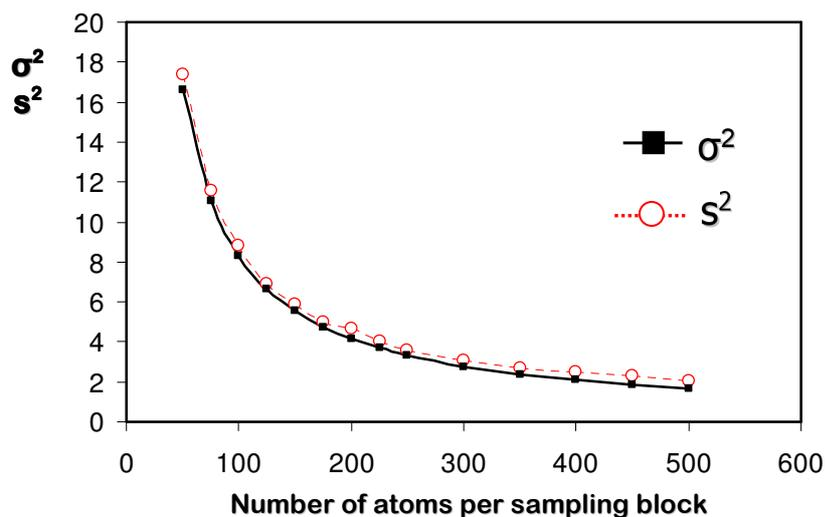
Figure 5.2. Comparison of the standard error ( $s$ ) with the standard deviation ( $\sigma$ ) in the Fe-9%Cr model alloy after 300 h of aging at 500°C. Experimental distribution almost coincides with the binomial one. Chromium atoms are homogeneously distributed.
