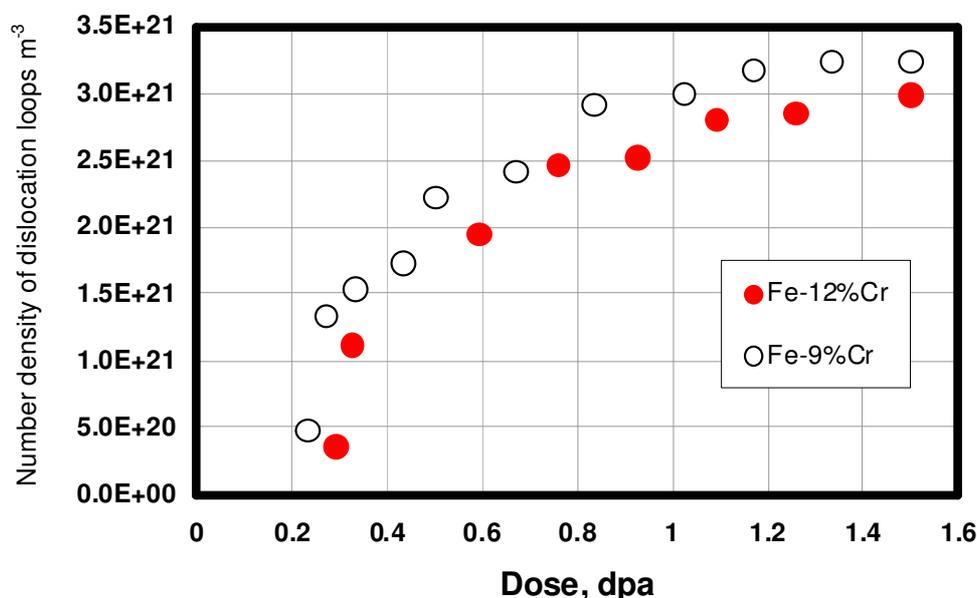
Figure 5.8. Number densities of visible dislocation loops as a function of dose in the Fe-9%Cr and Fe-12%Cr alloys irradiated at 500°C with 150 keV  $Fe^+$  ions.
