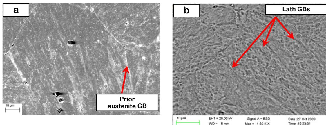
Figure 3.7. Results of SEM observation of the Fe-9%Cr alloy:
