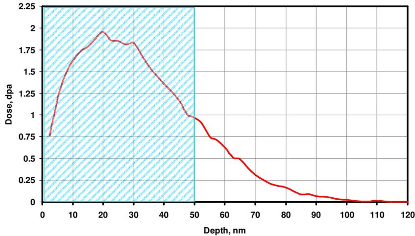
Figure 2.6. Distribution of damage after irradiation with 150 keV Fe<sup>+</sup> ions in an Fe-12Cr model alloy, calculated with SRIM 2008. Flux:  $1.6 \times 10^{15} \text{ m}^{-2} \text{ s}^{-1}$ ; fluence:  $4.32 \times 10^{18} \text{ ions} \cdot \text{m}^{-2}$ . The estimated fluence on the layer up to 50 nm (adapted to TEM and TAP samples) is 1.5 dpa
