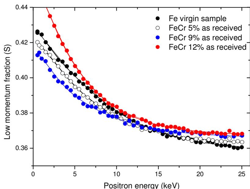
Figure 5. Variation of the  $S$  characteristic as a function of the positron energy for the pure Fe reference sample and for the Fe-Cr model alloys after electrochemical polishing
