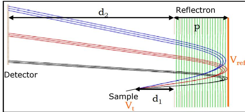
Figure 2.15. Scheme of principle of the reflectron (from [24])
