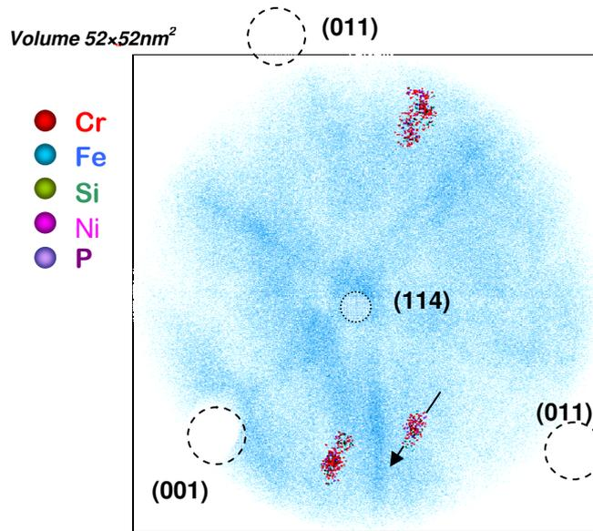
Figure 4.2. “Top view” of an analyzed volume of the Fe-5%Cr alloy after neutron irradiation at 300°C up to 0.6 dpa (the tip axis is normal to the figure) with indexed crystallographic poles. Only 10% of Fe atoms are represented on the 3D map of the matrix. Multicolor areas represent the NiSiPCr-enriched clusters. A threshold of  $C_{(Ni+Si+P)} > 3\text{at}\%$  is used to reveal the clusters. The clusters have an ellipsoidal shape.
