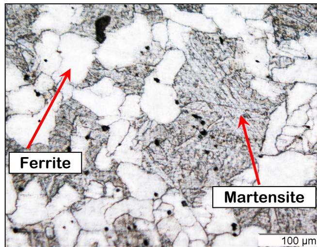
Figure 3.1. Metallography of the investigated Fe-5%Cr model alloy
