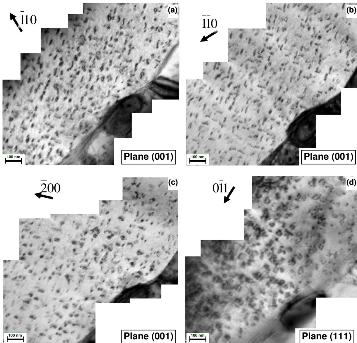
Figure 5.14 Bright field micrographs of the thin foil the Fe-9%Cr model alloy irradiated with 150 keV  $Fe^+$  ions at 500°C up to 1.5 dpa with different orientations imaged in four reflection conditions.
