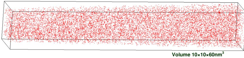
Figure 5.3. 3D distribution of chromium atoms in the Fe-12%Cr model alloy after 600h of aging at 500°C. Chromium is homogeneously distributed after the aging.
