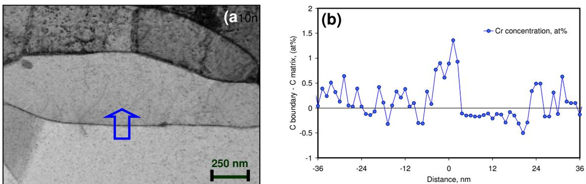
Figure 4.24. (a) Low angle annular dark field micrograph obtained on the as-received Fe-12%Cr (b) variation of  $C_{\text{boundary}} - C_{\text{matrix}}$  measured through the martensitic lath boundary (highlighted by blue arrow) showing Cr segregation across it.  $C_{\text{boundary}}$  is measured by EDX on the FIB-foil of about 50 nm in thickness,  $C_{\text{matrix}}$  is equal to the mean Cr content measured inside the two neighboring grains (11.1at%).
