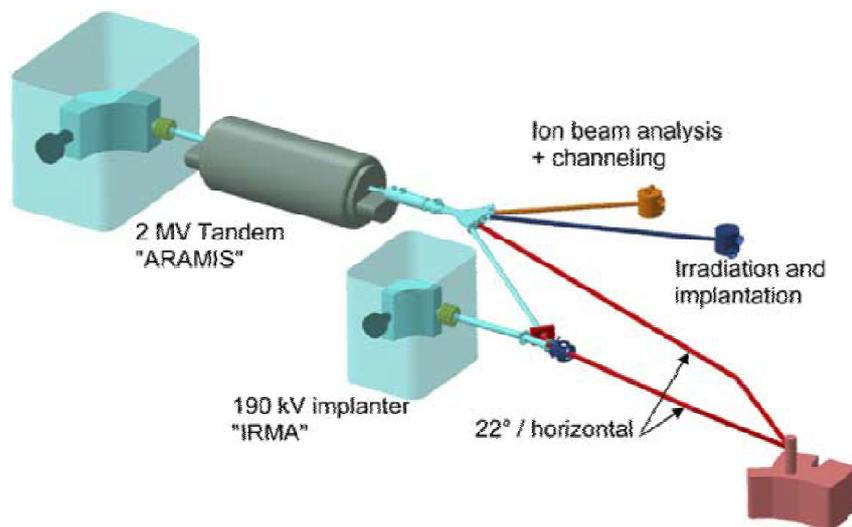
Figure 2.5. Scheme of the facilities of JANNUS installations(Orsay) : ARAMIS accelerator and IRMA implanter and their beam line (from [6]).
