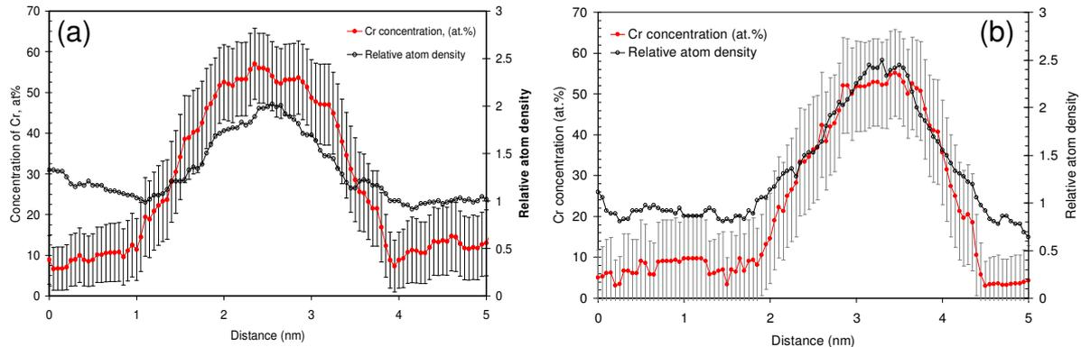
Figure 4.16. Cr-concentration profile drawn through a Cr-enriched clusters in the (a) Fe-9%Cr and (b) Fe-12%Cr model alloys and corresponding relative atom density.
