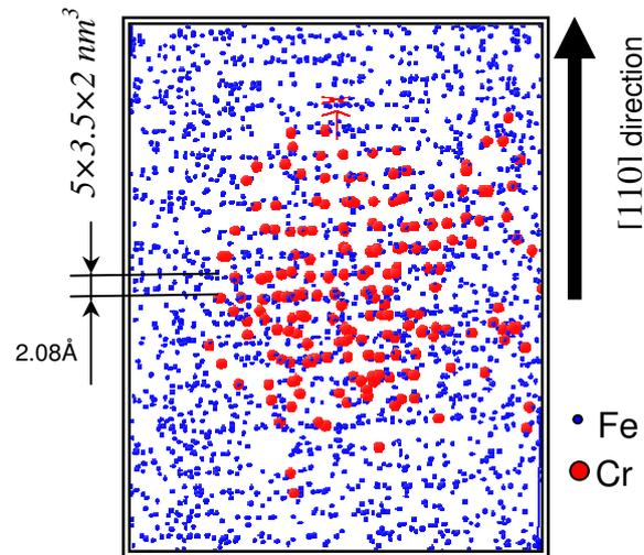
Figure 2.13. 3DAP image obtained in the alloy Fe-12%atCr after neutron irradiation at 300°C up to 0.6 dpa. The analyses have been performed in the [110] direction. Interplane distance in bcc Fe is  $\sim 2.03\text{\AA}$  that is in good corresponds to the value, obtained by TAP ( $2.08\text{\AA}$ ).
