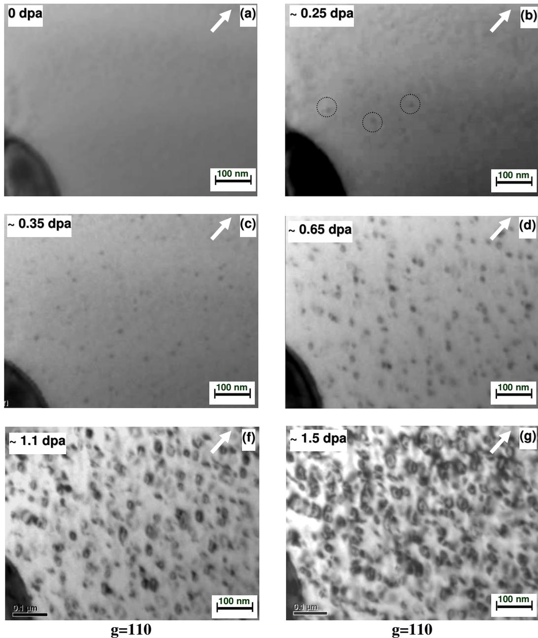
Figure 5.6. Evolution of the dislocation structure in the Fe-9%Cr model alloy during in-situ irradiation by  $Fe^+$  ions with energy 150keV at 500°C. The mean thickness of the foil in the imaged area is about 140nm. The micrographs have been captured from the film made under bright field conditions. The small dislocation loops became visible at dose range of about 0.25dpa (highlighted by black circles)
