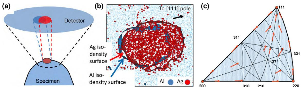
Figure 4.4. Schematic view of 'chromatic' aberrations in the case of small precipitates (b) Case of Ag-rich precipitates in a Al-Ag alloy. The Ag atoms are displaced towards the  $\{111\}$  pole; (c) Pole figure illustrating the direction of the Ag atom movement (from [15, 17])
