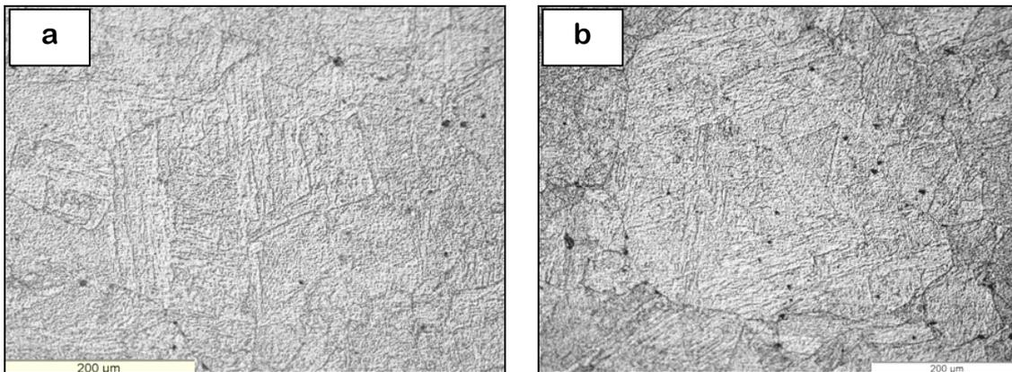
Figure 3.13. Metallography on the Fe-12%Cr model alloy: prior austenitic grains (with a broad distribution of grain size) have been transformed to lath martensite or upper bainite during  $\gamma \rightarrow \alpha$  transformation.
