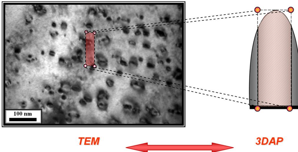
*Figure 5.15. Schematic comparison of the scales of investigated by TEM and by 3DAP. Consider the measured number density of the loops during the ion irradiation at 500°C ( $\sim 3 \times 10^{21} \text{ m}^{-3}$ ) and their mean size ( $\sim 30 \text{ nm}$ ), it has been estimated that in the typical LAWATAP experiment (volume of analysis is about  $40 \times 40 \times 100 \text{ nm}^3$ ) we can expect to have half of a full dislocation loop*
