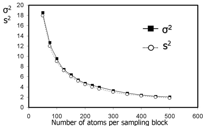
Figure 3.18. Comparison of the standard error ( $s$ ) with the standard deviation ( $\sigma$ ) in the as-received Fe-12%Cr model alloy. Experimental distribution almost coincides with the binomial one. Chromium atoms are homogeneously distributed.
