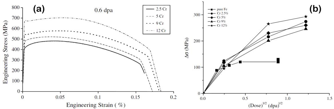
Figure 2.4. a) Tensile tests at room temperature of model alloys after neutron irradiation at 300°C up to 0.6 dpa; b) increase in room temperature yield strength upon irradiation at 300°C,  $\Delta\sigma_Y$  vs  $(\text{dose})^{1/2}$  (from [2])
