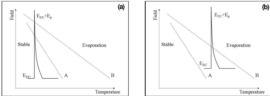
Figure 2.16. Influence of electric field on the specimen's tip on the evaporation conditions of chemical species A and B: a) proper evaporation conditions; b) preferential evaporation conditions for A.
