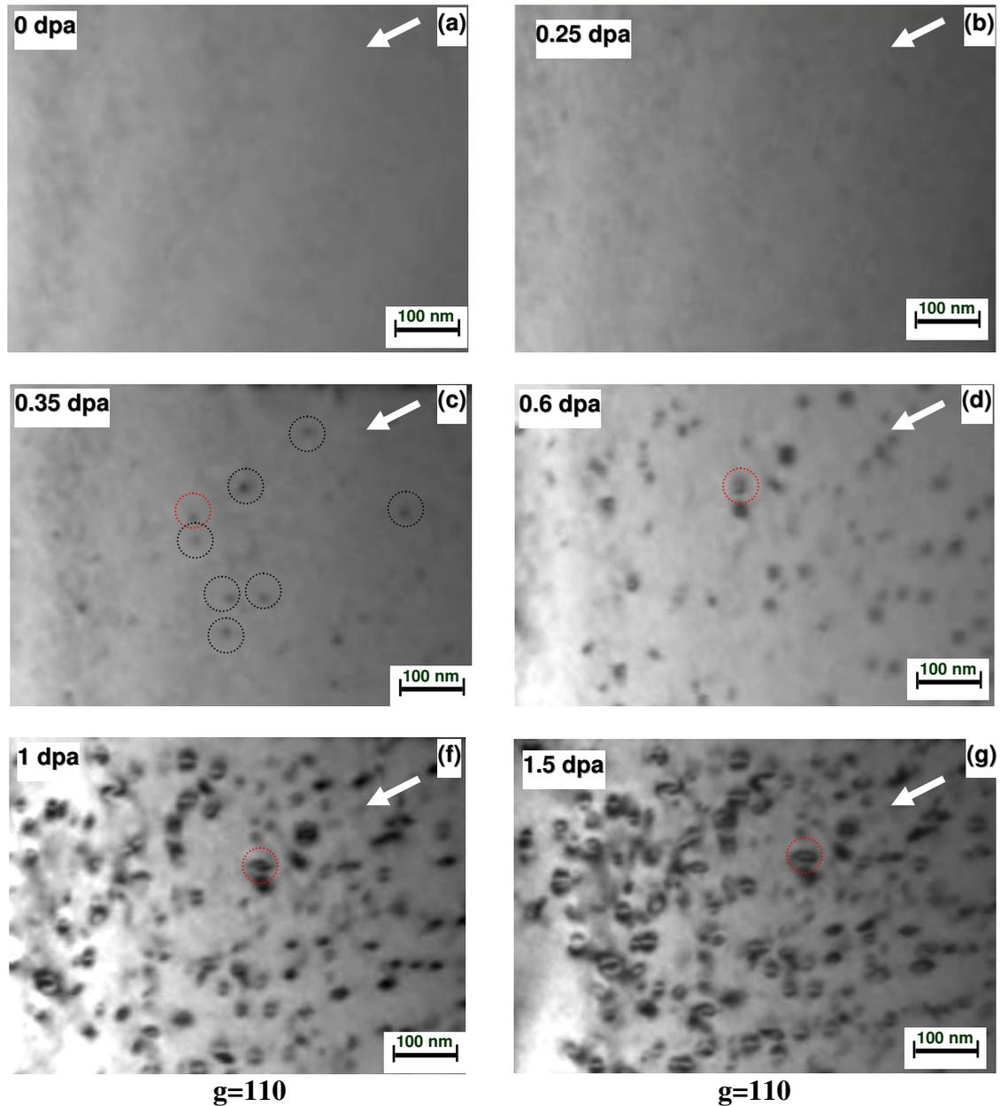
Figure 5.7. Evolution of the dislocation structure in the Fe-12%Cr model alloy during in-situ irradiation by  $Fe^+$  ions with energy 150keV at 500°C. The mean thickness of the foil in the imaged area is about 100 nm. The micrographs have been captured from the film made under bright field conditions. The small dislocation loops became visible at dose range of about 0.35dpa (highlighted by black circles). The evolution of the size of the dislocation loop is highlighted by red circle.
