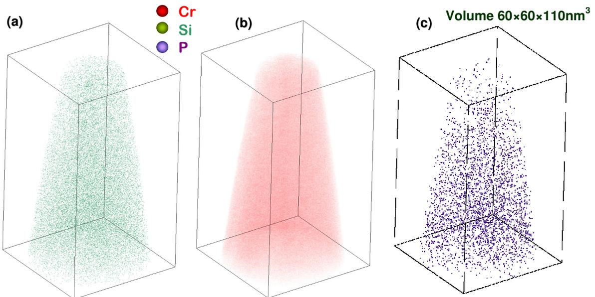
Figure 5.19. 3D distribution of chromium (a), silicon (b) and phosphorous (c) atoms in the Fe-12%Cr model alloy irradiated up to 1.5 dpa by  $Fe^+$  ions with energy 150keV at 500°C. All chemical species are homogeneously distributed after irradiation exposure
