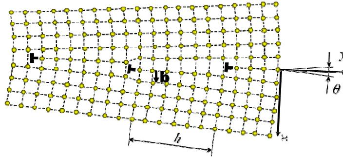
Figure 4.27. Diagram of the structure of tilt sub-grain boundary which consist of edge dislocations
