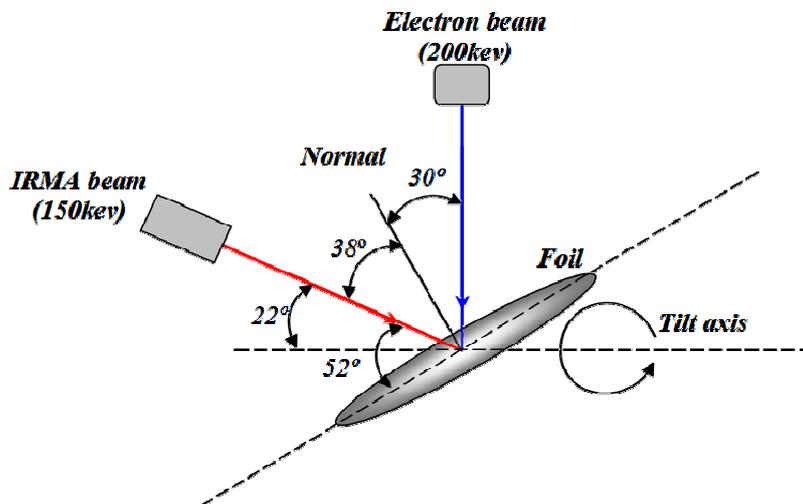
Figure 2.7. Scheme of in-situ TEM ion irradiation experiment.
