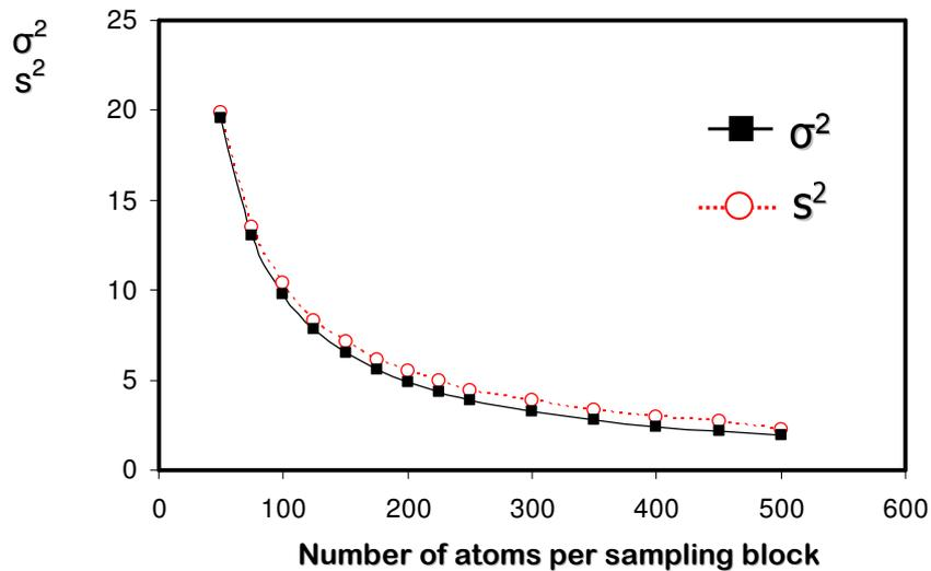
Figure 5.4. Comparison of the standard error ( $s$ ) with the standard deviation ( $\sigma$ ) in the Fe-12%Cr model alloy after 600 h of aging at 500°C. Experimental distribution almost coincides with the binomial one. Chromium atoms are homogeneously distributed.
