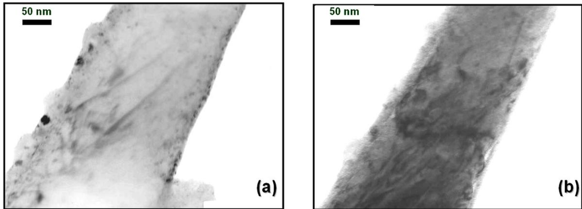
Figure 5.16. TEM investigation of the 3DAP tips of the Fe-9%Cr(a) and Fe-12%Cr (b) model alloys after irradiation by  $Fe^+$  ions with energy 150keV at 300°C. The contrast of some objects appropriates with the presence of dislocations. It can be expected that the possible segregation on dislocations can be registered by 3DAP experiments
