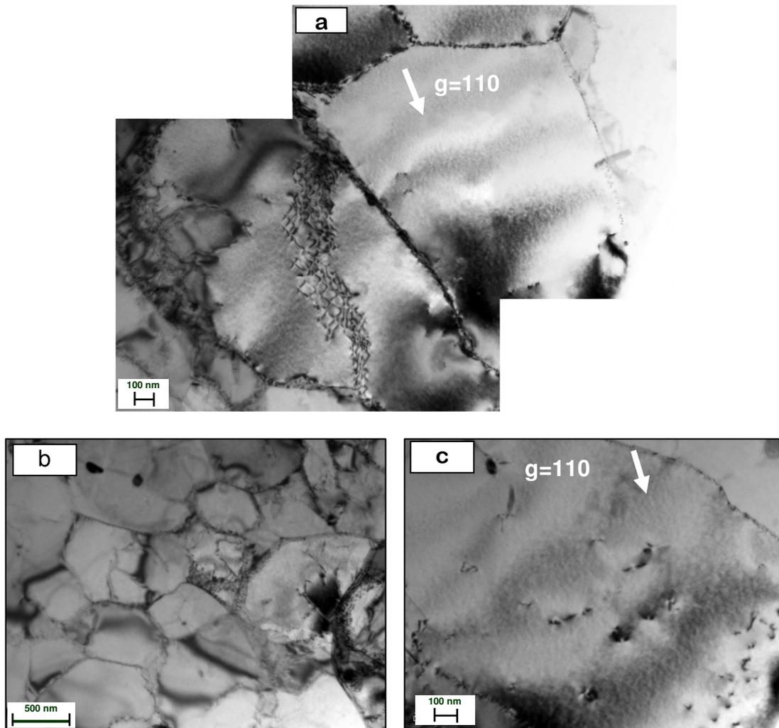
Figure 3.9. Bright field images obtained by TEM on the Fe-9%Cr alloy
