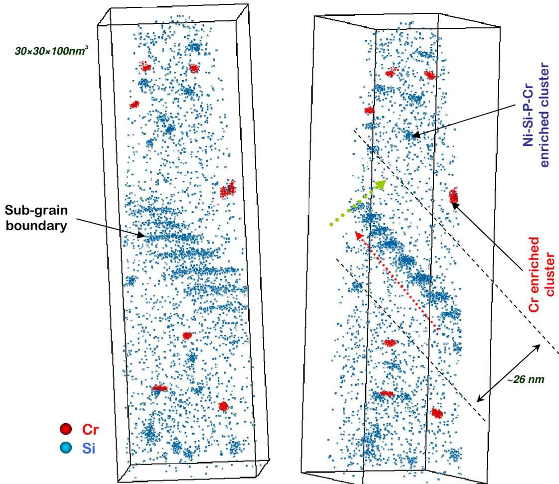
Figure 4.29. (a) and (b) 3D distribution of Si and Cr atoms of an analyzed volume of the Fe-9%Cr alloy after neutron irradiation at  $300^\circ\text{C}$  up to 0.6 dpa. Only Cr atoms which are inside Cr-enriched clusters are presented (Cr concentration is higher than 24at.%) whereas all the Si atoms are shown (in blue). Colored arrows show the direction of the composition profiles drawn across (green arrow, see Figure 4.30(a)) and inside (red arrow, see Figure 4.30(b)) sub-grain boundary.
