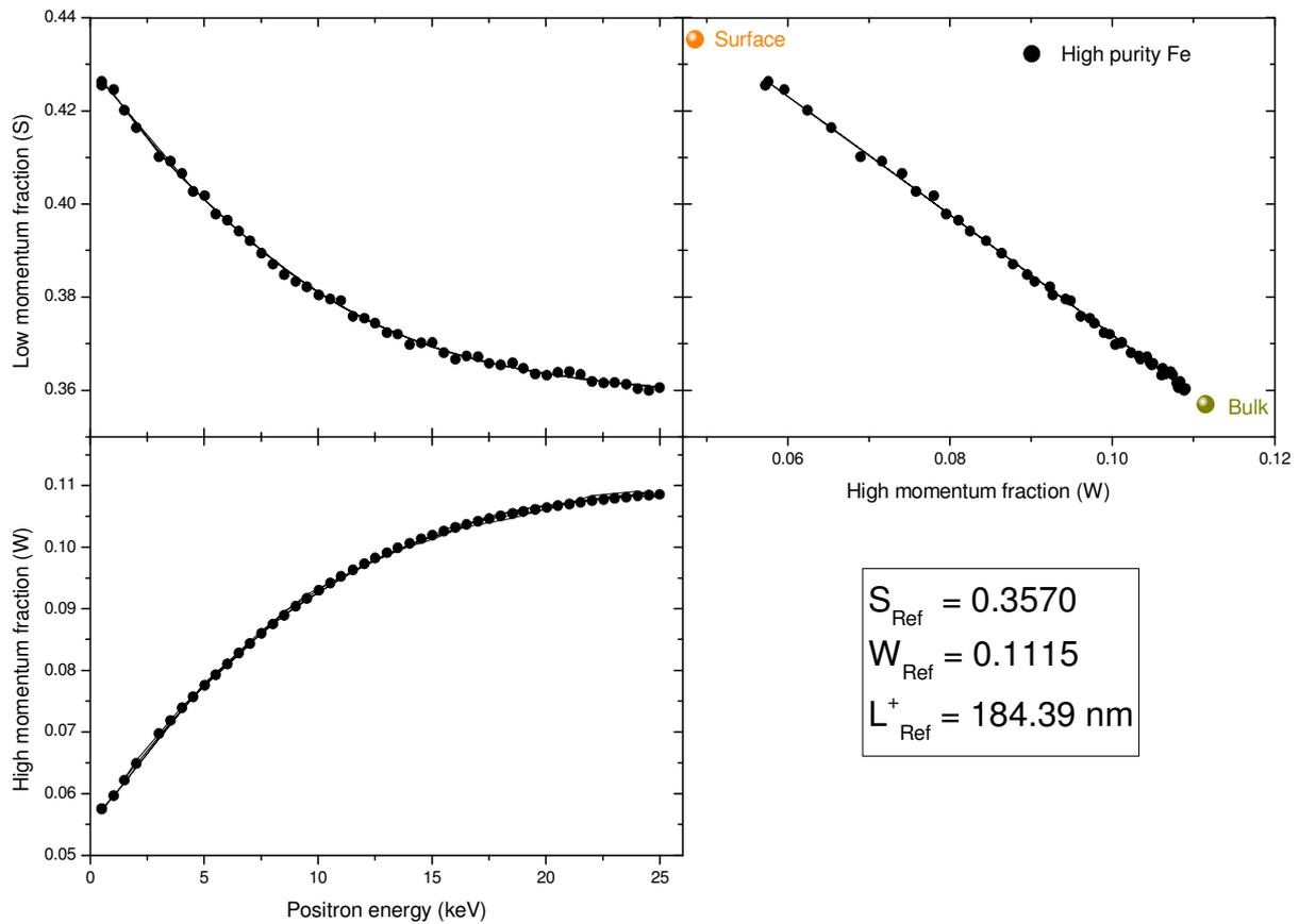
Figure 2.27. Variation of the characteristic  $S$  and  $W$  as a function of the positron energy for the pure Fe reference sample. The effective diffusion length of positrons  $L^+$  is equal to about 184 nm
