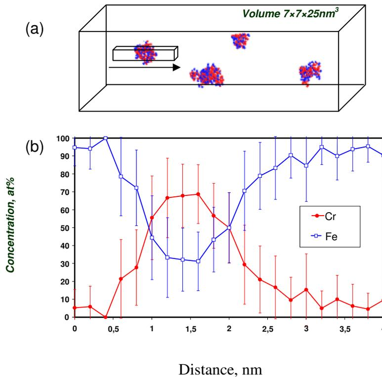
Figure 2.20. Atom probe analysis of the Fe-12Cr model alloy neutron irradiated at  $300^\circ\text{C}$  up to 0.6 dpa: a) Filtered 3D image of the alloy. Concentrated zones represent the Cr-enriched clusters. A threshold of 28at% is applied to distinguish  $\alpha'$  from  $\alpha$  phase; b) composition profile drawn along the parallelepiped indicated in (a). Sampling size:  $0.7 \times 0.7 \times 0.7 \text{ nm}^3$
