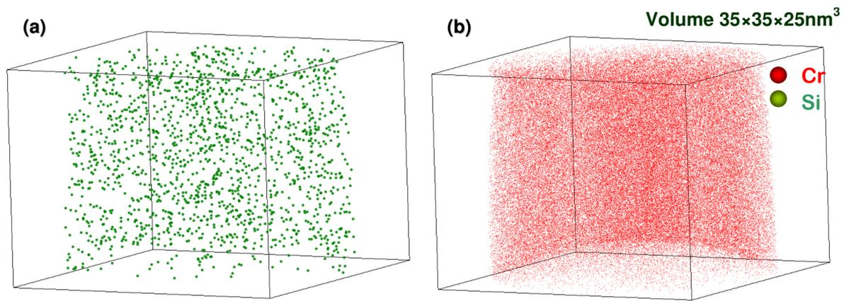
*Figure 5.20. 3D distribution of silicon (a) and chromium (b) atoms in the Fe-12%Cr model alloy irradiated up to 1.5 dpa by  $\text{Fe}^+$  ions with energy 150keV at 500°C. All chemical species are homogeneously distributed after irradiation exposure*
