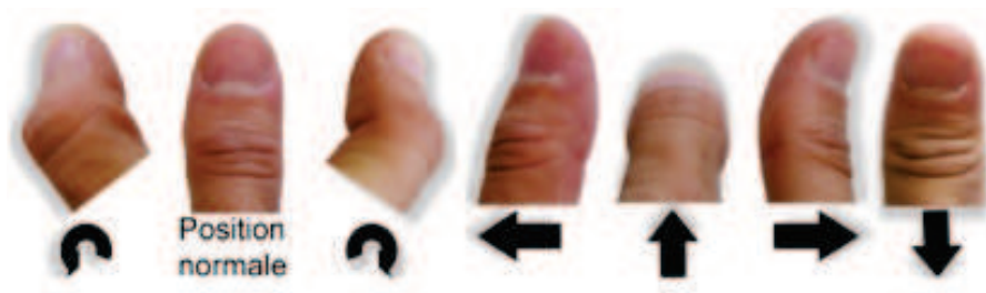
Figure 1.6.: Roudaut proposes the exploitation of micro-gestures on touch screen based devices with “Microrolls” [Roudaut 10].
