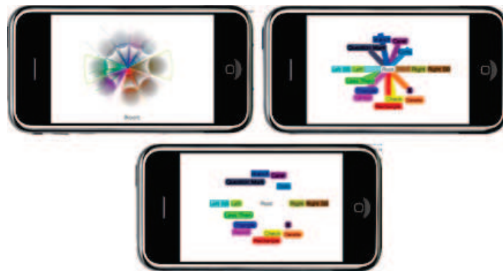
Figure 7.8.: Different GUI aspects can be associated to the same gestural menu. The first row shows the two default GUI aspects integrated in the library. The first one is an accurate representation of the functioning of the underlying algorithm. The second one is an OctoPocus-like view of a GeLaTI menu. The second row shows a third GUI aspect designed to imitate the Marking Menu.
