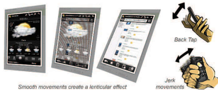
Figure 4.5.: Tapping the back of the device trigger the continuous/discrete mode. In continuous mode application switch is activated by tilting the device. In discrete mode application switch is achieved using jerk movements [Roudaut 09].
