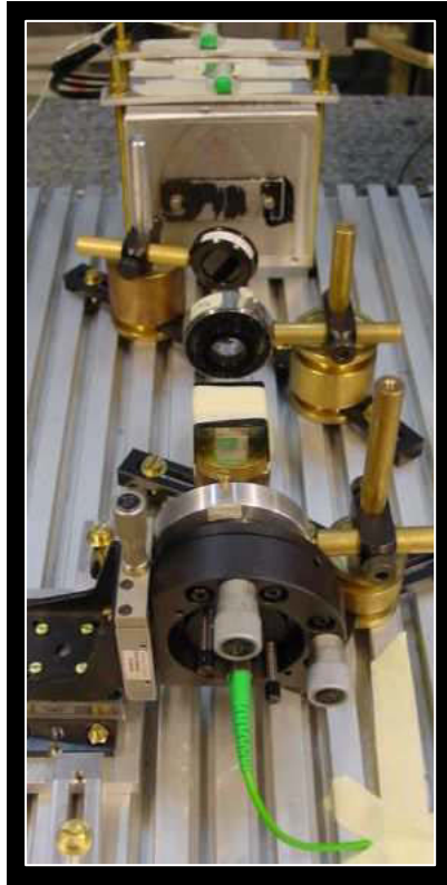
Figure 3.6: Additional optical setup: Injection of the probe laser (single-frequency DBR laser diode) into an optical fibre. The following optical elements are used (from top to bottom): Aluminium housing of the laser diode (with closed cover plate on the photo), inclined neutral density filter (to avoid feedback into the laser diode and reduce laser intensity), \lambda/2 halfwave plate (to rotate polarisation plane for laser intensity control), polarising beam splitting cube and \lambda/4 quarterwave plate (serve as optical isolator) and precisely adjustable fibre mount.
