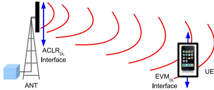
Figure 3.18.: Measurement points for ACLR and EVM for a downlink signal
