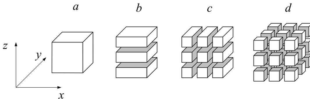
Figure 5.2: Domain decomposition in a cartesian topology. *a*) Original (serial) domain, *b*) one-dimensional decomposition, *c*) two-dimensional and *d*) domain decomposition in the three cartesian directions.
