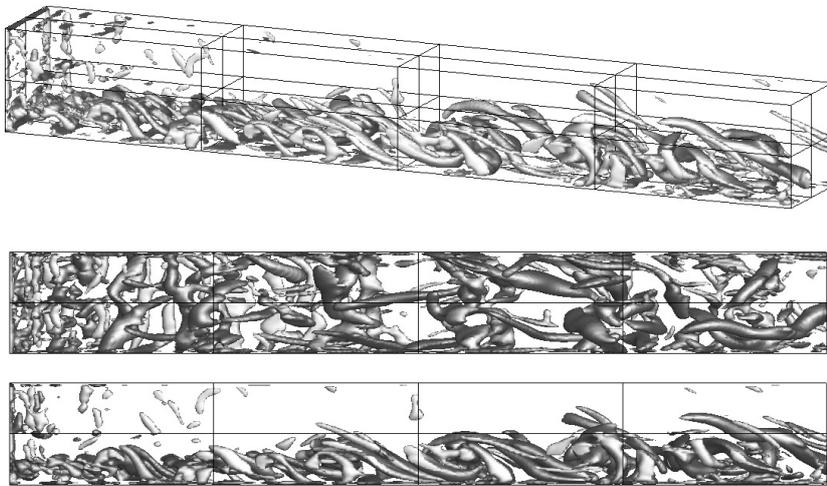
Figure 7.16: Perspective, top and lateral views of the isosurface of the second invariant of the velocity-gradient tensor  $Q = 2^6$ , at  $t = 0.020$  s. The method of Klein, Sadiki and Janicka (2003) was used.
