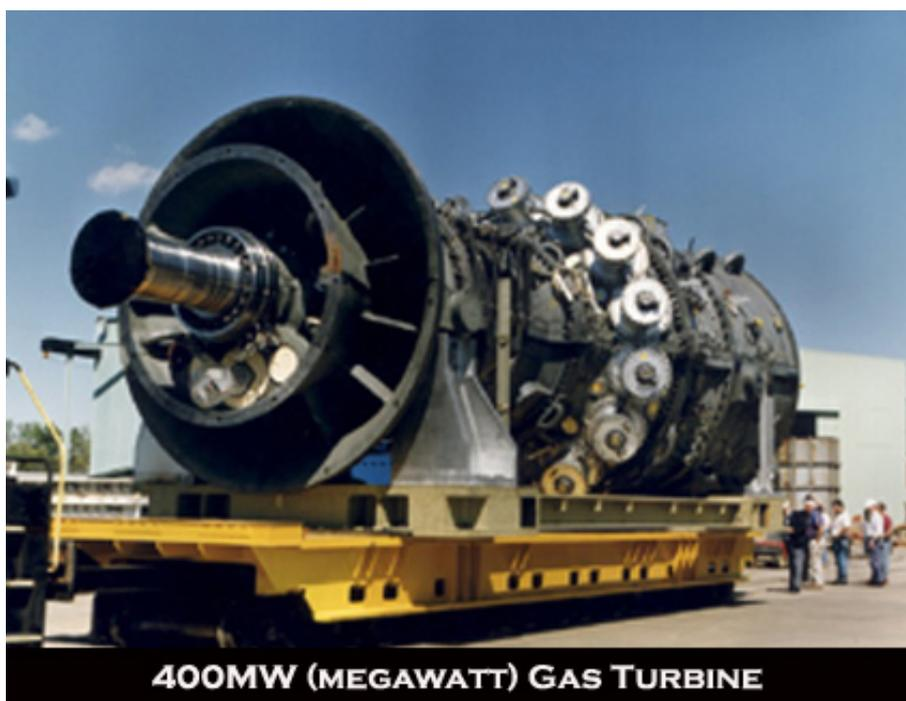
Figure 1.1: A 400MW gas turbine, <http://www.global-greenhouse-warming.com/gas-as-a-wedge-against-carbon-emissions.html>, accessed on 16/08/2011.
