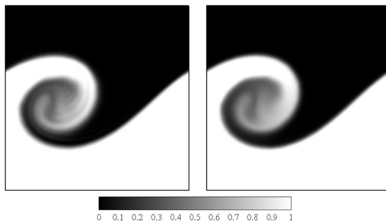
Figure 4.12: Two-dimensional temporal mixing layer simulation results for a density ratio  $s = 2$  at  $t^* = tU_r/L_r = 54$ . Contours of the scalar  $c$ . The figure in the right hand side presents results for the simulation using the finite volume scheme. In the left hand side, results of the Monte-Carlo simulation.
