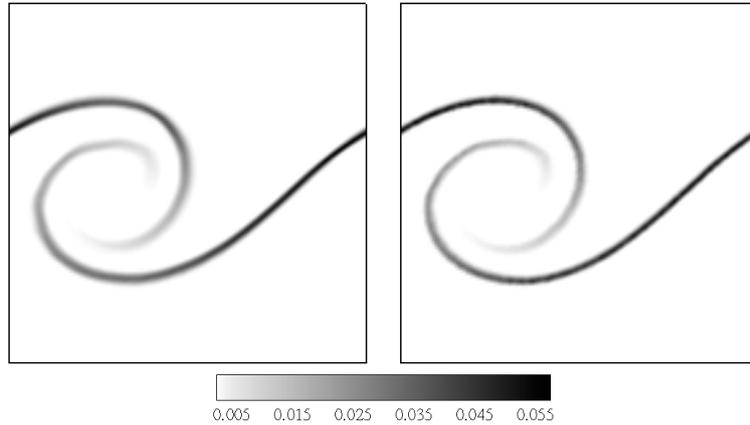
Figure 4.13: Two-dimensional temporal mixing layer simulation results for a density ratio  $s = 2$  at  $t^* = tU_r/L_r = 50$ , where  $t$  is the physical time. Contours of the variance of the scalar  $c$ . The figure in the right hand side presents results for the simulation using the finite volume scheme. In the left hand side, results of the Monte-Carlo simulation.
