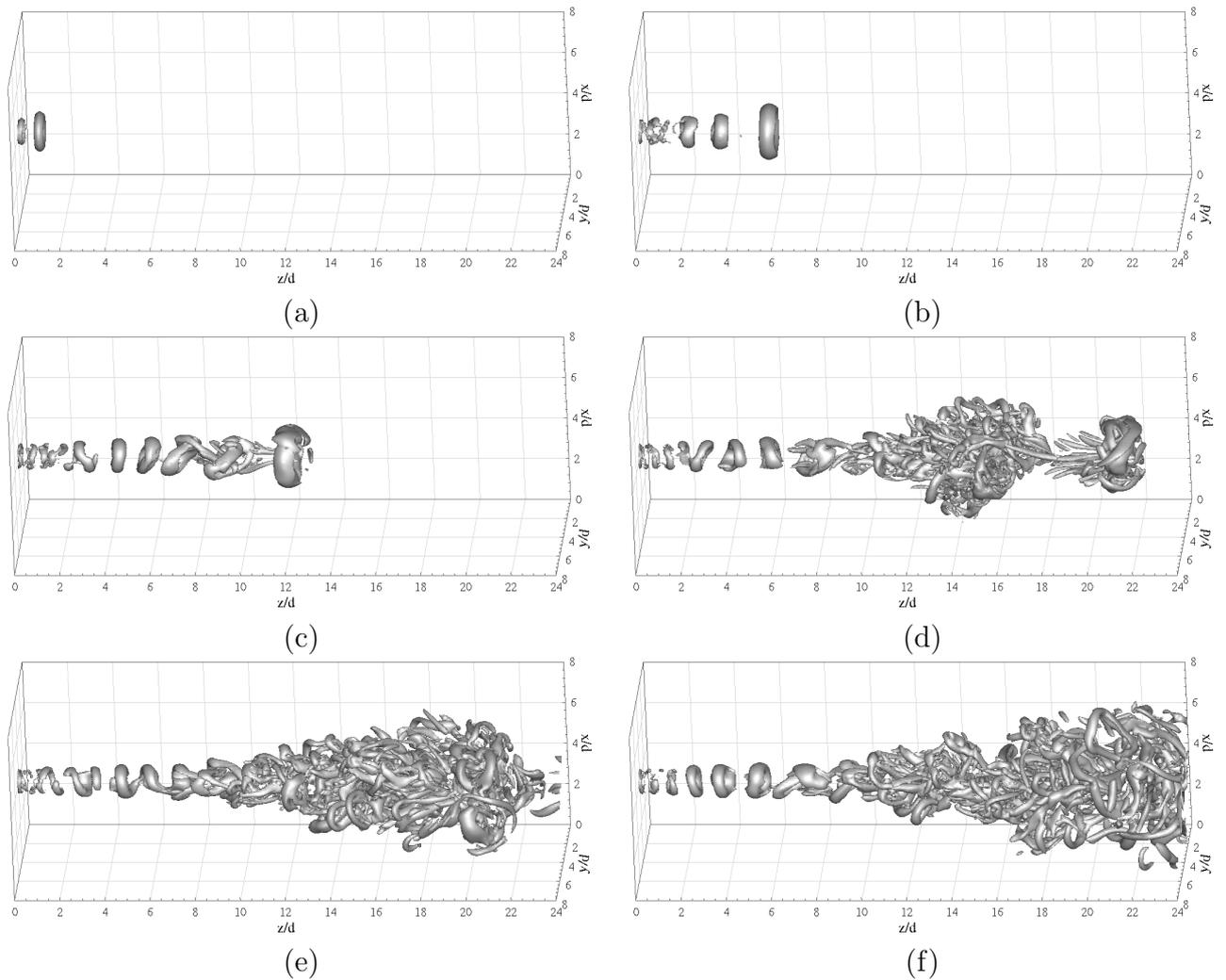
Figure 2.3: Temporal evolution of  $Q = 0, 1$  [s<sup>-1</sup>] isosurfaces: (a)  $t=0.1$  [s], (b)  $t=5$  [s], (c)  $t=10$  [s], (d)  $t=20$  [s], (e)  $t=30$  [s] e (f)  $t=40$  [s]. (MOREIRA, 2011).
