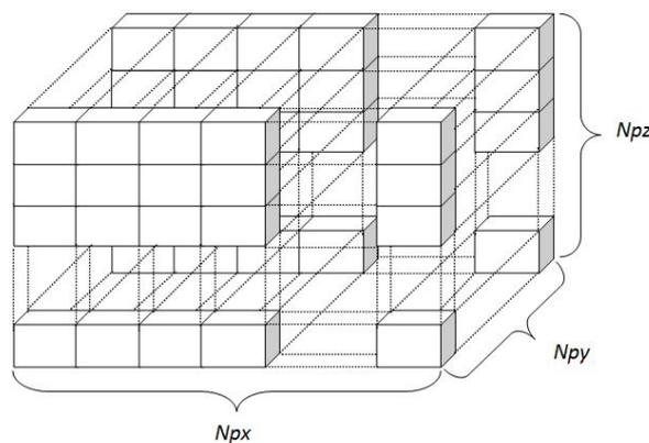
Figure 5.1: Domain decomposition in a three-dimensional cartesian topology.  $Np_x$ ,  $Np_y$  and  $Np_z$  stand for, respectively, the number of processes in the  $x$ ,  $y$  and  $z$  directions
