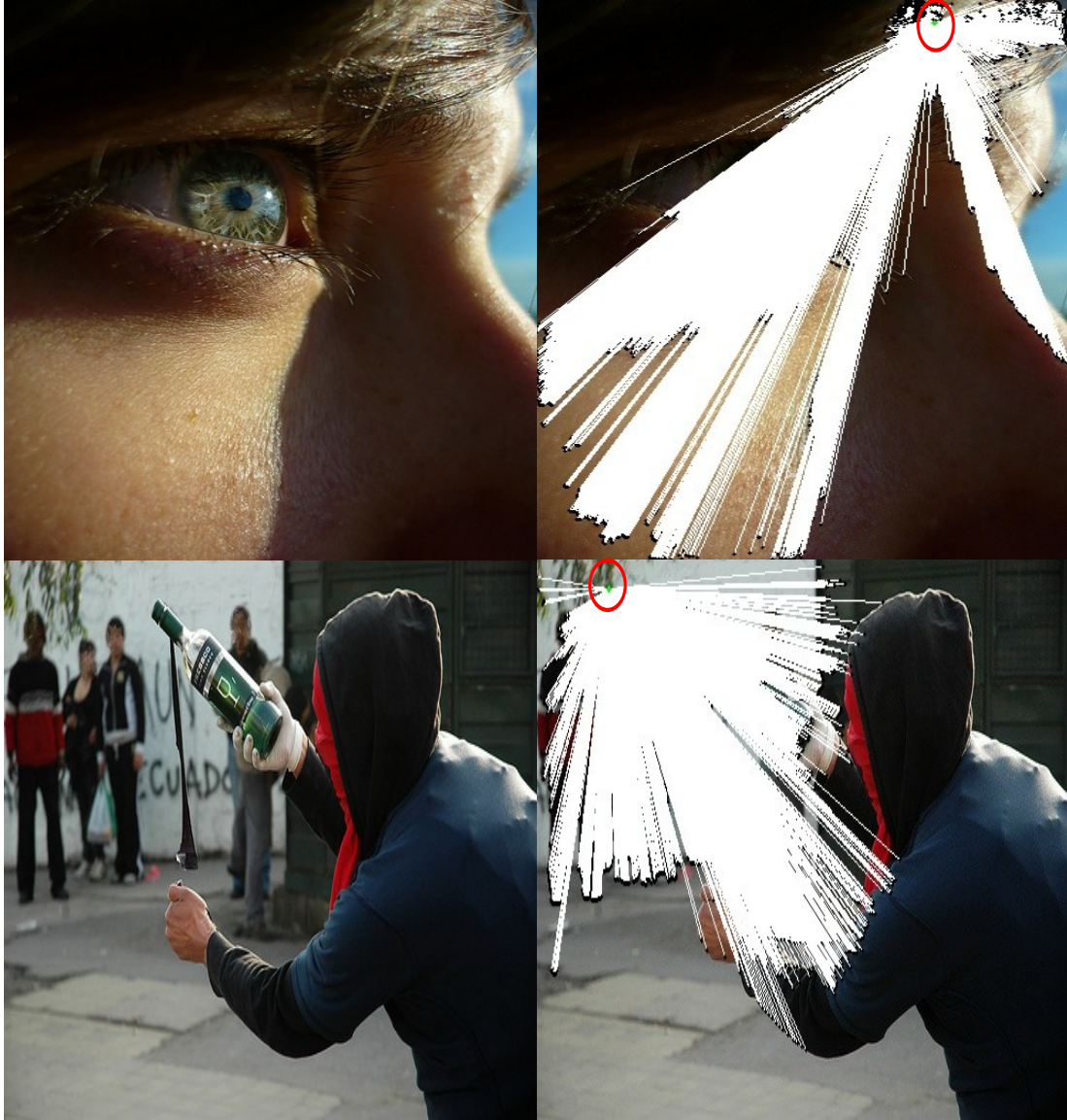
Figure 5.10: Examples of vectors (white lines) drawn from a given interest point (green dot inside the red circle) to all other edge points (black points) that are in the same 5D Gaussian cluster as the interest point.
