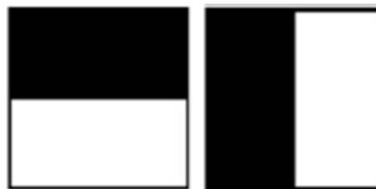
Figure 5.8: Haar wavelet types used for SURF.
