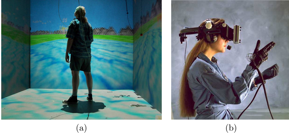
Figure 1.1: Two widely used immersive systems: the Cave Automatic Virtual Environment (a) and the classic goggles and gloves (b). Their goals are to replace most of the user's perceptions of the real world by virtual ones and to make the interaction with the environment more natural.
