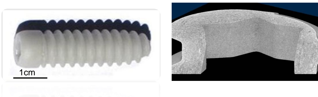
Figure 3: Photograph and computed X-tomography of the upper part of the P(L,DL)LA/Bioglass® 45S5 (30 wt.%) composite screw (ActiKER™, Noraker, France) processed by injection moulding.
