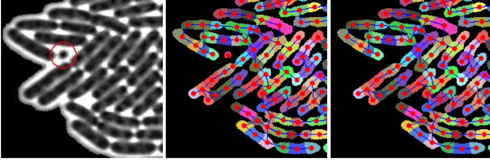
Figure 17: Clean-up of spurious blobs. The bright halo around the cells has left a small patch of dark pixels in the colony (highlighted in red), which has been detected as a small blob seed that has no neighbor in the connection graph. Such over-segmentation artifacts are easy to detect and eliminate.
