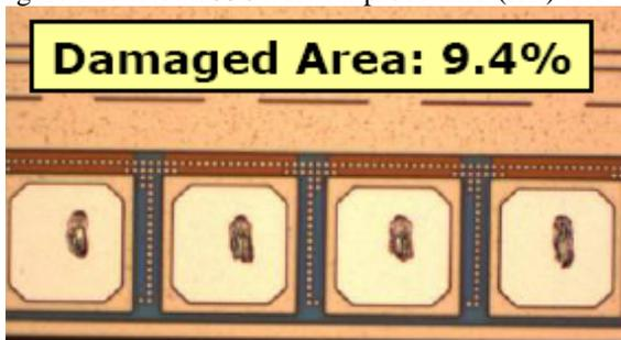
Figure I.18. Scrub mark induced by probing with cantilever PC [Vallauri, 2007].
