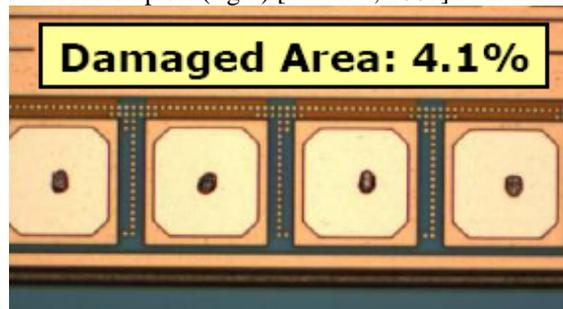
Figure I.19. Scrub mark induced by probing with Route60@ vertical PC [Vallauri, 2007].
