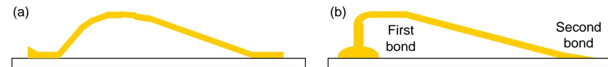
Figure I.27. Typical geometrical configurations for ultrasonic wedge bond (a) and for gold ball bond (b)
