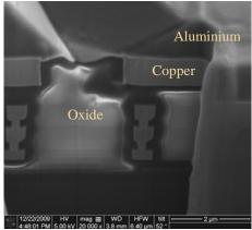
Figure IV.47. SEM cross section after FIB milling of the sample 6.
