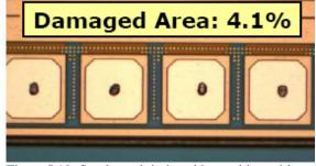
Figure I.19. Scrub mark induced by probing with Route60® vertical PC [Vallauri, 2007].
