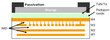
Figure IV.1. Schematic cross section of the evaluated CMOS 120nm pads.
