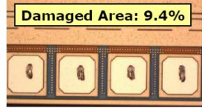
Figure I.18. Scrub mark induced by probing with cantilever PC [Vallauri, 2007].
