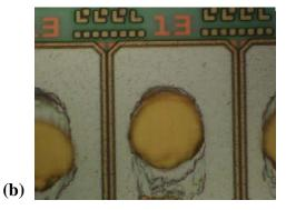
Figure III.26. Failure mode 1 (a) without gold remaining on the pad and failure mode 2 (b) with gold remaining.
