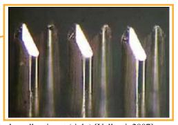
Figure I.17. Route60® vertical probe card (left) and vertical needles tip set (right) [Vallauri, 2007].
