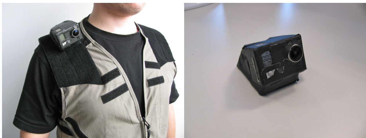
Figure 1.2: Video lifelog recording device used in the IMMED project, which is one applicative context of this work: (left) vest with autonomous video camera; (right) detachable video camera composed of camera, battery and memory card
