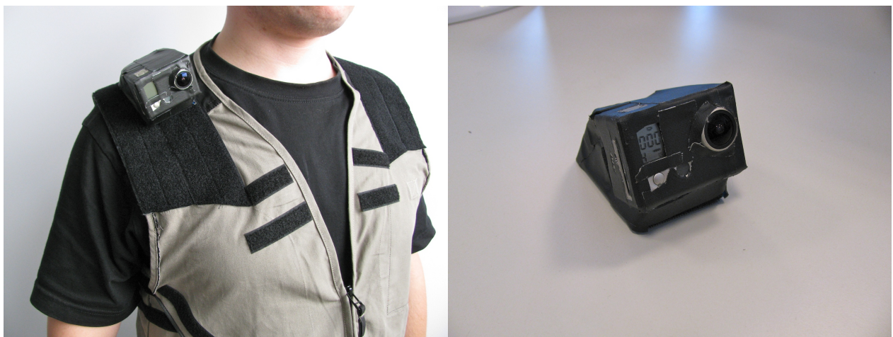
Figure 1.2: Video lifelog recording device used in the IMMED project, which is one applicative context of this work: (left) vest with autonomous video camera; (right) detachable video camera composed of camera, battery and memory card
