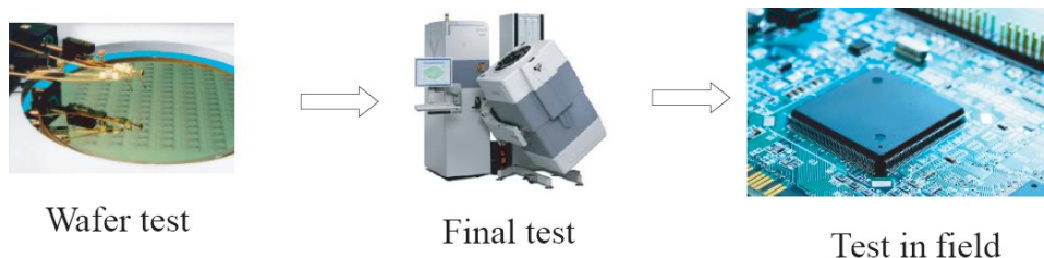
Figure 2.1: Different test steps of an IC.
