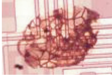
Figure 2.14: Example of an internal contaminant on the die [7].
