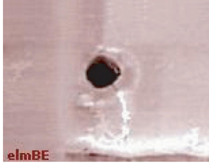
Figure 2.19: An ESD-induced oxide breakdown [9].
