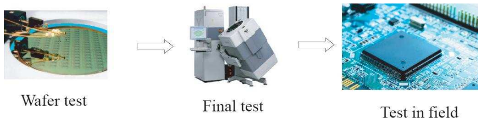
Figure 2.1: Different test steps of an IC.
