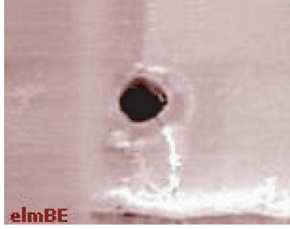
Figure 2.19: An ESD-induced oxide breakdown [9].
