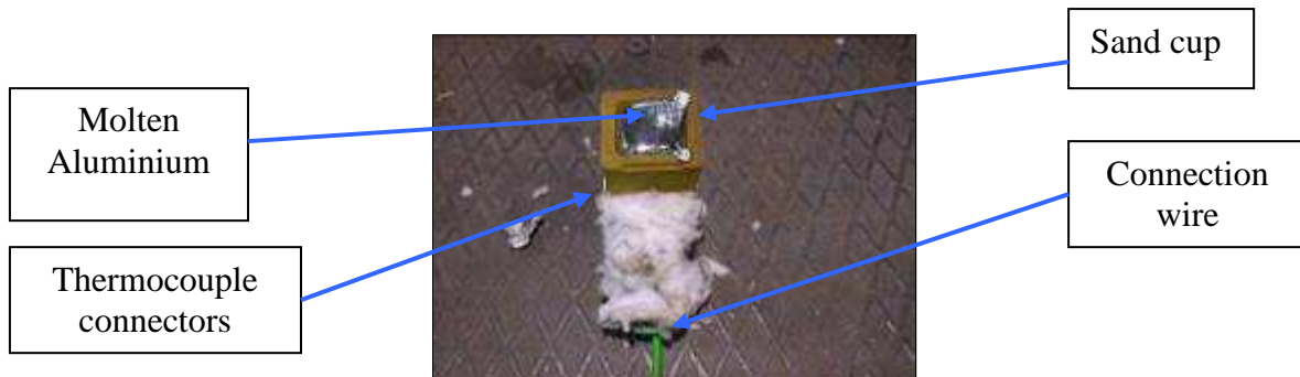
Figure 3.12.- Commercial sand cup for DTA determination
