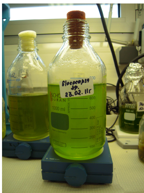
Fig. II. 10. Closed batch kinetic reactor used in the kinetic experiment with cyanobacteria Gloeocapsa sp.
