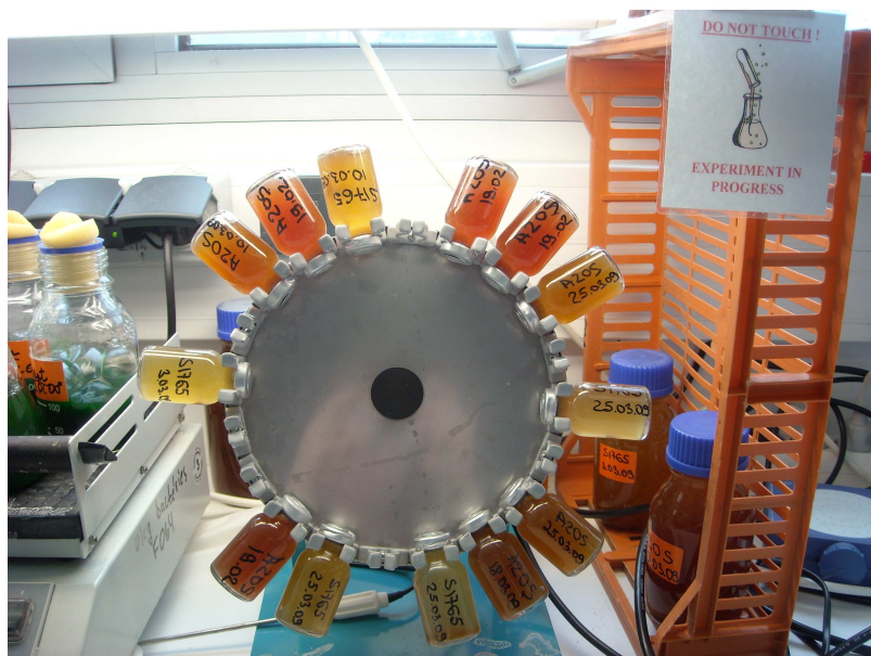
Fig. II. 9 . Rotator with the bottles in the kinetic experiment with APB A-20s and S-17-65.
