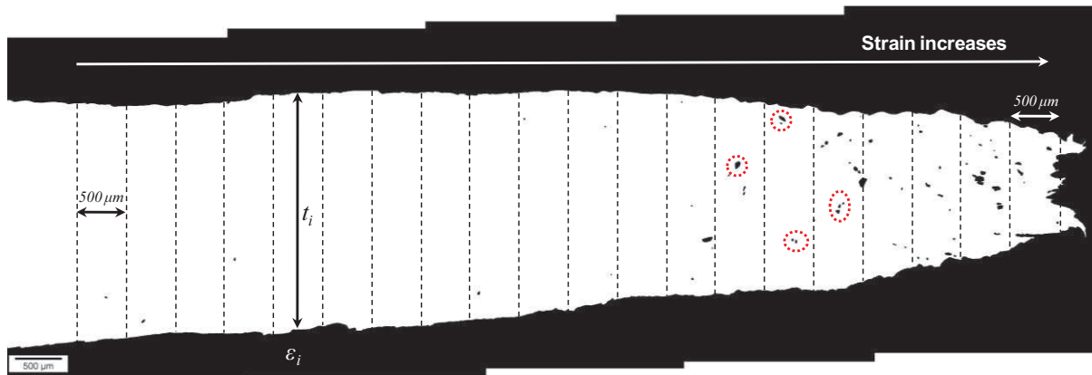
Figure III.8. Section perpendicular to the ligament in order to quantify the density of cracks per unit area ( \text{mm}^2 ) as a function of strain; the dotted lines correspond to the 500 \mu\text{m} -step partition; the black arrow shows the position where the thickness was measured to estimate the strain; and the red circled zones highlight a few voids.
