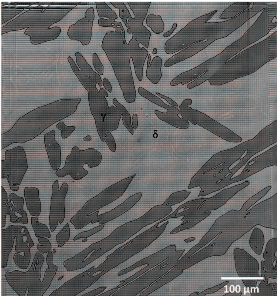
Figure C. 1. High resolution SEM micrograph of the D1_W microstructure (map1) in the undeformed configuration; sample iii. The compression will be applied vertically.
