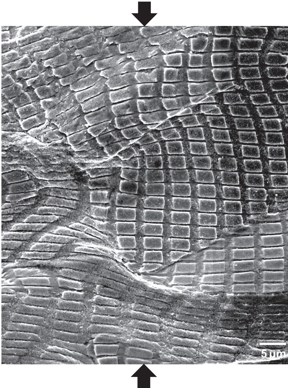
Figure C. 9. Small area from the deformed microgrid on sample III, D2_W microstructure, map1. The arrows indicate the loading direction.
