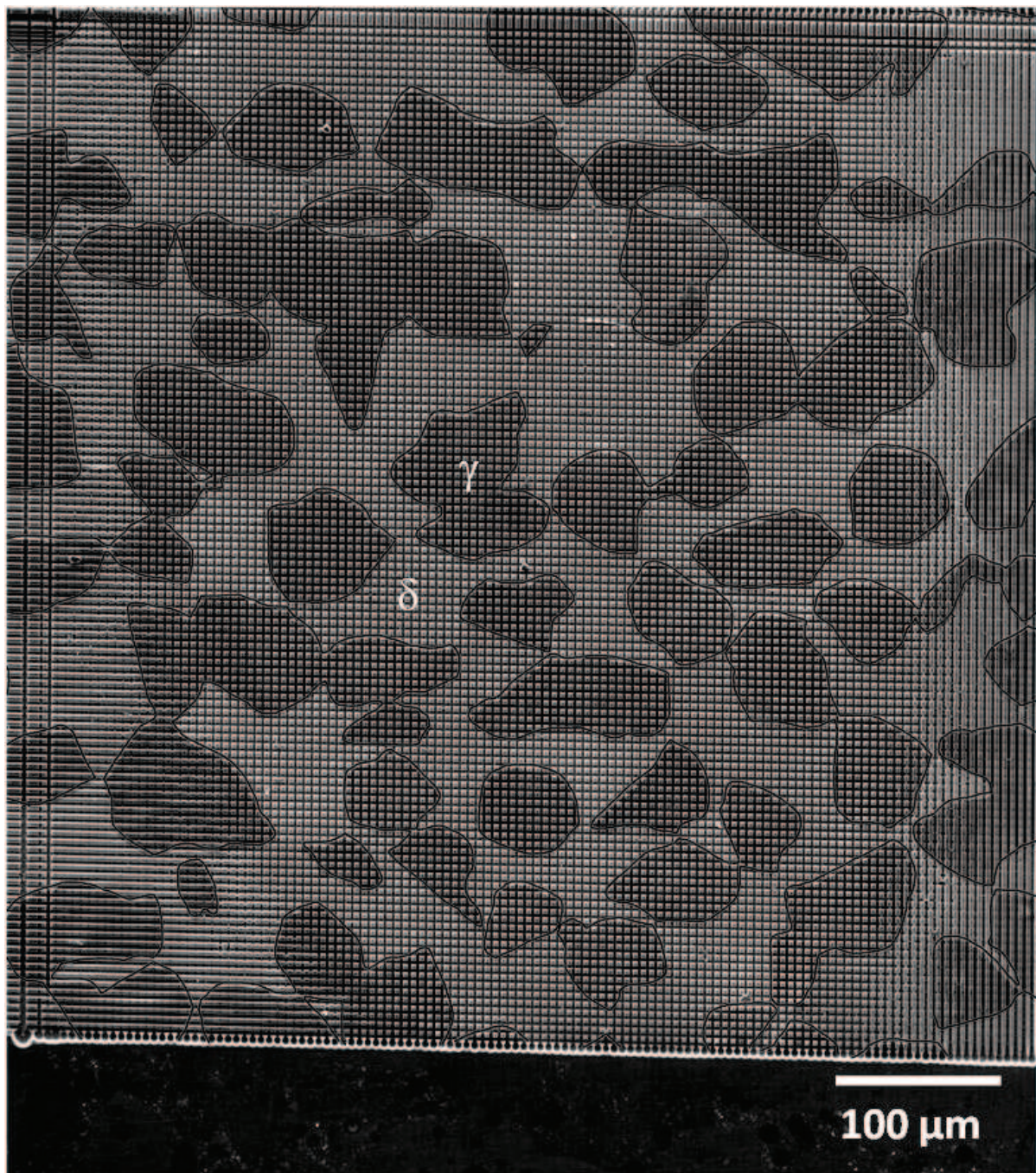
Figure C. 5. High resolution SEM micrograph of the D1_E microstructure in the undeformed configuration; sample B. The compression will be applied vertically.
