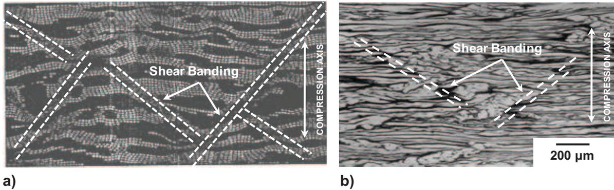
**Figure II.7.** Shear banding development in duplex stainless steel; a) deformed mesh obtained via finite element modeling after simulation of a specimen deformed at 1050°C under plane strain compression [16]; b) optical micrograph of a hot-rolled 2304 specimen (77% reduction) [9].
