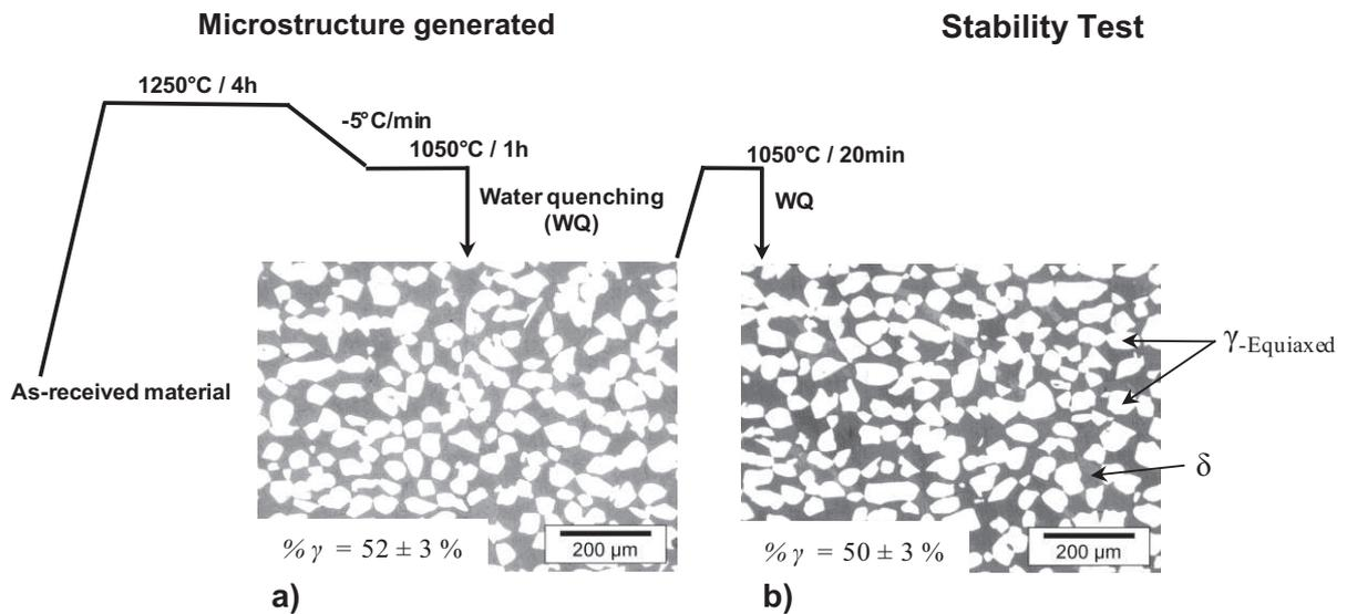
**Figure III.27.** Schematics of the HTE.2 applied to D2 and resulting microstructures; white =  $\gamma$ , grey =  $\delta$ ; a) HTE.2; b) Stability test of HTE.2.
