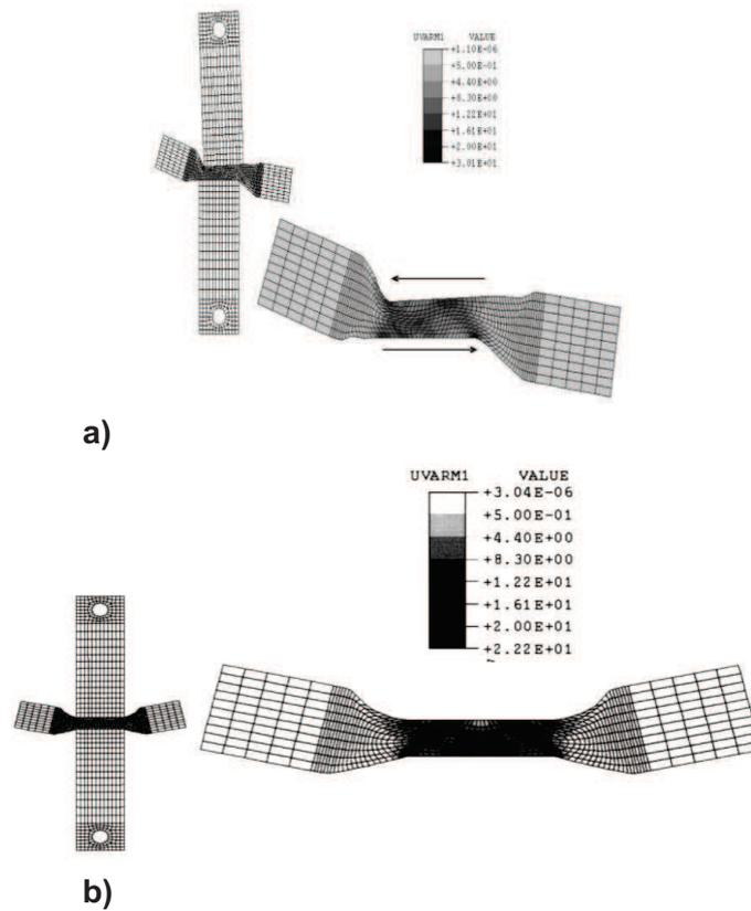
**Figure IV.12.** Possible problems encountered during plane strain compression; a) Z shape deformed specimen due to initial platen misalignment; b) U shape deformed specimen with different friction coefficients at the top and bottom tools [127].
