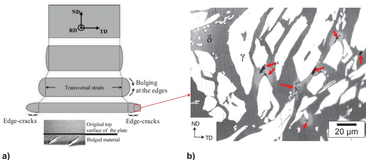
**Figure I.9.** a) Evolution of the transverse dimensions of the hot rolling blocks with increasing reduction; a clear transverse strain develops and cracks have been observed only in the bulged region; b) microstructure in the edge part illustrating the damage; red arrows emphasize the voids.
