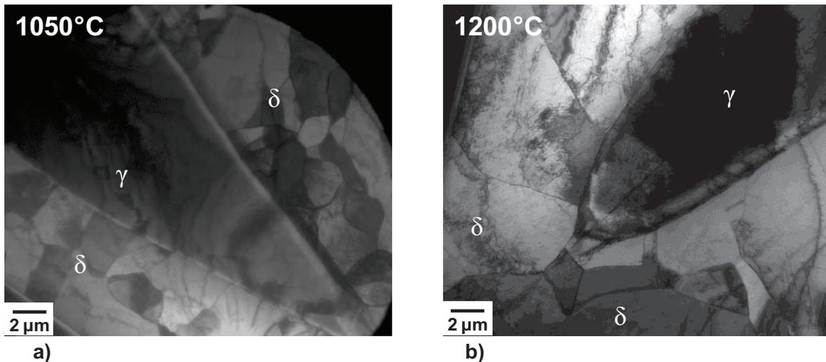
**Figure III.19.** TEM micrographs taken of the homogeneous zone of D2 broken DENT-specimens. A well-recovered microstructure in the ferrite with subgrains; and a high dislocation density with no sign of recrystallization in the austenite; a) T=1050°C; b) T=1200°C.
