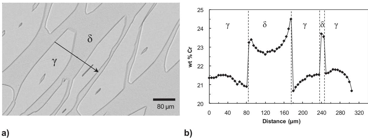
**Figure III.23.** Composition profile in wt% Cr from a D2 specimen obtained by WDS.
