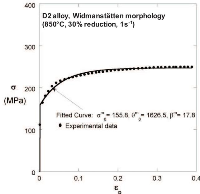
**Figure IV.48.** Macroscopic equivalent true stress-strain curve of D2 alloy presenting a Widmanstätten morphology measured during plane strain compression test at 850°C and 1s<sup>-1</sup>. Thick curve is the fit to Kocks-Mecking hardening law, see eq IV-12. The superscript 'm' means macroscopic.
