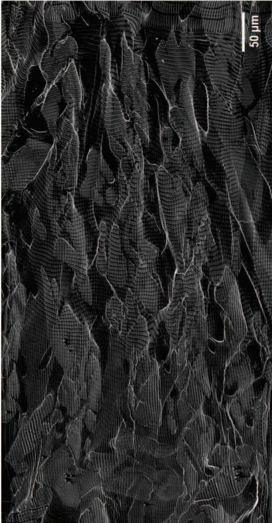
Figure C. 15. Microgrid of the D1\_W microstructure from sample iii after plane strain compression at 950°C.
