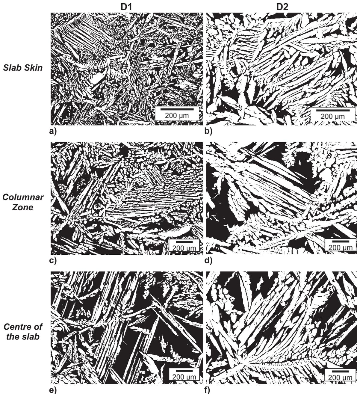
**Figure III.17.** Comparison between the as-cast slab of the alloys D1 and D2; a) & b) microstructures of the slab skin; c) & d) microstructures of the columnar zone; e) & f) microstructures at the centre of the slab. The austenite is in white and the ferrite in black.
