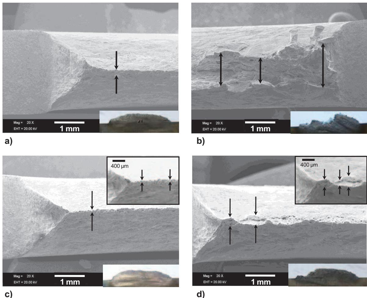
**Figure III.13.** Fracture micrographs and profiles of the broken DENT specimens ( $l_0 = 37\text{mm}$ ); a) D1 at 1050°C; b) D2 at 1050°C; c) D1 at 1200°C. d) D2 at 1200°C. The arrows emphasize the thickness variation in the profile.
