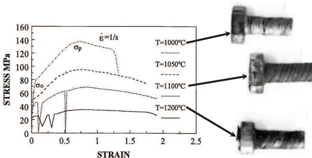
**Figure II.23.** Stress strain curves of a hot rolled 2304 grade deformed under torsion at different temperatures at  $1\text{s}^{-1}$  and the corresponding deformed specimens showing different levels of damage [25].
