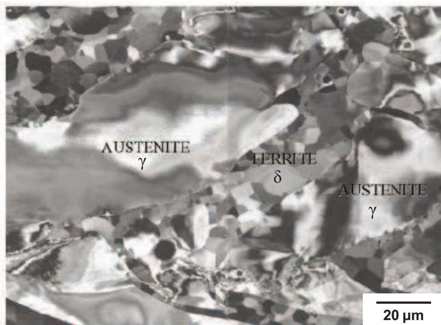
**Figure II.9.** SEM backscattered electron picture; as-cast 2304 duplex stainless steel deformed to 0.4 at 1000°C and 1s<sup>-1</sup> [9].
