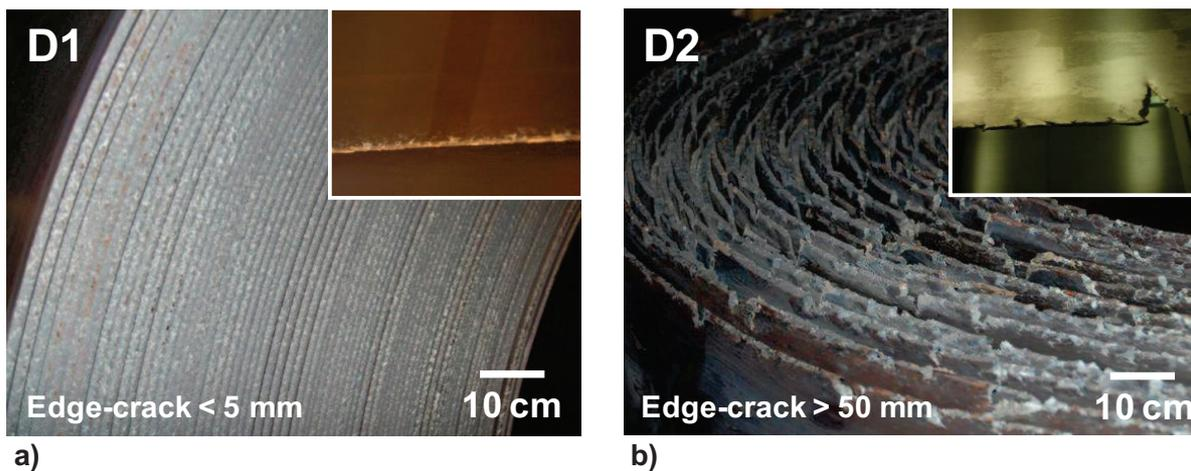
**Figure I.4.** Coils at the end of the hot rolling process showing different levels of edge-cracking depending on the grade; a) coil of the D1 grade with edge-cracks < 5mm; b) coil of the D2 grade with edge cracks > 50mm.
