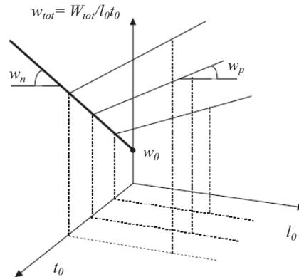
**Figure III.46.** Procedure followed to separate the three contributions to the total energy: the work of diffuse plasticity,  $w_p$  (per unit volume), the work of localized plasticity  $w_n$  (per unit volume), and the fracture work  $w_0$  (per unit surface) [76].
