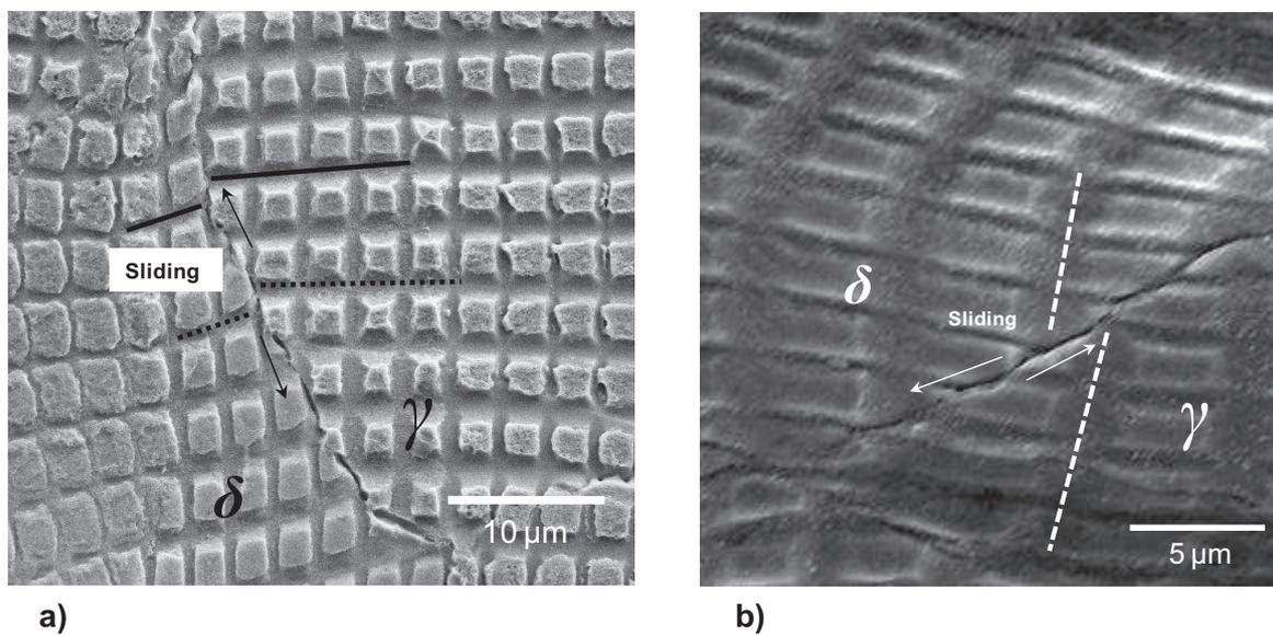
**Figure IV.42.** Illustration at different magnifications and different locations of the  $\delta/\gamma$  sliding mechanism occurring along the incoherent interface boundaries in the equiaxed microstructure.
