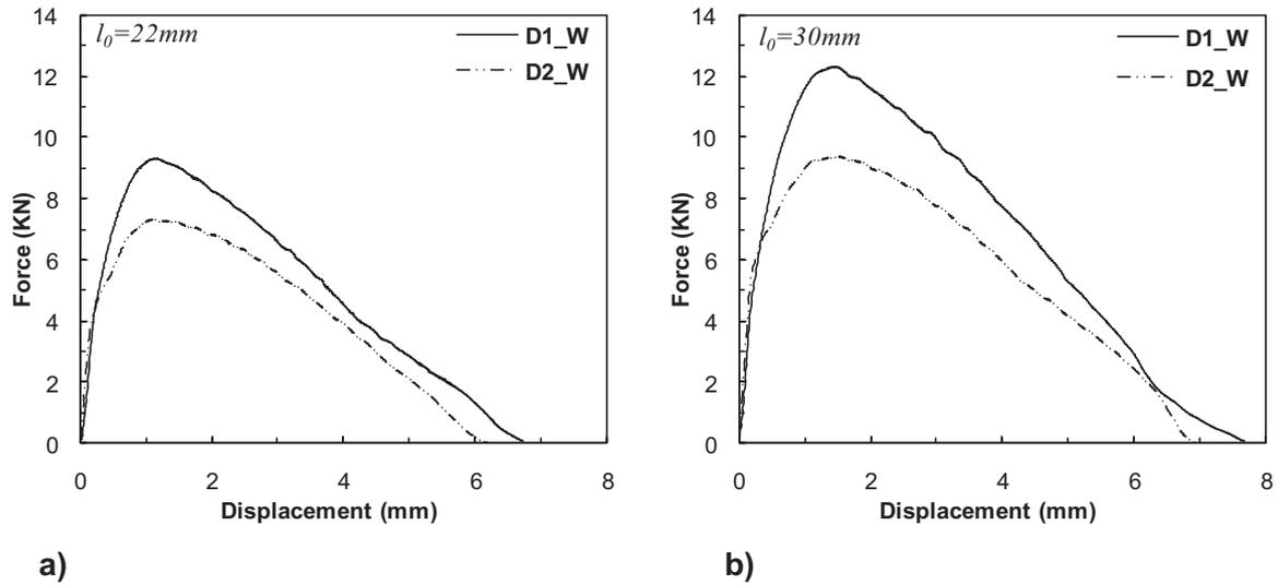
**Figure III.31.** Comparison between typical force-displacement curves of DENT specimens with the same ligament length  $l_0$  for both grades, D1\_W and D2\_W with a Widmanstätten microstructure; a)  $l_0 = 22\text{mm}$ ; b)  $l_0 = 30\text{mm}$ .
