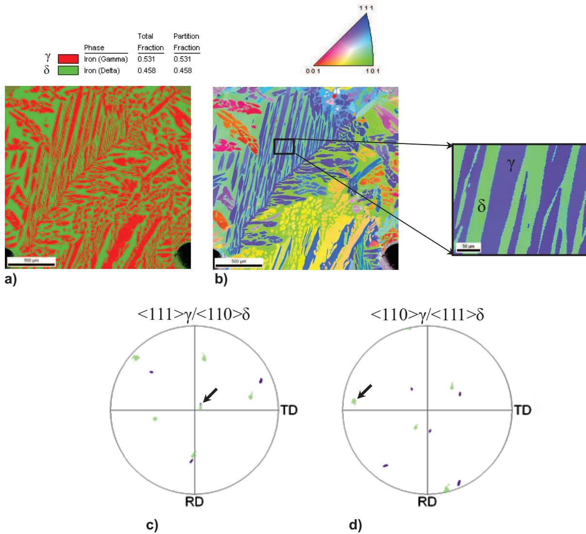
**Figure III.22.** EBSD analysis of the D2 as-cast microstructure; a) phase map; b) inverse Pole Figure orientation map; overlaying of c)  $\langle 111 \rangle_{\gamma}$  and  $\langle 110 \rangle_{\delta}$  and of d)  $\langle 110 \rangle_{\gamma}$   $\langle 111 \rangle_{\delta}$  poles figures, showing the existence of Kurdjumov-Sachs orientation relationship between  $\delta$  and  $\gamma$ .
