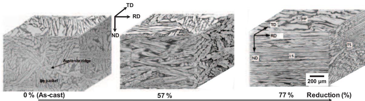
**Figure II.2.** Evolution in 3D of the as-cast microstructure with the applied rolling reduction of the duplex microstructure; as the deformation proceeds, austenite becomes more and more elongated in the rolling direction (RD) [11].
