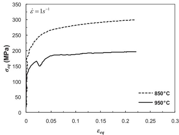
**Figure IV.36.** Comparison between the macroscopic equivalent stress strain curves of the equiaxed morphology obtained under plane strain compression at  $1\text{s}^{-1}$  and different temperatures:  $T = 850^\circ\text{C}$  and  $950^\circ\text{C}$  up to a reduction of 20%.
