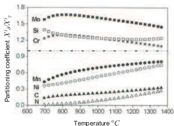
**Figure II.12.** The partitioning coefficient of the alloying elements between  $\delta$ -ferrite and  $\gamma$ -austenite as a function of temperature; the compositional changes will influence the strength and the deformation behaviour of the material [46].
