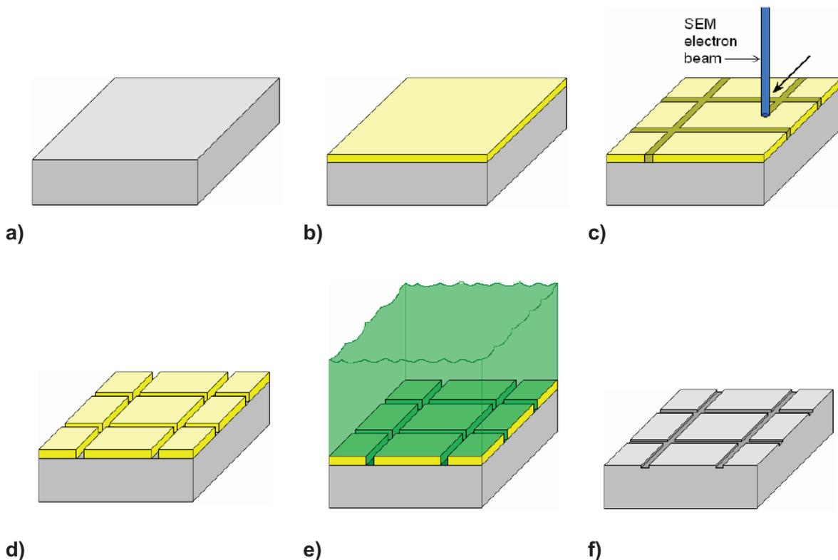
**Figure IV.7.** Steps of modified microgrid technique; a) polishing and electro-etching; b) coating with an electro-sensitive polymer; c) irradiation of the resin with the electron beam; d) dissolution of the irradiated polymer; e) engraving by electro-etching; f) dissolution of the remaining polymer [50].
