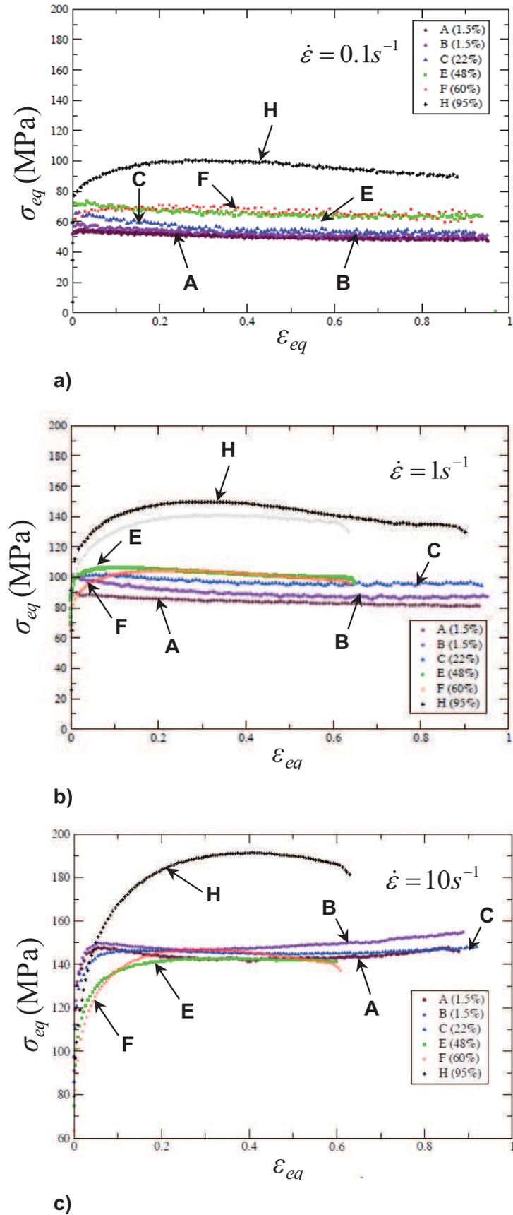
**Figure II.11.** Equivalent flow stress strain curves of different duplex stainless steels deformed under plane strain compression at 1050°C and at different strain rates; a)  $0.1s^{-1}$ ; b)  $1s^{-1}$ ;  $10s^{-1}$ . The value between the parenthesis gives the austenite content [42].
