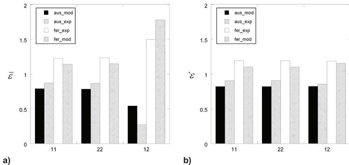
**Figure IV.51.** Comparison of experimental (denoted as *exp*) and finite element predictions (denoted as *mod*); a) average strain per phase; b) dispersion for strain components 11, 22 and 12. The strains and dispersions are expressed relative to the respective totals in the map. *aus* stands for austenite, and *fer* stands for ferrite.
