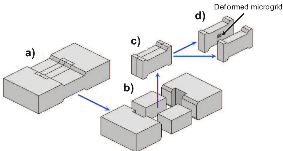
**Figure IV.19.** Schematic extraction of microgrid from deformed plane strain compression sample; a) deformed plane strain compression specimen; b) specimen cut in five pieces; c) inserts; d) separation of the two inserts, one of them being the microgrid sample.
