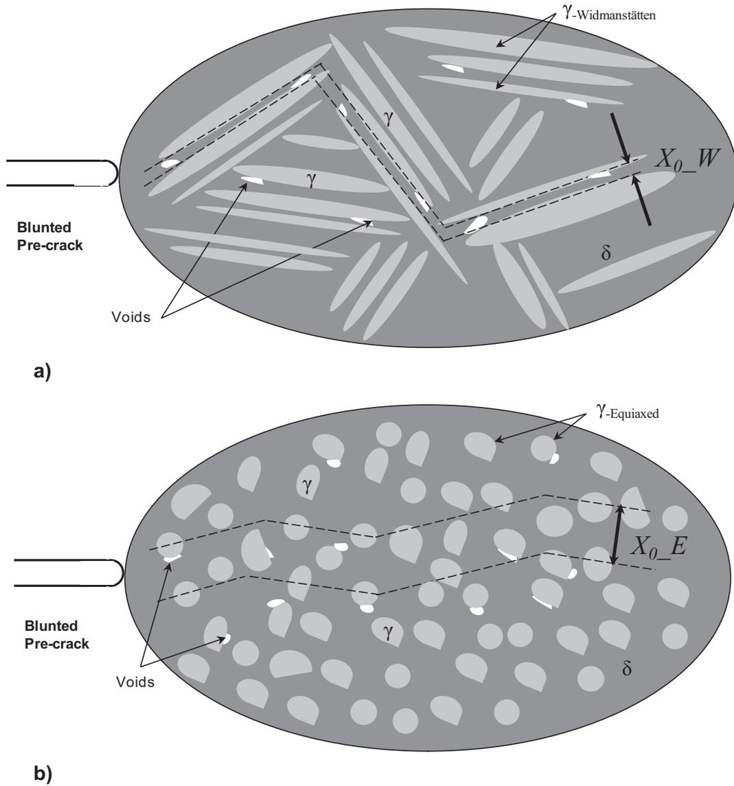
**Figure III.45.** Schematic definition of the characteristic length  $X_0$  for each morphology: a) equiaxed morphology, and b) Widmanstätten morphology.
