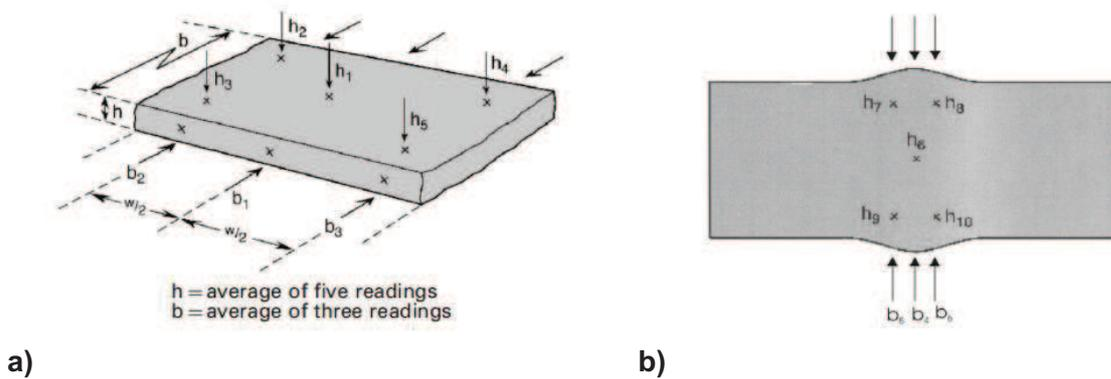
**Figure A. 1.** Schematic diagram of a testpiece; a) before and b) after testing, and approximate dimensional measurement positions.
