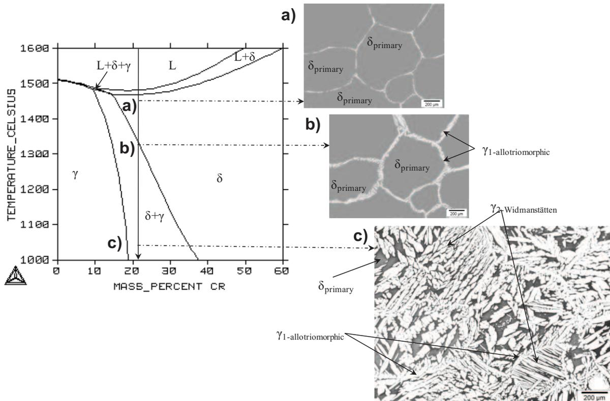
**Figure I.5.** Origin of the as-cast microstructure in duplex stainless steel; a) at high temperature duplex stainless steel is entirely ferritic; during cooling, the austenite precipitates b) at existing ferrite grain boundaries and c) inside the ferrite matrix with a lath morphology; thermal history explains the as-cast microstructure.
