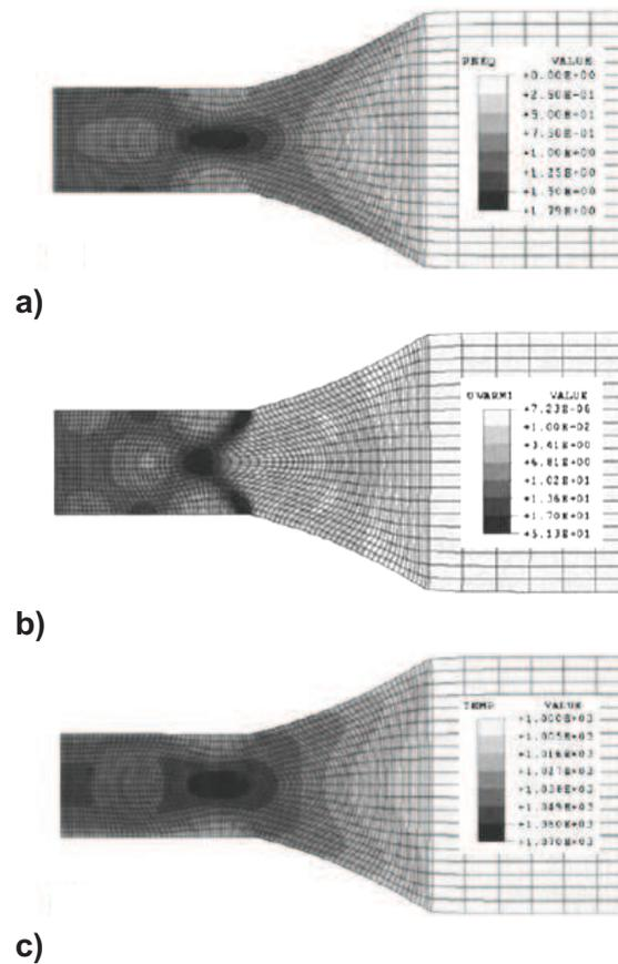
**Figure IV.33.** Finite elements predictions of given parameters at nominal equivalent strain of 1 for frictionless deformation of a 316L-austenitic stainless steel specimen with  $h_0 = 10$  mm,  $\dot{\epsilon} = 10\text{s}^{-1}$  and  $T=1000^\circ\text{C}$ ; a) equivalent strain; b) equivalent strain rate; c) temperature distributions [130].
