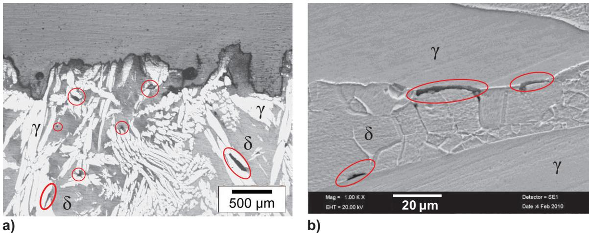
**Figure III.15.** a) Optical micrograph and b) SEM micrograph of a region close to the fracture of a DENT specimen deformed at 1050°C. Voids nucleate by a partial decohesion of the  $\delta/\gamma$  interface, see circled red areas.
