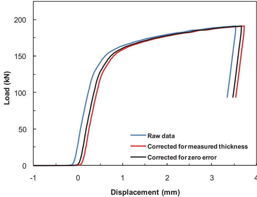
Figure A.2. Origin corrections, taken from a single deformation carried out at 850°C and 1s<sup>-1</sup>.
