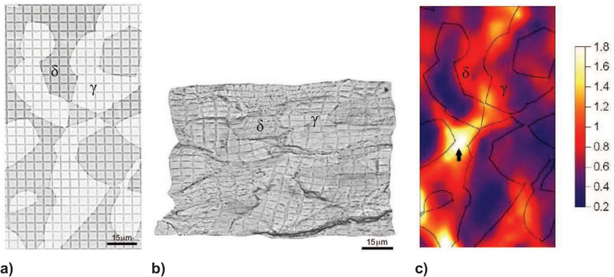
**Figure II.14.** Highlighting of strain partitioning via the microgrid technique in a laboratory 29.6%Cr-11.6%Ni-0.27%Mn duplex steel deformed at 950°C and 1s<sup>-1</sup>; a) undeformed state of a relatively small area; b) deformed configuration of the same area; c) distribution of the Green-Lagrange equivalent Von Mises strain [19].
