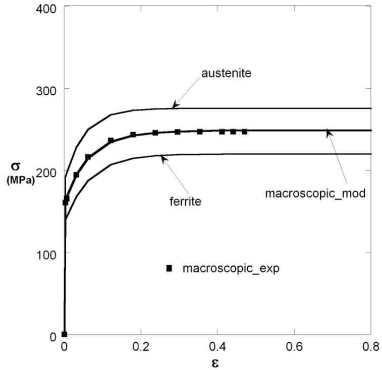
**Figure IV.52.** Flow curves for the macroscopic material and the two phases. The measured data is indicated by solid squares. The simulated macroscopic stress-strain curve is rather well in agreement with the experimental one.
