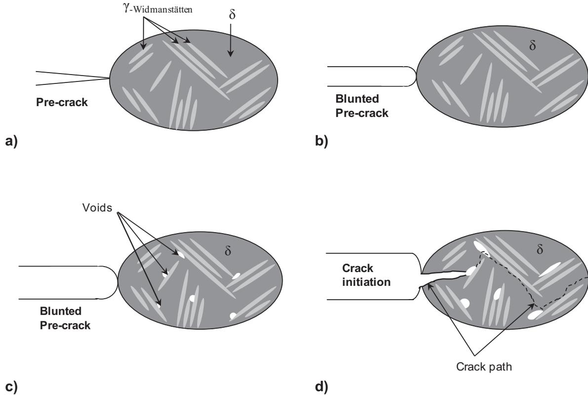
**Figure III.14.** Schematic illustration of the damage and fracture process taking place in the fracture process zone of duplex stainless steels ; a) initial state ; b) onset of the crack tip blunting ; c) damage nucleation ; d) void coalescence and crack initiation.
