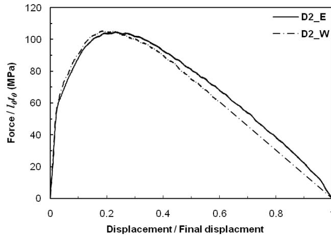
**Figure III.47.** Normalization of the force displacement curves for a ligament length of  $l_0 = 22\text{mm}$  for respectively, the D2\_E and D2\_W microstructures. The force is normalized by the area of the ligament that gives a stress and the displacement is divided by the final displacement.
