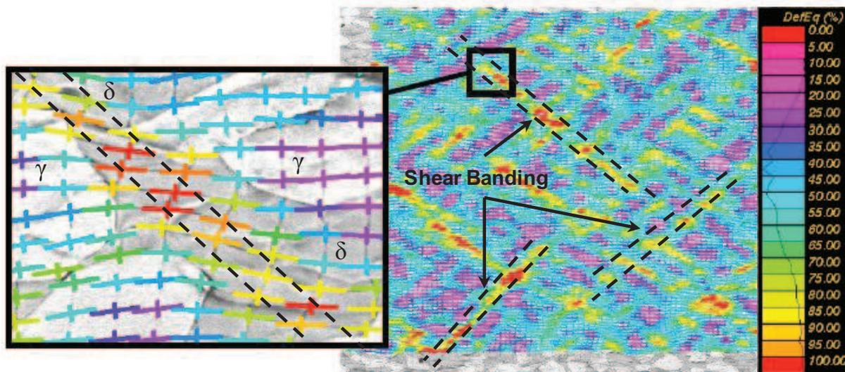
**Figure II.8.** Map of the Von Mises equivalent strain superimposed with the deformed microstructure revealing the development of localization bands under plane strain compression at 850°C and  $1s^{-1}$  of a 29%Cr-11%Ni duplex stainless steel [17].
