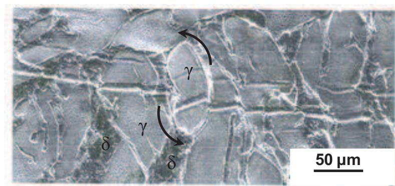
**Figure II.6.** SEM picture showing the rotation of an austenite grain highlighted by the displacement of the scratch markers at the specimen surface; as-cast 2304 duplex stainless steel deformed under torsion to 1.6 at 1000°C and 1s<sup>-1</sup> [13].
