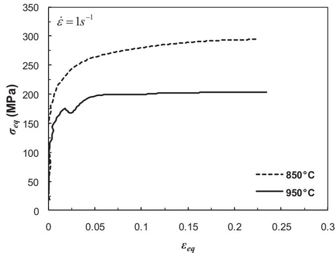
**Figure IV.39.** Comparison between the macroscopic equivalent stress strain curves of the Widmanstätten morphology obtained under plane strain compression at  $1\text{s}^{-1}$  and different temperatures:  $T = 850^\circ\text{C}$  and  $950^\circ\text{C}$  up to a reduction of 20%.
