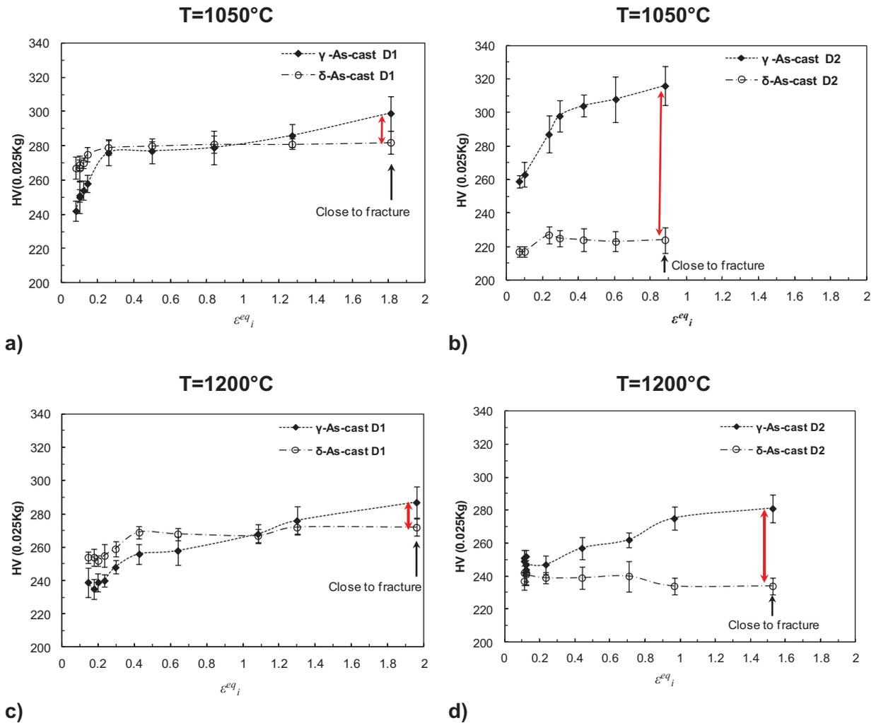
**Figure III.18.** Micro-hardness profiles along the homogeneous zone of DENT specimens in both phases; a) alloy D1, T=1050°C; b) alloy D2, T=1050°C; c) D1, T=1200°C; d) D2, T=1200°C. It is considered that there was no significant gradient of temperature along the region where the hardness tests were performed.
