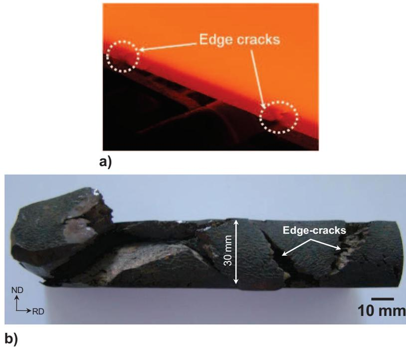
**Figure I.3.** Illustration of the poor hot workability of duplex stainless steels; a) occurrence of the first edge-cracks during the roughing mill operations; b) example of edge cracks after the roughing-mill operations.
