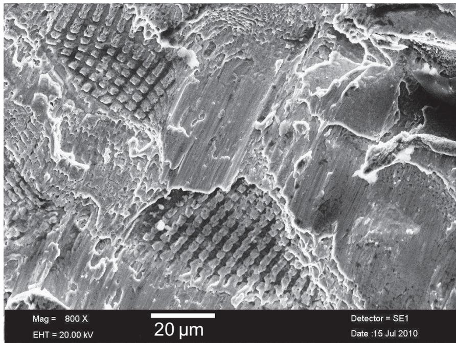
**Figure IV.45.** SEM micrograph showing the deformed microgrids after plane strain compression at 1050°C and 10s<sup>-1</sup>.
