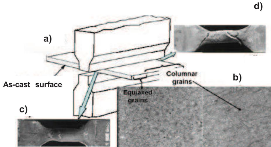
**Figure II.22.** Plane strain compression at  $1000^{\circ}\text{C}$  and  $1\text{s}^{-1}$  in order to test the effect of the macrostructure on the crack formation; a) schematic view showing the position of the specimen on the machine; b) view of the as-cast microstructure seen on the transverse section of the specimen; c) level of defect on the equiaxed grain side; d) level of defect on the columnar grain side [20].
