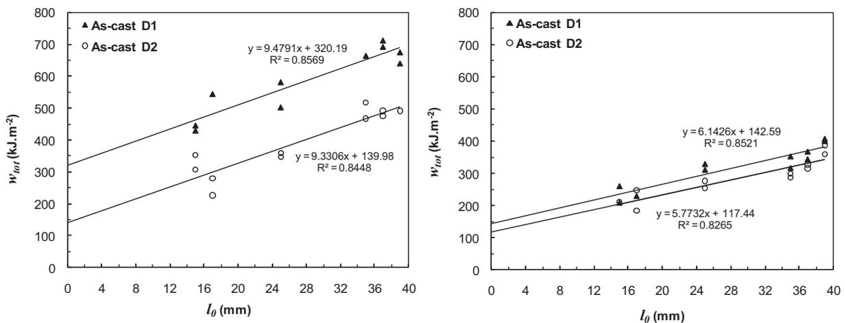
**Figure III.12.** Variation of the total specific work of fracture as a function of the ligament length for separation of the essential work of fracture; comparison between the two grades D1 and D2 in the as-cast conditions; a)  $T=1050^{\circ}\text{C}$ ; b)  $T=1200^{\circ}\text{C}$ .
