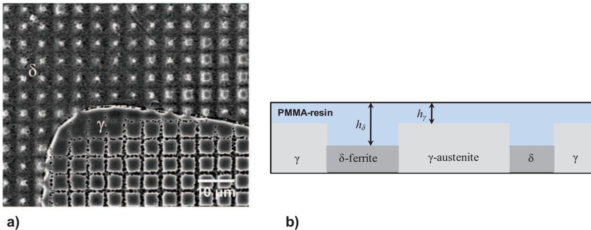
**Figure IV.9.** a) Microgrids before deformation (notice that the lines are more visible in the austenite); b) difference in terms of heights between austenite (light grey) and ferrite (dark grey) on the surface due to etching of ferrite.
