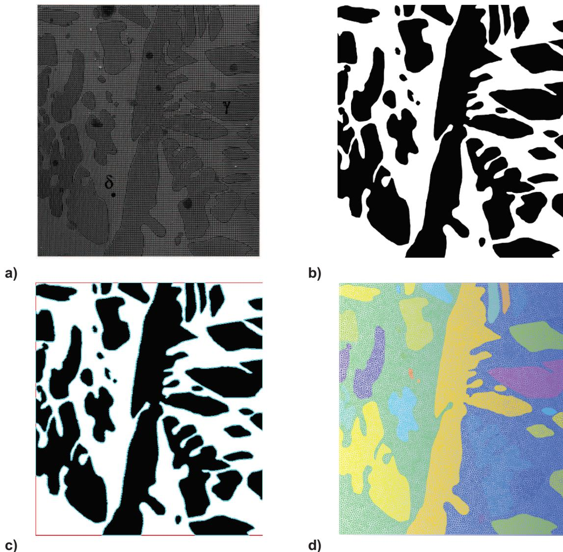
**Figure IV.47.** Illustration of the microstructure modelling using sample D2\_W, map2; a) SEM micrograph of undeformed sample; b) micrograph after image processing in MATLAB [136] (black = austenite, white = ferrite); c) geometric profile (green boundary lines computed by image analysis algorithm); d) FE mesh, as discretized by GSMH [137].
