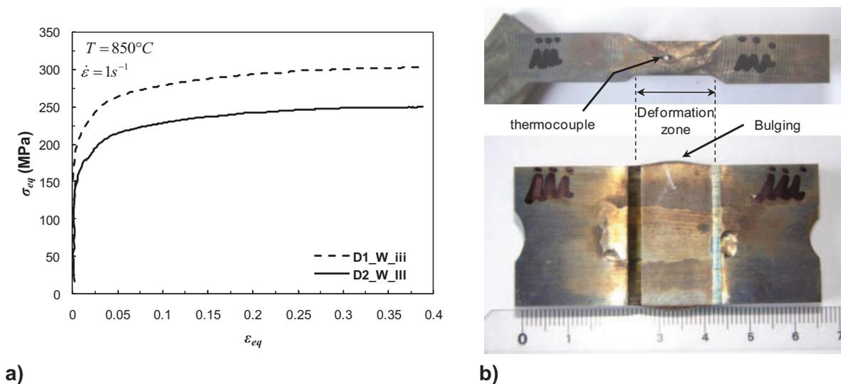
**Figure IV.22.** a) Comparison between the macroscopic stress strain curves of the D1\_W and D2\_W microstructures obtained under plane strain compression at 850°C and 1s<sup>-1</sup> up to a reduction of 30%; b) pictures showing a top view and a front view of a deformed plane strain compression specimen.
