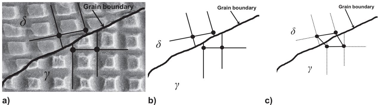
**Figure IV.43.** a) SEM micrograph and b) schematic of sliding at a  $\delta/\gamma$  interphase boundary; and c) shear deformation as interpreted by the strain calculation method, which only takes into account the four corners of each microgrid square.
