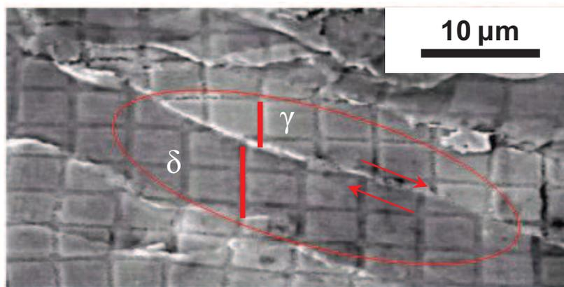
**Figure II.4.** A clear example of interphase boundary sliding in a 2205 duplex stainless steel deformed to 0.15 at 1050°C and 1s<sup>-1</sup> [14].
