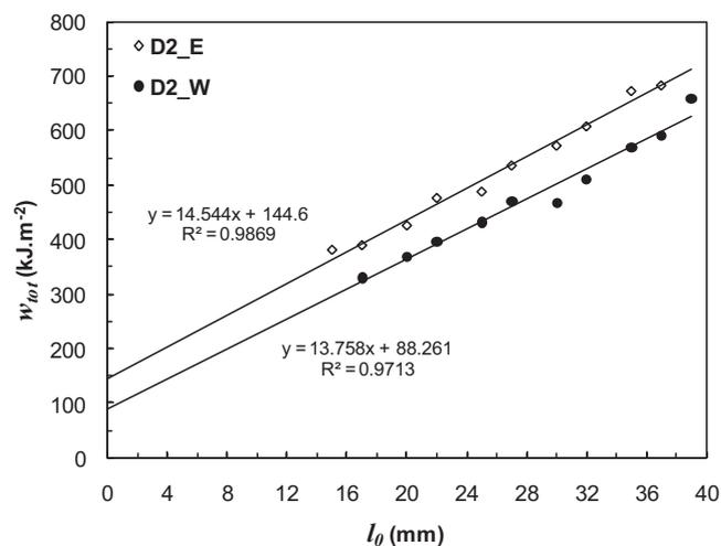
**Figure III.40.** Variation of the specific work of fracture as a function of the ligament length for separation of the essential work of fracture. Comparison between the two microstructures at  $1050^\circ\text{C}$ : D2\_E and D2\_W.
