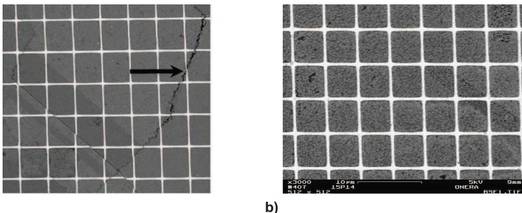
**Figure IV.4.** a) Illustration of the grain boundary sliding after creep at  $750^\circ\text{C}$  in nickel-based super alloy thanks to  $\text{HfO}_2$  microgrids (step of  $5\mu\text{m}$ ); b)  $\text{HfO}_2$  grid after 1000h at  $750^\circ\text{C}$  under vacuum (SEM, Back-scattered electron mode) [103].
