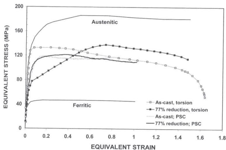
**Figure II.16.** Effect on the equivalent stress strain curves of the deformation mode for a 2304 duplex stainless steel deformed at  $1000^{\circ}\text{C}$  and  $1\text{s}^{-1}$  under torsion and plane strain compression [25].
