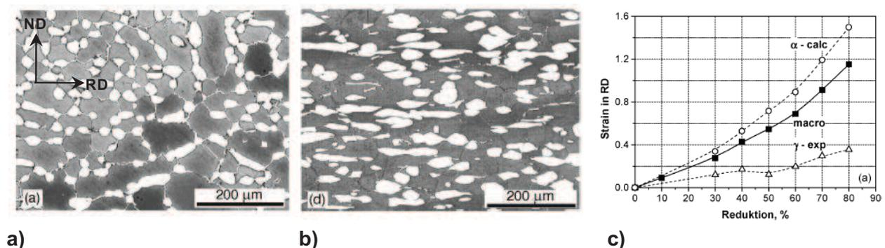
**Figure II.13.** Microstructure evolution during hot rolling at 1250°C for reduction a) 0% and b) 80%. Initially austenite equiaxed islands are embedded in a ferrite matrix. During hot rolling, these islands become more elongated in the rolling direction. c) Strain partitioning in the rolling direction, austenite seems to accommodate only a fraction of the applied strain [48].
