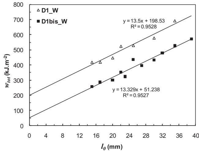
**Figure III.49.** Variation of the specific work of fracture as a function of the ligament length for separation of the essential work of fracture. Comparison between D1\_W and D1bis\_W microstructures at 1050°C.
