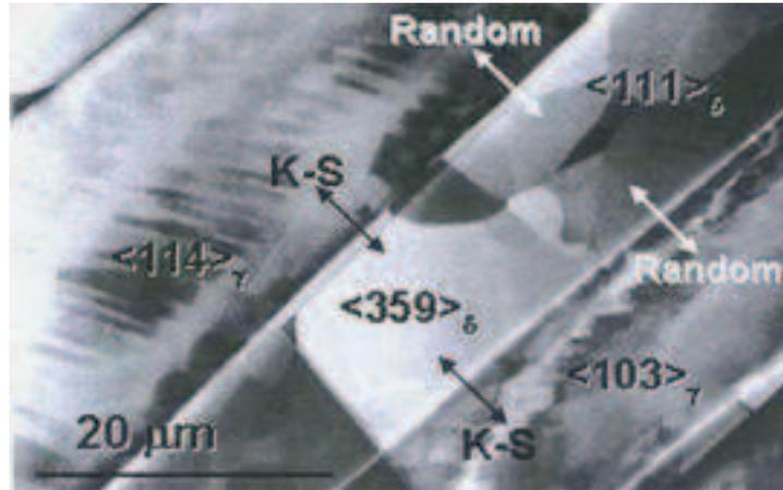
**Figure II.10.** STEM channeling picture and crystallographic orientation analysis; as-cast duplex stainless steel deformed to 1.6 at 1000°C and 1s<sup>-1</sup> [5].
