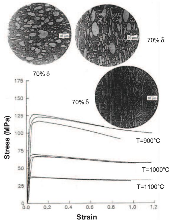
**Figure II.17.** Influence of the phase morphology on the flow stress of duplex stainless steel with 70%  $\delta$  deformed under uniaxial compression at different temperature at a strain rate of  $0.03\text{s}^{-1}$  [51].
