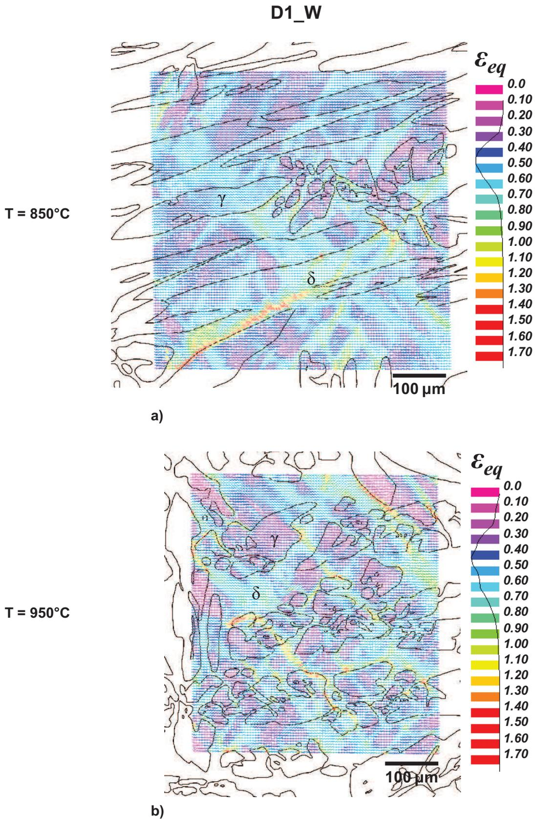
**Figure IV.40.** Equivalent strain distribution maps of the Widmanstätten morphology: D1\_W at T = 850 and 950°C; a) strain map at T = 850°C; b) strain map at T = 950°C. The equivalent strain map is superimposed with the undeformed microstructure to clearly present where in the microstructure the strains are distributed. The loading direction corresponds to the vertical axis.
