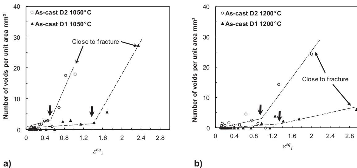
**Figure III.16.** Evolution of the damage as a function of strain for both grades in the as-cast conditions; a)  $T = 1050^\circ\text{C}$ ; b)  $T = 1200^\circ\text{C}$ . The arrow indicates the strain at which damage starts increasing significantly, i.e. the approximate strain at which damage nucleation occurs.
