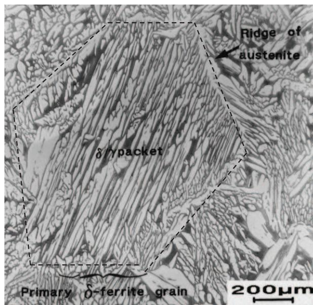
**Figure II.1.** As-cast microstructure in a conventional 2304 duplex stainless steel; the dotted lines indicate the primary  $\delta$ -ferrite grain, allotriomorphic austenite decorates the primary  $\delta$ -ferrite grain boundaries and Widmanstätten austenite appears inside the primary  $\delta$ -ferrite grain [12].
