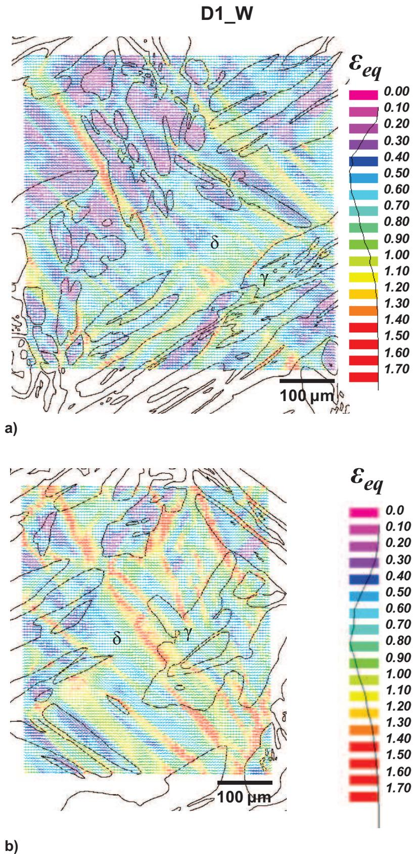
**Figure IV.23.** Equivalent strain distribution maps of the D1\_W microstructure; a) map 1; b) map 2; the equivalent strain map is superimposed with the undeformed microstructure to clearly present where in the microstructure the strains are distributed; the compression axis corresponds to the vertical axis.
