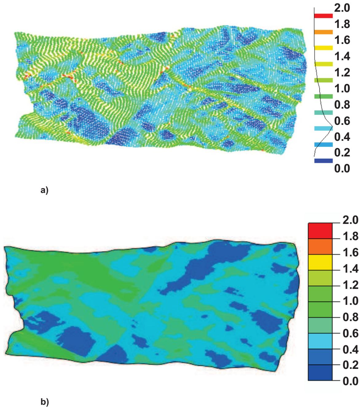
**Figure IV.49.** Equivalent strain distribution; a) experimental; b) computed by FE model for the best solution. The displacement profile on the edges is in good agreement with the experimental. Clearly, the strain localization is more in ferrite than in austenite. The compression is applied vertically.
