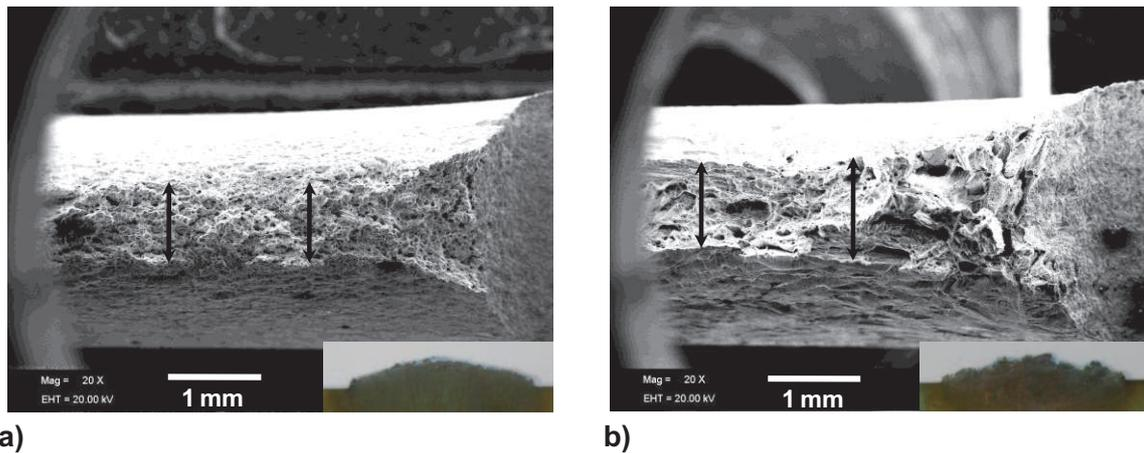
**Figure III.41.** Fracture micrographs and profiles of the broken DENT at 1050°C; a) D2\_E ( $l_0=35$ mm); b) D2\_W ( $l_0=37$ mm).
