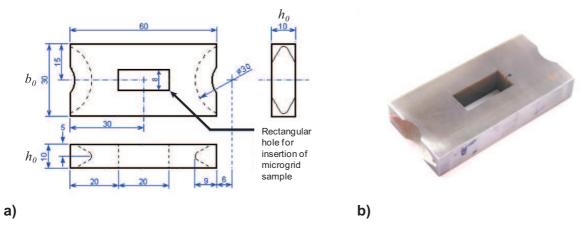
**Figure IV.13.** a) Technical drawing of the modified plane strain compression specimen, dimensions are in millimeters (mm); b) picture of a modified plane strain compression specimen.
