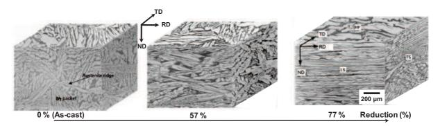
**Figure II.2.** Evolution in 3D of the as-cast microstructure with the applied rolling reduction of the duplex microstructure; as the deformation proceeds, austenite becomes more and more elongated in the rolling direction (RD) [11].
