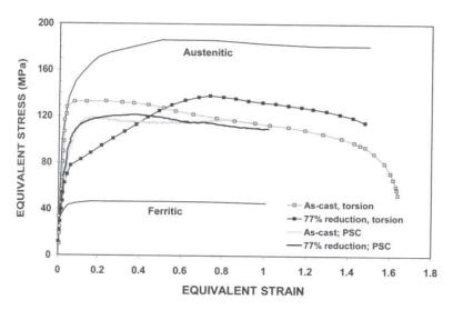
**Figure II.16.** Effect on the equivalent stress strain curves of the deformation mode for a 2304 duplex stainless steel deformed at 1000°C and 1s<sup>-1</sup> under torsion and plane strain compression [25].
