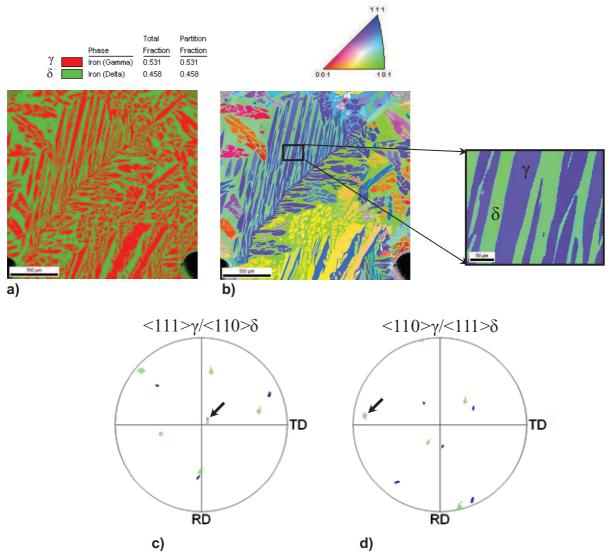
**Figure III.22.** EBSD analysis of the D2 as-cast microstructure; a) phase map; b) inverse Pole Figure orientation map; overlaying of c) <111> $\gamma$  and <110> $\delta$  and of d) <110> $\gamma$  <111> $\delta$  poles figures, showing the existence of Kurdjumov-Sachs orientation relationship between  $\delta$  and  $\gamma$ .
