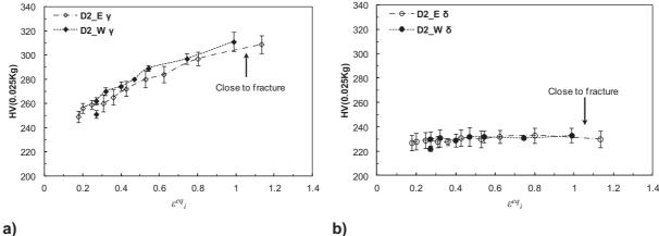
**Figure III.43.** Comparison between the micro-hardness profiles along the homogeneous zone of DENT specimens in both morphologies: D2\_E and D2\_W; a) Profile in the austenite, T=1050°C; b) Profile in the ferrite, T=1050°C.
