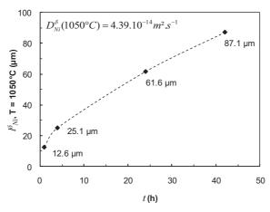
Figure III.28. Evolution of the Ni-diffusion length in the ferrite as a function of time at T = 1050°C.
