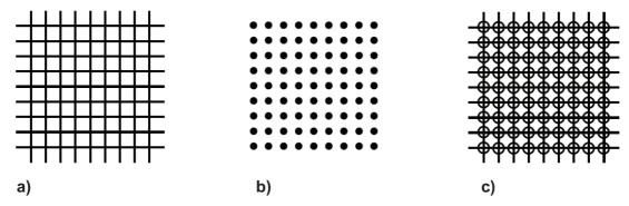
**Figure IV.1.** Illustration of different grid patterns; a) fiducial microgrids; b) fine array of dots; and c) fine array of lines encircled.
