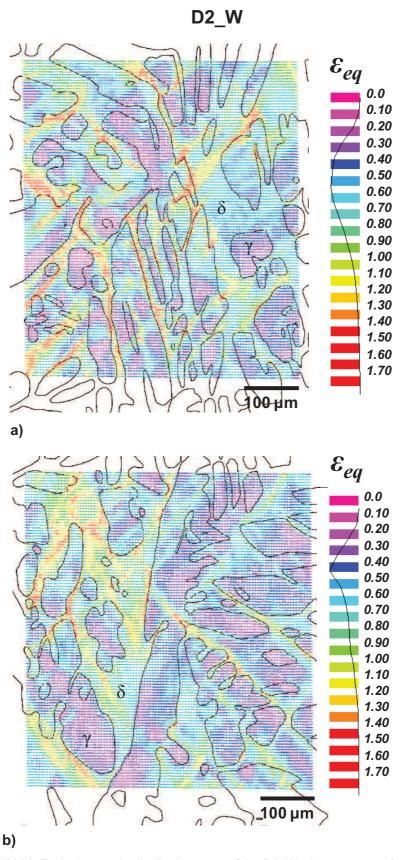
**Figure IV.24.** Equivalent strain distribution maps of the D2\_W microstructure; a) map 1; b) map 2; the equivalent strain map is superimposed with the undeformed microstructure to clearly present where in the microstructure the strains are distributed; the compression axis corresponds to the vertical axis.
