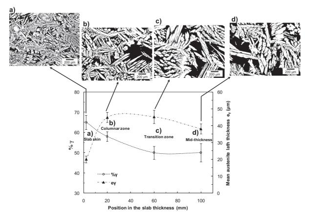
**Figure III.20.** Illustration of the alloy D2 as-cast slab heterogeneity through thickness; a) slab skin; b) columnar zone; c) transition zone; d) centre of the slab. The austenite is in white and the ferrite is in black.
