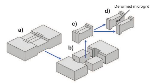
**Figure IV.19.** Schematic extraction of microgrid from deformed plane strain compression sample; a) deformed plane strain compression specimen; b) specimen cut in five pieces; c) inserts; d) separation of the two inserts, one of them being the microgrid sample.
