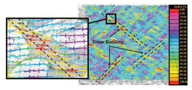
**Figure II.8.** Map of the Von Mises equivalent strain superimposed with the deformed microstructure revealing the development of localization bands under plane strain compression at 850°C and 1s<sup>-1</sup> of a 29%Cr-11%Ni duplex stainless steel [17].
