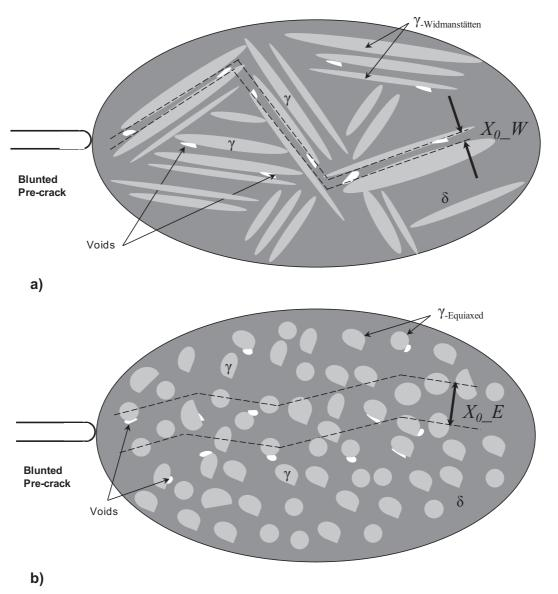
**Figure III.45.** Schematic definition of the characteristic length  $X_{\theta}$  for each morphology: a) equiaxed morphology, and b) Widmanstätten morphology.
