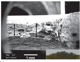
**b) Figure III.33.** Fracture micrographs of the broken DENT at 1050°C; a) D1\_W ( $l_0$ =35mm); b) D2\_W
