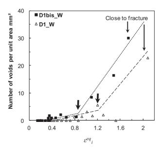
**Figure III.51.** Evolution of the damage as a function of equivalent strain for both D1\_W and D1bis\_W microstructures. The arrows indicate the approximate strain at which damage nucleation occurs.
