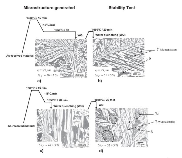
**Figure III.24.** Schematics of the HTW applied to D2 and resulting microstructures; white =  $\gamma$ , grey =  $\delta$ ; a) HTW.1; b) stability test of HTW.1; c) HTW.2; d) stability test of HTW.2. The encircled zones indicate the precipitation of the secondary fine austenite.
