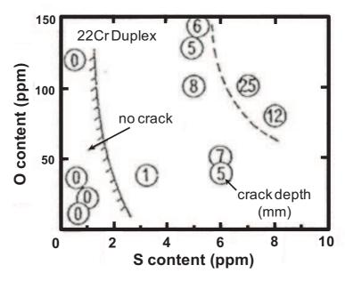
**Figure II.21.** Effect of S and O contents on the crack length of a 2205 hot-rolled duplex stainless steels (85% reduction) [63].
