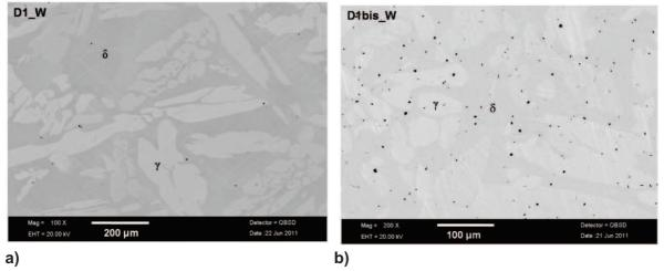
**Figure III.53.** SEM micrograph to illustrate the difference in terms of inclusion content between a) D1\_W and b) D1bis\_W. Austenite is the brightest phase, ferrite is the dark phase and the inclusions are in black due to a significant difference in terms of chemical composition.
