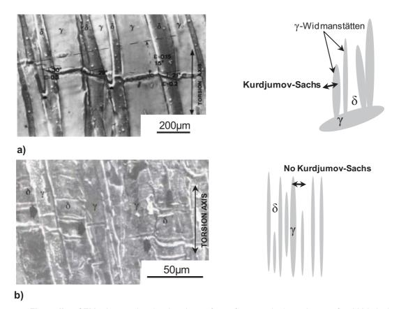
**Figure II.5.** SEM micrographs showing the surface of two marked specimens of a 2304 duplex stainless steel deformed to 0.17 under torsion at 1000°C and 1s<sup>-1</sup>; a) in the as-cast condition,  $\delta$  is related to  $\gamma$  by a Kurdjumov-Sachs orientation relationship; b) in the hot-rolled condition (reduction 77%), no lattice correspondence between  $\delta$  and  $\gamma$  [12].
