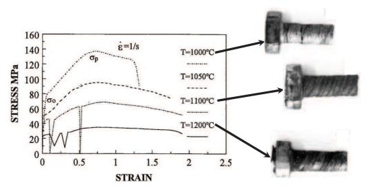
**Figure II.23.** Stress strain curves of a hot rolled 2304 grade deformed under torsion at different temperatures at 1s<sup>-1</sup> and the corresponding deformed specimens showing different levels of damage [25].
