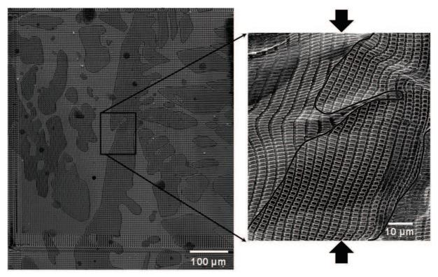
**Figure C. 12.** Undeformed state of the map2 of the D2\_W microstructure and zoom of a part of the corresponding deformed microgrid. The arrows indicate the loading direction.
