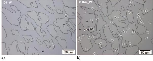
**Figure III.54.** Optical micrograph to illustrate the difference in terms of inclusion content between a) D1\_W and b) D1bis\_W. The inclusions are circled in white and the interfaces between ferrite and austenite are highlighted to determine the location of the particles.
