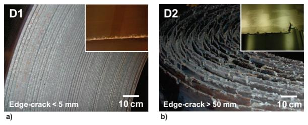
**Figure I.4.** Coils at the end of the hot rolling process showing different levels of edge-cracking depending on the grade; a) coil of the D1 grade with edge-cracks < 5mm; b) coil of the D2 grade with edge cracks > 50mm.
