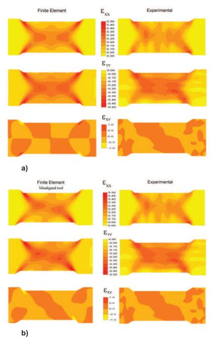
**Figure IV.35.** Numerical (left) and experimental (right) contour plots of the components of the logarithmic plastic strain; a) numerical values were obtained assuming perfect alignment between tools; b) results obtained considering a misalignment of 1mm between tools [125].
