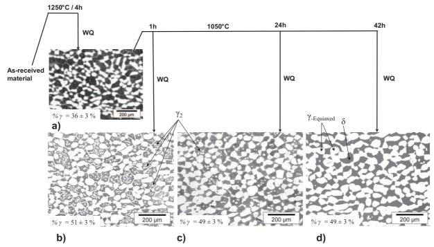
**Figure III.26.** Schematics of the HTE.1 applied to D2 and resulting microstructures; white =  $\gamma$ , grey =  $\delta$ ; a) 1250°C/4h + WQ; b) 1250°C/4h + WQ + 1050°C/1h + WQ; c) 1250°C/4h + WQ + 1050°C/24h + WQ; d) 1250°C/4h + WQ + 1050°C/42h + WQ.
