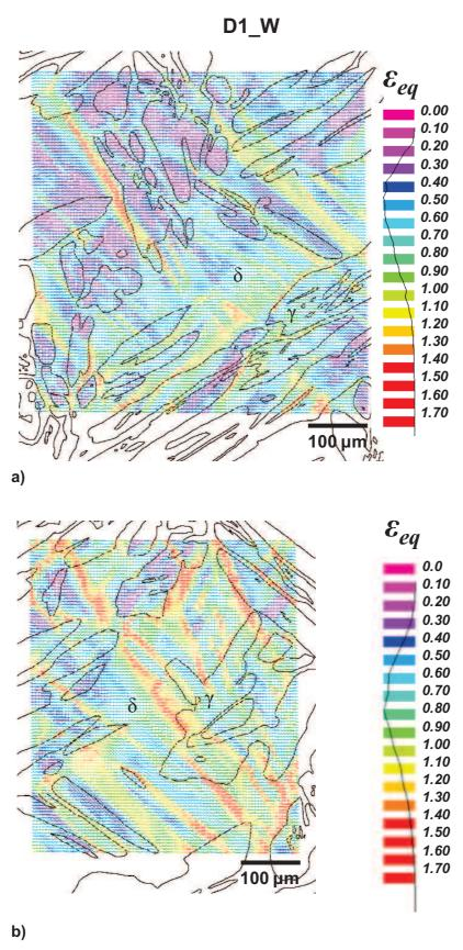
**Figure IV.23.** Equivalent strain distribution maps of the D1\_W microstructure; a) map 1; b) map 2; the equivalent strain map is superimposed with the undeformed microstructure to clearly present where in the microstructure the strains are distributed; the compression axis corresponds to the vertical axis.
