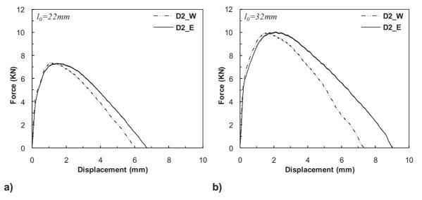
**Figure III.39.** Comparison between typical force-displacement curves (alloy D2) for both austenite morphologies; a)  $l_0=22mm$ ; b)  $l_0=32mm$ .
