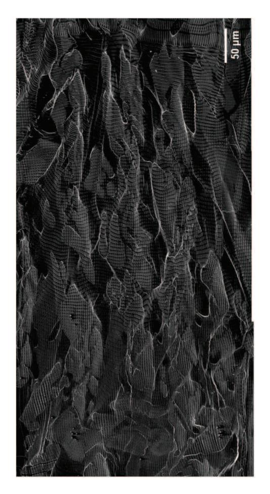
Figure C. 15. Microgrid of the D1\_W microstructure from sample iiii after plane strain compression at 950°C.
