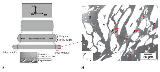
**Figure I.9.** a) Evolution of the transverse dimensions of the hot rolling blocks with increasing reduction; a clear transverse strain develops and cracks have been observed only in the bulged region; b) microstructure in the edge part illustrating the damage; red arrows emphasize the voids.
