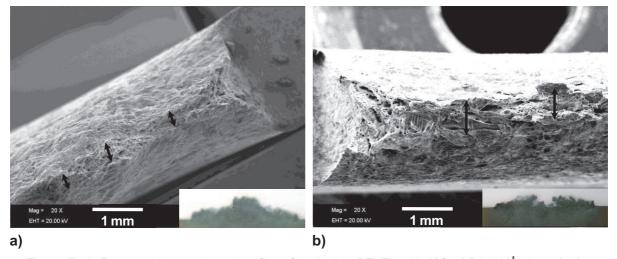
**Figure III.50.** Fracture micrographs and profiles of the broken DENT at 1050°C; a) D1\_W ( $l_0$ =35mm); b) D1bis\_W ( $l_0$ =35mm).
