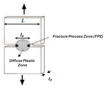
Figure III.1. DENT geometry showing the diffuse plastic zone as well as the localized necking zone in front of the crack tips.
