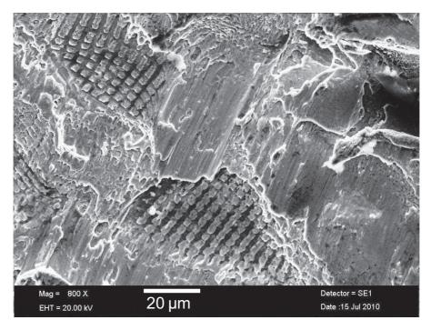
**Figure IV.45.** SEM micrograph showing the deformed microgrids after plane strain compression at 1050°C and 10s<sup>-1</sup>.
