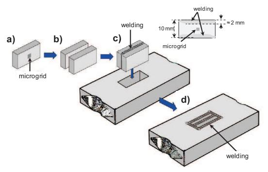
**Figure IV.14.** Preparation of the modified plane strain compression sample; a) microgrid sample; b) face to face with a similar polished plate; c) assembly with modified plane strain compression specimen; d) welding at top and bottom [97].
