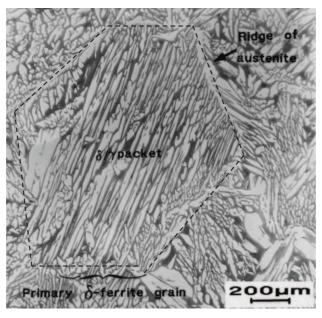
**Figure II.1.** As-cast microstructure in a conventional 2304 duplex stainless steel; the dotted lines indicate the primary δ-ferrite grain, allotriomorphic austenite decorates the primary δ-ferrite grain boundaries and Widmanstätten austenite appears inside the primary δ-ferrite grain [12].
