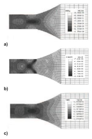
**Figure IV.33.** Finite elements predictions of given parameters at nominal equivalent strain of 1 for frictionless deformation of a 316L-austenitic stainless steel specimen with  $h_{\theta}$  = 10 mm,  $\dot{\varepsilon}$  = 10s<sup>-1</sup> and T=1000°C; a) equivalent strain; b) equivalent strain rate; c) temperature distributions [130].
