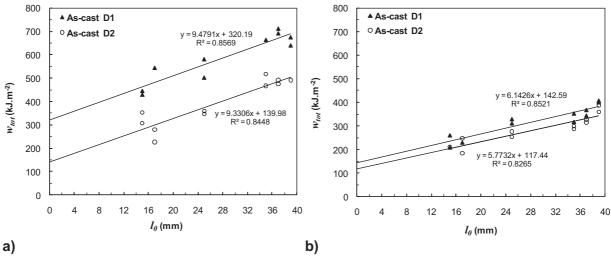
**Figure III.12.** Variation of the total specific work of fracture as a function of the ligament length for separation of the essential work of fracture; comparison between the two grades D1 and D2 in the as-cast conditions; a) T=1050°C; b) T=1200°C.
