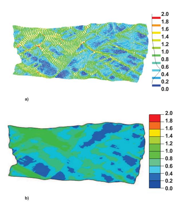
**Figure IV.49.** Equivalent strain distribution; a) experimental; b) computed by FE model for the best solution. The displacement profile on the edges is in good agreement with the experimental. Clearly, the strain localization is more in ferrite than in austenite. The compression is applied vertically.
