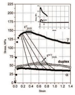
**Figure II.15.** Results of the hot torsion test performed at 1200°C and 1s<sup>-1</sup> for a single ferritic, a single austenitic and a duplex stainless steel [48].
