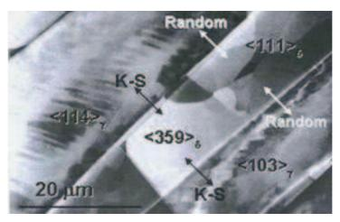
**Figure II.10.** STEM channeling picture and crystallographic orientation analysis; as-cast duplex stainless steel deformed to 1.6 at 1000°C and 1s<sup>-1</sup> [5].
