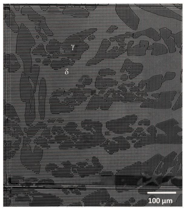
**Figure C. 8.** High resolution SEM micrograph of the D1\_W microstructure in the undeformed configuration; sample iiii. The compression will be applied vertically.
