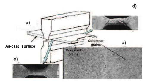
**Figure II.22.** Plane strain compression at 1000°C and 1s<sup>-1</sup> in order to test the effect of the macrostructure on the crack formation; a) schematic view showing the position of the specimen on the machine; b) view of the as-cast microstructure seen on the transverse section of the specimen; c) level of defect on the equiaxed grain side; d) level of defect on the columnar grain side [20].
