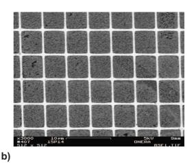
**Figure IV.4.** a) Illustration of the grain boundary sliding after creep at 750°C in nickel-based super alloy thanks to HfO<sub>2</sub> microgrids (step of 5μm); b) HfO<sub>2</sub> grid after 1000h at 750°C under vacuum (SEM, Back-scattered electron mode) [103].
