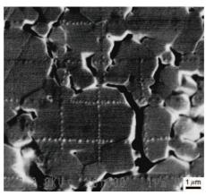
**Figure IV.3.** SEM micrograph (secondary electron mode) showing a MoSi<sub>2</sub> grid after 4h at 1200°C [123].
