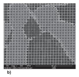
**Figure IV.2.** 5µm-microgrid patterns [103]; a) processing by micro-lithography; b) engraving by chemical etching from this work.
