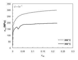
**Figure IV.36.** Comparison between the macroscopic equivalent stress strain curves of the equiaxed morphology obtained under plane strain compression at  $1s^{-1}$  and different temperatures:  $T = 850^{\circ}\text{C}$  and  $950^{\circ}\text{C}$  up to a reduction of 20%.
