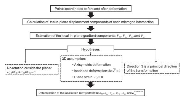
**Figure IV.20.** Procedure to calculate the strain components starting from the coordinates of the grid points.
