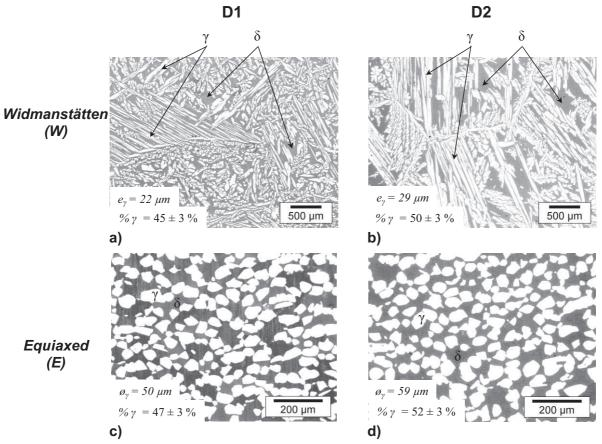
**Figure III.29.** Summary of the model microstructures obtained with the appropriate heat treatments; a) D1 Widmanstätten microstructure after HTW.1; b) D2 Widmanstätten microstructure after HTW.1; c) D1 equiaxed microstructure after HTE.2; d) D2 equiaxed microstructure after HTE.2.
