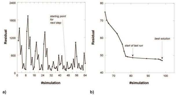
**Figure IV.50.** Evolution of the residual as a function of simulation number a) during the set of 64 simulations and b) during the line search procedure. The last run assures that the residual does not decrease further. It is observed in general that the best solution is achieved within 100 simulations.
