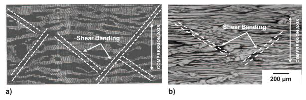
**Figure II.7.** Shear banding development in duplex stainless steel; a) deformed mesh obtained via finite element modeling after simulation of a specimen deformed at 1050°C under plane strain compression [16]; b) optical micrograph of a hot-rolled 2304 specimen (77% reduction) [9].
