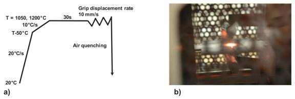
Figure III.6. a) The thermo-mechanical history path followed by the DENT specimens; b) picture showing the shape of the heated zone.
