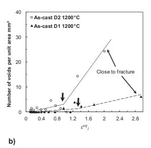
**Figure III.16.** Evolution of the damage as a function of strain for both grades in the as-cast conditions; a) T = 1050°C; b) T = 1200°C. The arrow indicates the strain at which damage starts increasing significantly, i.e. the approximate strain at which damage nucleation occurs.
