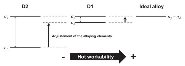
**Figure IV.32.** Schematic illustration of the effect of flow stress differential between ferrite and austenite on the hot workability.
