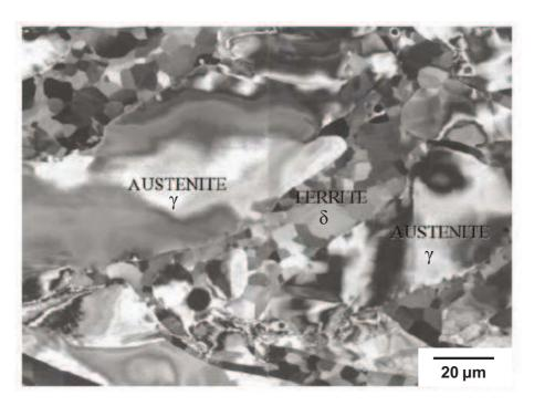
**Figure II.9.** SEM backscattered electron picture; as-cast 2304 duplex stainless steel deformed to 0.4 at 1000°C and 1s<sup>-1</sup> [9].
