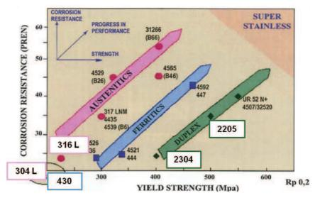
**Figure I.2.** Performance of the different stainless steel families, pitting corrosion resistance and yield strength [2].
