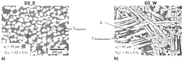
Figure III.38. Generated microstructures with a constant phase ratio but a different austenite morphology; a) Widmanstatten austenite (D2\_W); b) equiaxed austenite (D2\_E).
