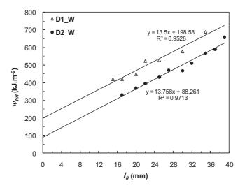
**Figure III.32.** Variation of the specific work of fracture versus ligament length for separation of the essential work of fracture. Comparison between two Widmanstätten microstructures at 1050°C: D1\_W and D2\_W.
