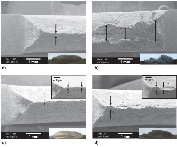
**Figure III.13.** Fracture micrographs and profiles of the broken DENT specimens ( $l_0$  = 37mm); a) D1 at 1050°C; b) D2 at 1050°C; c) D1 at 1200°C. d) D2 at 1200°C. The arrows emphasize the thickness variation in the profile.
