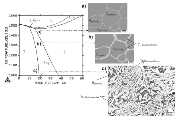
**Figure 1.5.** Origin of the as-cast microstructure in duplex stainless steel; a) at high temperature duplex stainless steel is entirely ferritic; during cooling, the austenite precipitates b) at existing ferrite grain boundaries and c) inside the ferrite matrix with a lath morphology; thermal history explains the as-cast microstructure.
