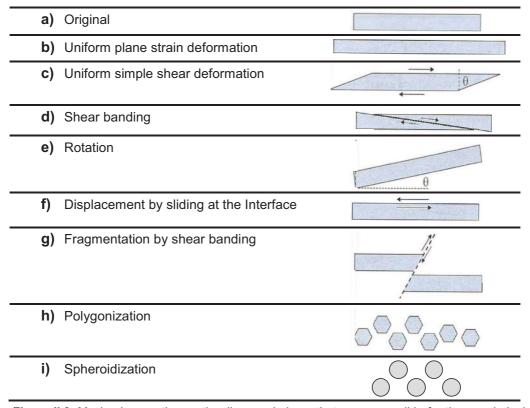
**Figure II.3.** Mechanisms acting on the dispersed phase that are responsible for the morphological and distribution changes undergone by the austenite during hot-working of austeno-ferritic stainless steels [5].
