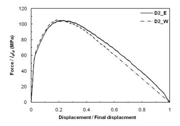
**Figure III.47.** Normalization of the force displacement curves for a ligament length of  $l_0$  = 22mm for respectively, the D2\_E and D2\_W microstructures. The force is normalized by the area of the ligament that gives a stress and the displacement is divided by the final displacement.
