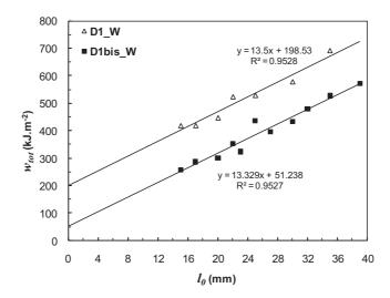
**Figure III.49.** Variation of the specific work of fracture as a function of the ligament length for separation of the essential work of fracture. Comparison between D1\_W and D1bis\_W microstructures at 1050°C.
