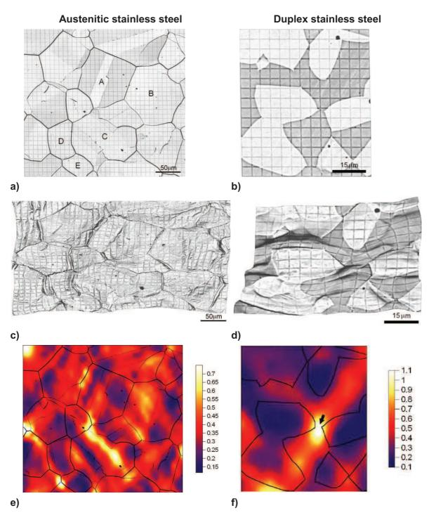
**Figure IV.5.** Results provided by the modified microgrid technique on model stainless steel alloys: austenitic (deformed at 900°C) and duplex (deformed at 850°C); a) & b) microgrids before deformation; c) & d) microgrids after deformation; e) & f) Green-Lagrange equivalent strain Maps [97].
