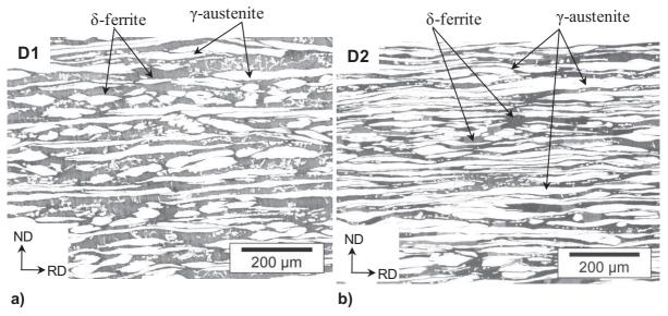
**Figure I.8.** Microstructures of the transfer bar, i.e. just after the roughing-mill operations; a) D1 grade; b) D2 grade;  $\gamma$ -austenite in white, δ-ferrite in grey.
