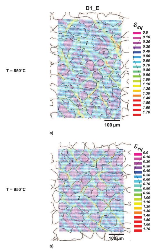
**Figure IV.37.** Equivalent strain distribution maps of the equiaxed morphology: D1\_E at T = 850 and 950°C for a 20% macroscopic thickness reduction; a) strain map at T = 850°C; b) strain map at T = 950°C. The equivalent strain map is superimposed with the undeformed microstructure to clearly present where in the microstructure the strains are distributed. The loading direction corresponds to the vertical axis.
