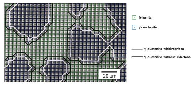
**Figure B. 3.** Integration scheme for the average gradient over a phase; two different polygonal lines are constructed: one called "without interface" and the other referred as "with interface".
