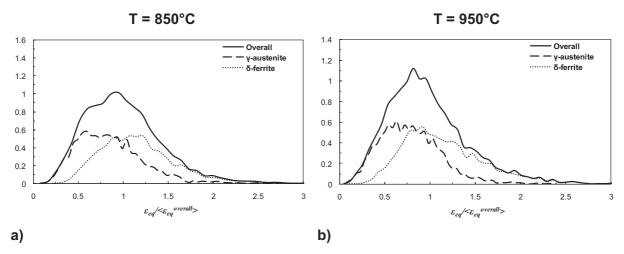
**Figure IV.38.** Strain distribution functions relative to the volume fraction of phase for the equiaxed morphology: D1\_E. a) D1\_E,  $T = 850^{\circ}C$ . b) D1\_E,  $T = 950^{\circ}C$ .
