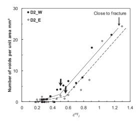
**Figure III.42.** Evolution of the damage as a function of equivalent strain for both austenite morphologies. The arrows indicate the approximate strain at which damage nucleation occurs.
