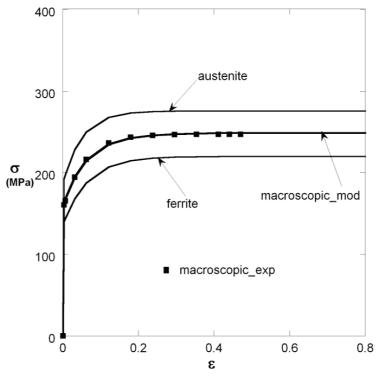
**Figure IV.52.** Flow curves for the macroscopic material and the two phases. The measured data is indicated by solid squares. The simulated macroscopic stress-strain curve is rather well in agreement with the experimental one.
