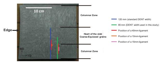
Figure III.7. Illustration of the specimen or ligament position as a function of the dimensions.
