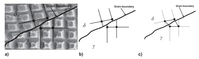
**Figure IV.43.** a) SEM micrograph and b) schematic of sliding at a  $\delta/\gamma$  interphase boundary; and c) shear deformation as interpreted by the strain calculation method, which only takes into account the four corners of each microgrid square.
