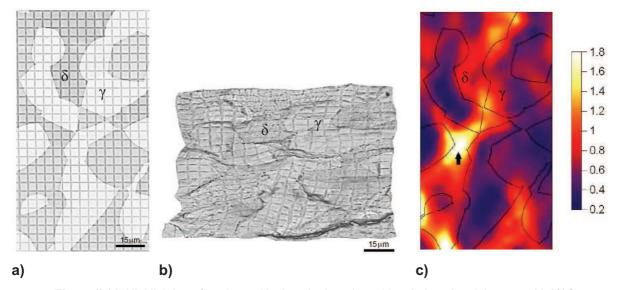
**Figure II.14.** Highlighting of strain partitioning via the microgrid technique in a laboratory 29.6%Cr-11.6%Ni-0.27%Mn duplex steel deformed at 950°C and 1s<sup>-1</sup>; a) undeformed state of a relatively small area; b) deformed configuration of the same area; c) distribution of the Green-Lagrange equivalent Von Mises strain [19].
