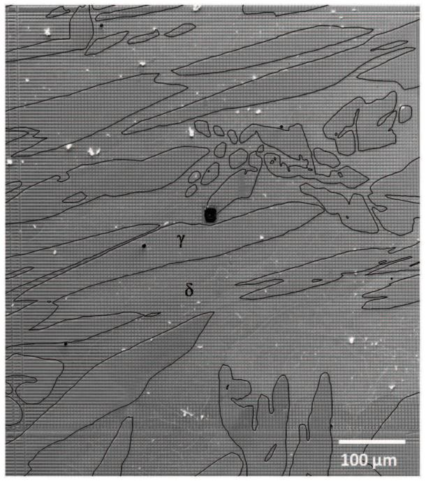
**Figure C. 7.** High resolution SEM micrograph of the D1\_W microstructure in the undeformed configuration; sample ii. The compression will be applied vertically.
