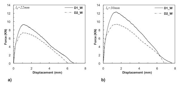
**Figure III.31.** Comparison between typical force-displacement curves of DENT specimens with the same ligament length  $l_{\theta}$  for both grades, D1\_W and D2\_W with a Widmanstätten microstructure; a)  $l_{\theta}$ = 22mm; b)  $l_{\theta}$ =30mm.
