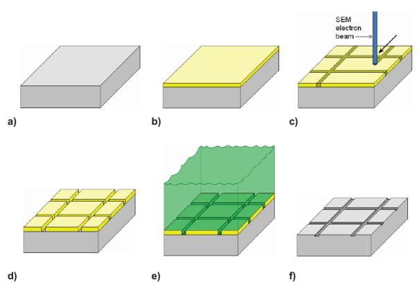
**Figure IV.7.** Steps of modified microgrid technique; a) polishing and electro-etching; b) coating with an electro-sensitive polymer; c) irradiation of the resin with the electron beam; d) dissolution of the irradiated polymer; e) engraving by electro-etching; f) dissolution of the remaining polymer [50].
