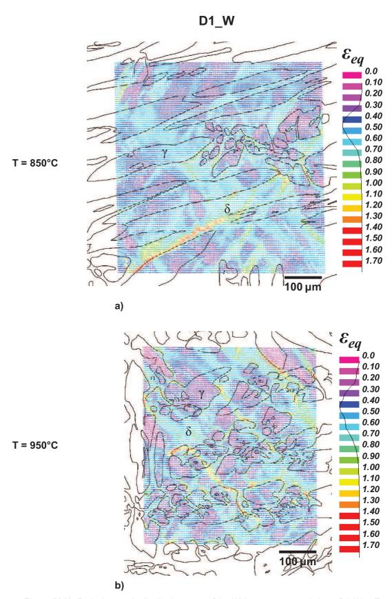
**Figure IV.40.** Equivalent strain distribution maps of the Widmanstätten morphology: D1\_W at T = 850 and 950°C; a) strain map at T = 850°C; b) strain map at T = 950°C. The equivalent strain map is superimposed with the undeformed microstructure to clearly present where in the microstructure the strains are distributed. The loading direction corresponds to the vertical axis.
