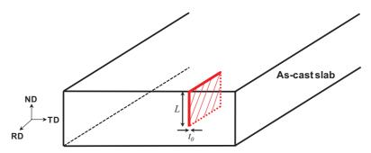
Figure III.10. Schematic the as-cast slab showing where the DENT specimens were machined.
