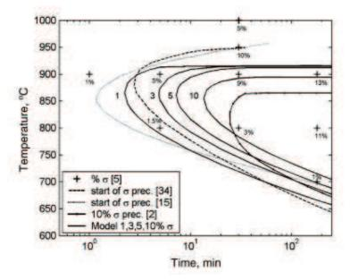
**Figure IV.18.** Time-Temperature-Transformation diagram of a 2205 duplex stainless steels. Illustration of the  $\sigma$  phase isothermal precipitation [69].
