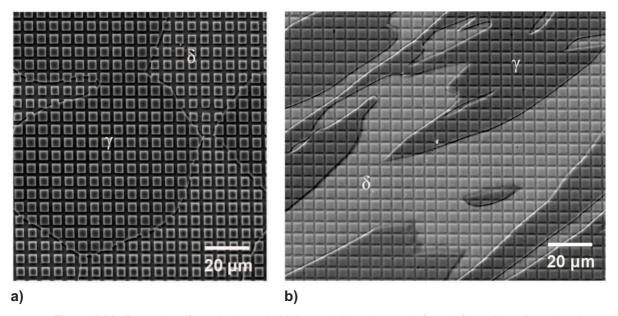
**Figure IV.8.** Examples of good microgrid high resolution pictures before deformation; a) equiaxed morphology; b) Widmanstätten morphology.
