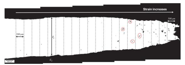
**Figure III.8.** Section perpendicular to the ligament in order to quantify the density of cracks per unit area (mm²) as a function of strain; the dotted lines correspond to the 500μm-step partition; the black arrow shows the position where the thickness was measured to estimate the strain; and the red circled zones highlight a few voids.
