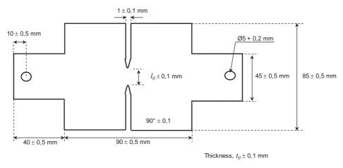
**Figure III.5.** Dimensions of the DENT (Double Edge Notch Tension) specimens used,  $t_0$  = 3mm.
