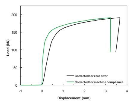
Figure A.3. Machine compliance corrections.
