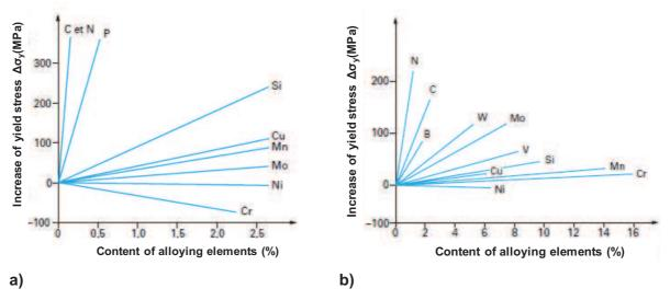
**Figure IV.31.** Influence of alloying content on the yield stress of a) ferrite and b) austenitic stainless steel at room temperature.
