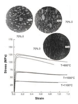
**Figure II.17.** Influence of the phase morphology on the flow stress of duplex stainless steel with 70%  $\delta$  deformed under uniaxial compression at different temperature at a strain rate of 0.03s<sup>-1</sup> [51].
