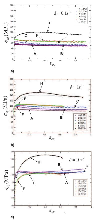
**Figure II.11.** Equivalent flow stress strain curves of different duplex stainless steels deformed under plane strain compression at 1050°C and at different strain rates; a) 0.1s<sup>-1</sup>; b) 1s<sup>-1</sup>; 10s<sup>-1</sup>. The value between the parenthesis gives the austenite content [42].
