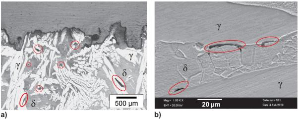
**Figure III.15.** a) Optical micrograph and b) SEM micrograph of a region close to the fracture of a DENT specimen deformed at 1050°C. Voids nucleate by a partial decohesion of the  $\delta/\gamma$  interface, see circled red areas.
