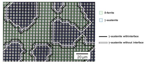
Figure IV.21. Integration scheme for the average gradient over a phase
