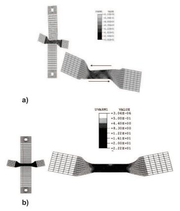
**Figure IV.12.** Possible problems encountered during plane strain compression; a) Z shape deformed specimen due to initial platen misalignment; b) U shape deformed specimen with different friction coefficients at the top and bottom tools [127].
