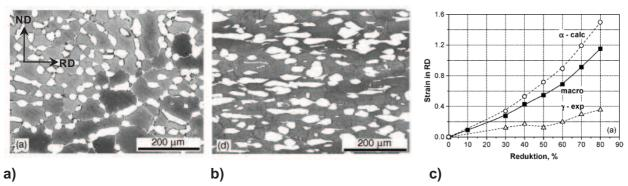
**Figure II.13.** Microstructure evolution during hot rolling at 1250°C for reduction a) 0% and b) 80%. Initially austenite equiaxed islands are embedded in a ferrite matrix. During hot rolling, these islands become more elongated in the rolling direction. c) Strain partitioning in the rolling direction, austenite seems to accommodate only a fraction of the applied strain [48].
