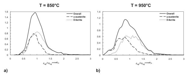
**Figure IV.41.** Strain distribution functions relative to the volume fraction of phase for the Widmanstätten morphology: D1\_W. a) D1\_W, T = 850°C. b) D1\_W, T = 950°C.
