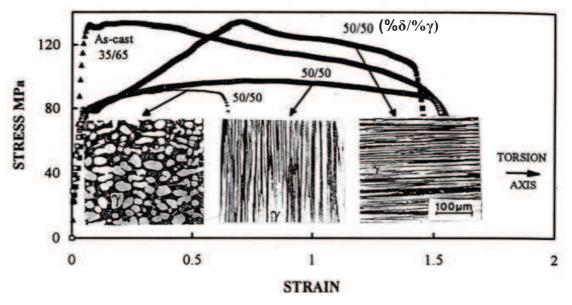
**Figure II.18.** Influence of the phase morphology and phase orientation on the flow stress of a 2304 duplex stainless steel deformed under torsion at 1000°C at a strain rate of 1s<sup>-1</sup> [11].
