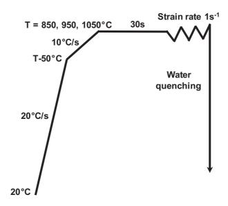
Figure IV.17. Thermo-mechanical path undergone by the plane strain compression specimens.
