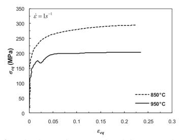
**Figure IV.39.** Comparison between the macroscopic equivalent stress strain curves of the Widmanstätten morphology obtained under plane strain compression at 1s<sup>-1</sup> and different temperatures: T = 850°C and 950°C up to a reduction of 20%.
