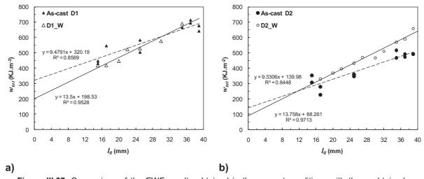
**Figure III.37.** Comparison of the EWF results obtained in the as-cast conditions with those obtained starting from model Widmanstätten microstructures at T=1050°C; a) Alloy D1; b) Alloy D2.
