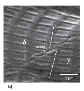
**Figure IV.42.** Illustration at different magnifications and different locations of the  $\delta/\gamma$  sliding mechanism occurring along the incoherent interface boundaries in the equiaxed microstructure.
