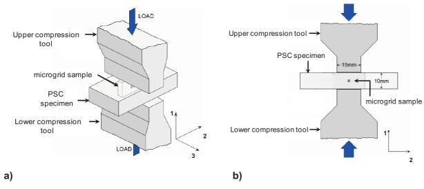
**Figure IV.16.** Schematic views of the microgrid sample inserted into the plane strain compression specimen and the compression tools during the tests; a) asymmetric view; b) plane view.
