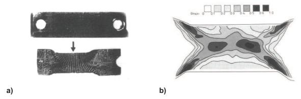
**Figure IV.34.** Investigation of the strain heterogeneity during plane strain compression test with the engraved grid technique, nominal strain = 0.33 and  $w/h_0$  = 2; a) engraved grid before and after deformation; b) average equivalent strain distribution [132].
