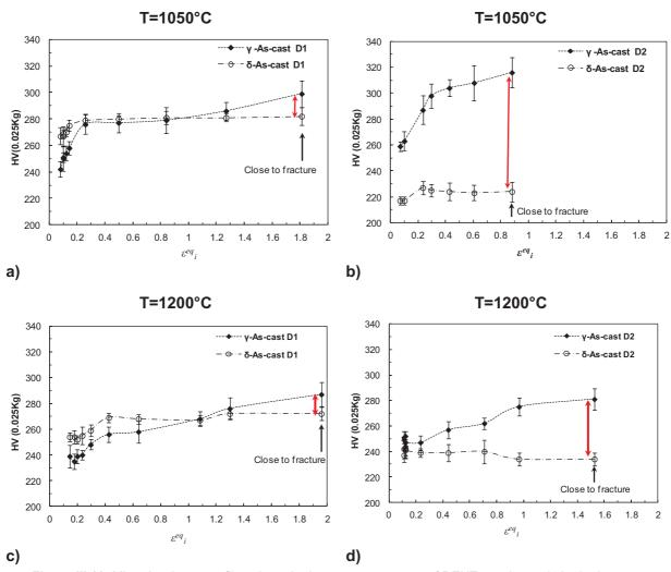
**Figure III.18.** Micro-hardness profiles along the homogeneous zone of DENT specimens in both phases; a) alloy D1, T=1050°C; b) alloy D2, T=1050°C; c) D1, T=1200°C; d) D2, T=1200°C. It is considered that there was no significant gradient of temperature along the region where the hardness tests were performed.
