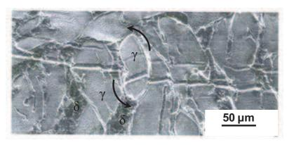
**Figure II.6.** SEM picture showing the rotation of an austenite grain highlighted by the displacement of the scratch markers at the specimen surface; as-cast 2304 duplex stainless steel deformed under torsion to 1.6 at 1000°C and 1s<sup>-1</sup> [13].
