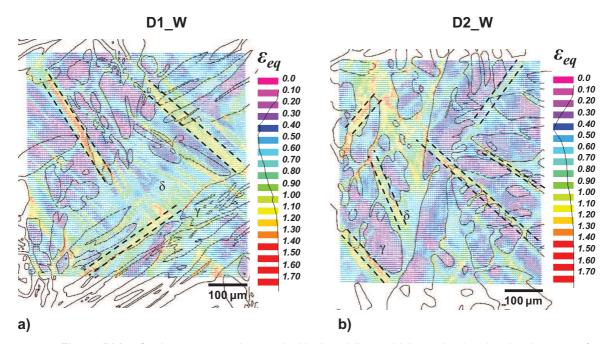
**Figure IV.27.** Strain maps superimposed with dotted lines which emphasize the development of shear bands; a) map 1 in D1\_W; b) map 2 in D2\_W.
