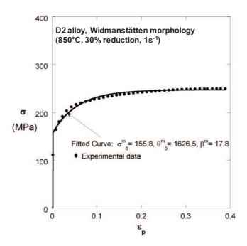
**Figure IV.48.** Macroscopic equivalent true stress-strain curve of D2 alloy presenting a Widmanstätten morphology measured during plane strain compression test at 850°C and 1s<sup>-1</sup>. Thick curve is the fit to Kocks-Mecking hardening law, see eq IV-12. The superscript 'm' means macroscopic.
