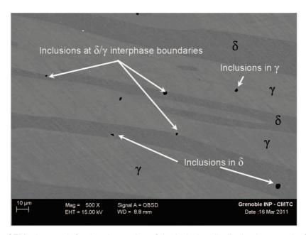
Figure III.9. SEM micrograph for the observation of the inclusion distribution in austenite-ferrite microstructures.
