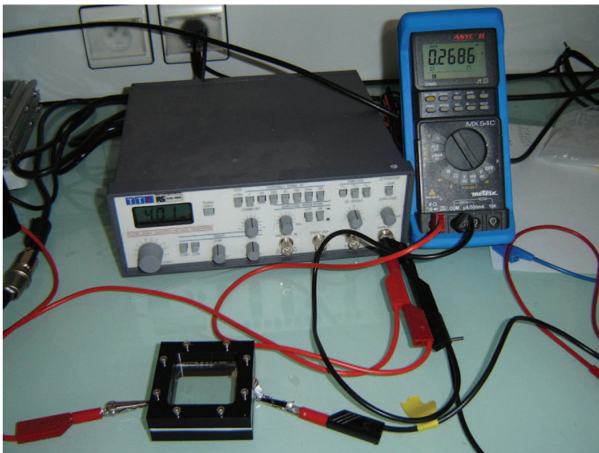
Figure 4.2: Complete chamber when formation of vesicles takes place
