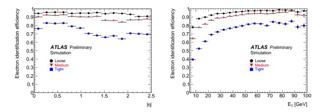
Figure 5.2: Identification of the electrons obtained on  $Z \to ee$  Monte Carlo samples, for the three default set of cuts, Loose, Medium and Tight. As a function of  $|\eta|$  (left) and  $E_T$  (right) [129].
