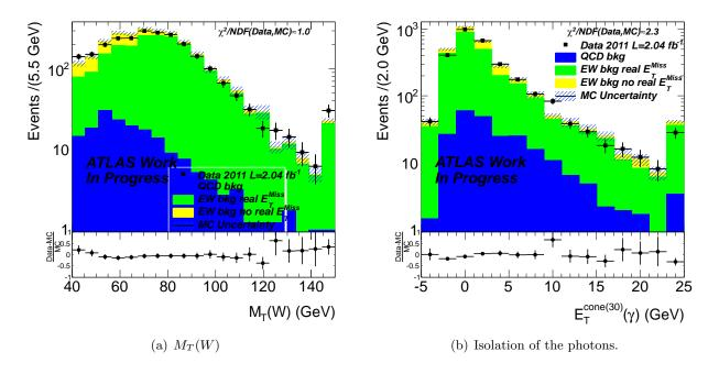
Figure 5.12: Control distributions obtained adding the QCD background template, for  $M_T(W)$  (left) and  $E_T^{\text{cone}(30)}(\gamma)$  (right).
