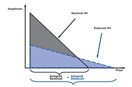
Figure 3.20: The triangular LAr signal in the case where the HV is nominal and non nominal.
