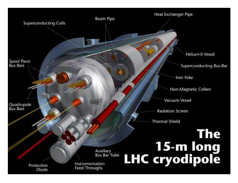
Figure 2.2: Sectional view of one LHC dipole, CERN<sup>©</sup>.
