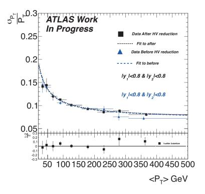
Figure 4.29: Jet fractional transverse momentum resolution for jets belonging in the |y| < 0.8 bin. The graph show the differences for the period before the PS HV was reduced and after. The results are shown for the bisector method. Data after the reduction are in black and data before the reduction are in blue.
