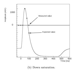
Figure 3.29: Sketch of a LAr pulse shape. The digitization is saturated. (a) The expected maximum sample is shown as well as the measured one. (b) The expected minimum samples are shown, as well as the measured one.
