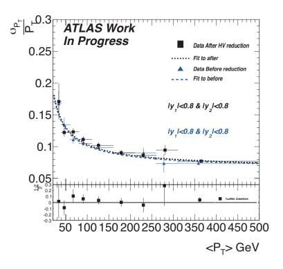
Figure 4.30: Jet fractional transverse momentum resolution for jets belonging in the |y| < 0.8 bin. The graph show the differences for the period before the PS HV was reduced and after. The results are shown for the di-jet balance method. Data after the reduction are in black and data before the reduction are in blue.
