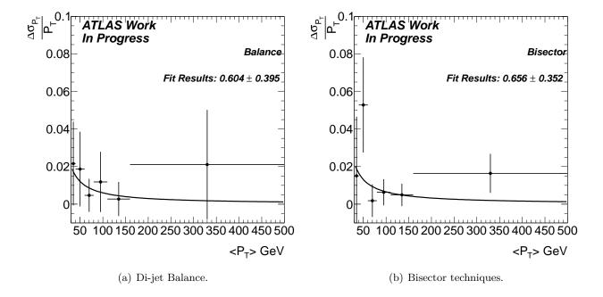
Figure 4.33: Resolution absolute difference between the first HV Ratio bin and the most divergent one as a function of  $\langle p_T \rangle$ .
