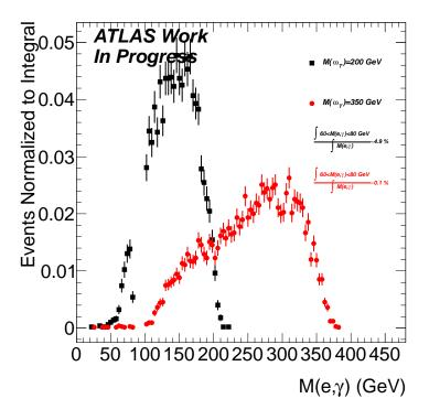
Figure 5.24: Invariant mass between photon and electron, for the LSTC sample mode T200 (black) and T350 (red).
