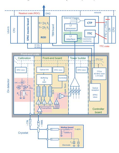
Figure 3.13: Block diagram of the LAr readout chain [66].
