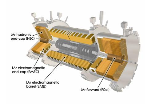
Figure 3.1: Cut view of the LAr Calorimeters. The Inner Detectors and the beam pipe are also visible in the center of the image [66].
