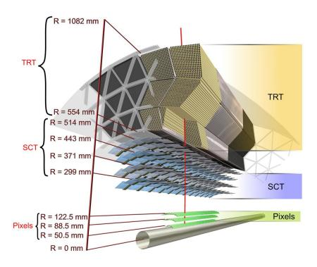
(b) Sectional view of the barrel Inner Detector. The straight line in the middle of the figure represent a 10 GeV track with  $\eta=0.3$ .
