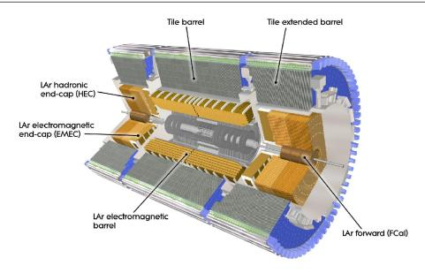
Figure 2.11: Atlas Calorimeter systems [66].
