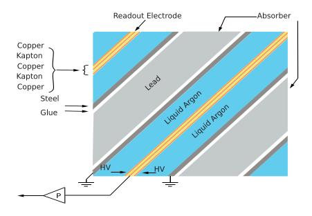
Figure 3.3: Schematic view of the EM LAr calorimeter principle [83].
