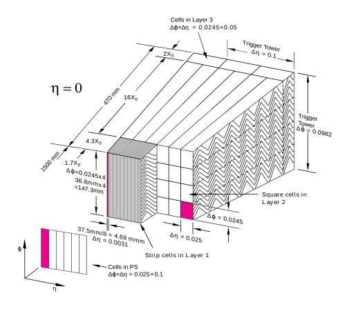
Figure 3.5: Segmentation of the LAr EM barrel calorimeter at  $|\eta| = 0$ . The size of the cells and interaction length for each layer is quoted [66].
