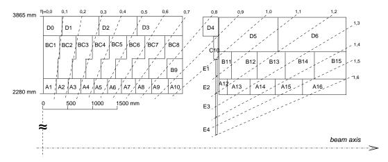
Figure 2.13: Sketch of the Atlas Tile Calorimeter system [66].
