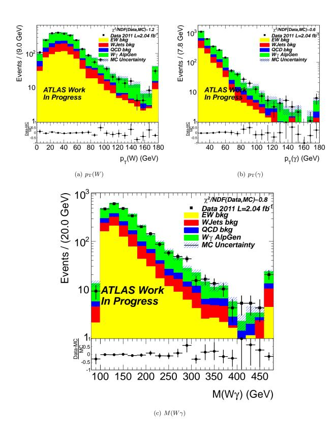
Figure 5.25: Distribution of  $p_{\rm T}(W)$  (a),  $p_{\rm T}(\gamma)$  (b) and  $M(W\gamma)$  (c) in the control region  $p_{\rm T}(\gamma)$  < 60 GeV or  $p_{\rm T}(W)$  < 60 GeV.
