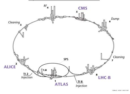
Figure 2.3: Schematic view of the underground LHC complex. The access point and the experiments are visible. CERN<sup>©</sup>.
