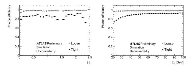
Figure 5.3: Identification of the photons obtain on MC for the two default set of cuts, Loose and Tight. As a function of  $|\eta|$  (left) and  $E_T$  (right). [130]
