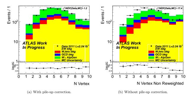
Figure 5.1: Number of reconstructed vertices with (a) and without (b) the Pile-Up reweighing correction.
