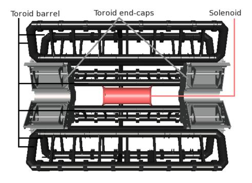
Figure 2.8: Atlas Magnet system. The solenoid magnet is present in the middle of the image. The toroidal magnet barrel are surrounding it. The toroidal end caps magnets are disposed on each side of the solenoid magnet.
