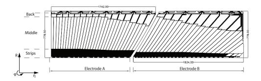
Figure 3.6: Arrangement of the LAr electrodes in the barrel ensuring the coverage up to  $|\eta| < 1.4$  [66].
