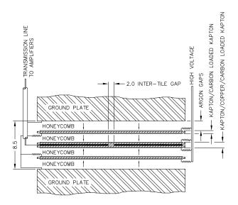
Figure 3.10: Schematic view of one HEC electrode. A preamplifier is located in the cryostat to reduce the electronic noise [83].
