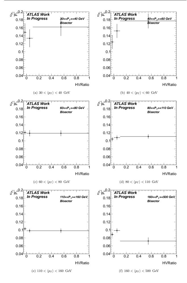
Figure 4.32: Jet fractional transverse momentum resolution measured vs the variable HV Ratio, for different  $\langle p_T \rangle$  bins. Results obtained using the bisector technique.
