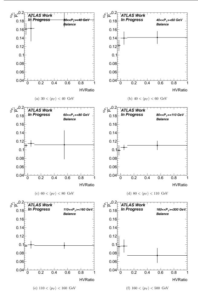
Figure 4.31: Jet fractional transverse momentum resolution measured vs the variable HV Ratio, for different  $\langle p_T \rangle$  bins. Results obtained using the balance method.
