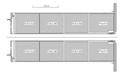
Figure 3.12: Cut view of one FCal. The three modules can be seen. The last layer or "plug" is a shielding [66].
