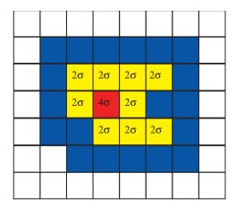
Figure 4.3: Sketch view of a 4/2/0 TopoCluster. The seeding cell with an energy greater than  $4\sigma$  of the pedestal value is drawn in red. The neighbors cells with an energy greater than  $2\sigma$  in yellow, and finally their direct neighbors entering in the cluster energy calculation are drown in blue.
