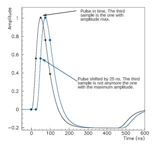
Figure 3.26: Sketch of a LAr pulse shapes. The black one has the proper timing, the blue one is shifted by 25 ns with what is expected.
