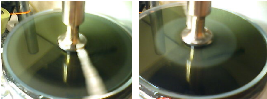
(b) Positive voltage +500 VDC. The particles migrated toward the edge (c) Negative voltage -500 V DC. The particles migrated toward the center
