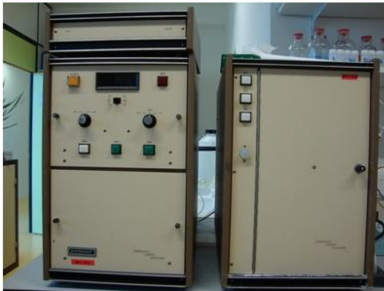
Photo II-1. System used for the determination of the soil microbial C biomass. A: vacuum incubator along with vacuum pump. B: Total carbon analyzer (Dohrman DC80) used to determine the concentration of organic carbon in solution
