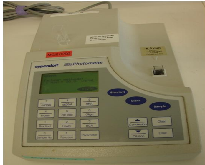
Photo II-5. Spectrophotometer (Biophotometer, Eppendorff) for the estimation of DNA amount
