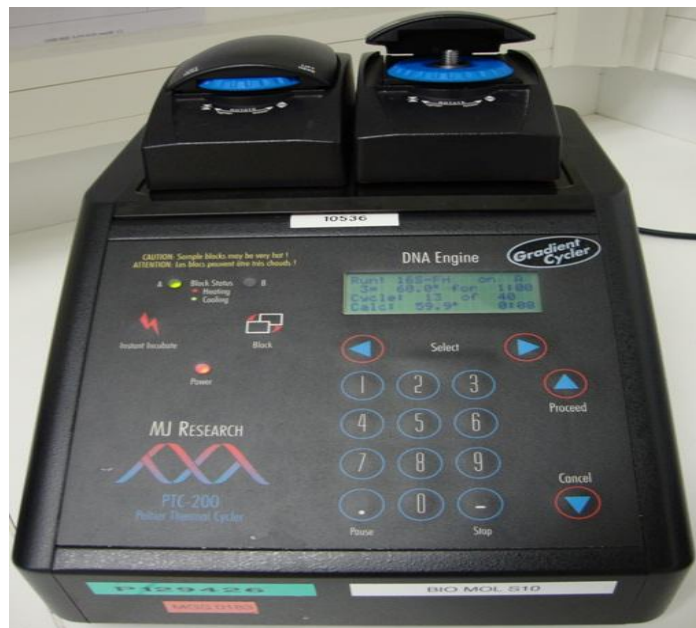
Photo II-6. PTC 200 gradient thermocycler (MJ Research)
