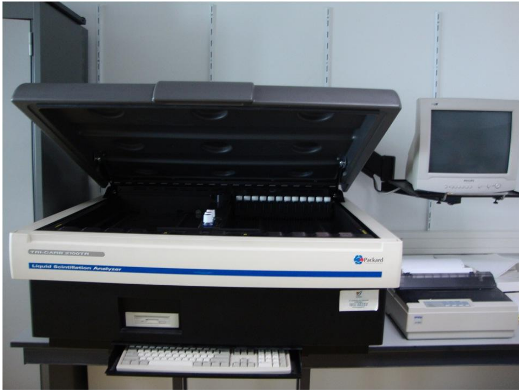
Photo II-2. Packard (Tri-Corb 2100 Tr) liquid scintillation counter for the determination of radioactivity
