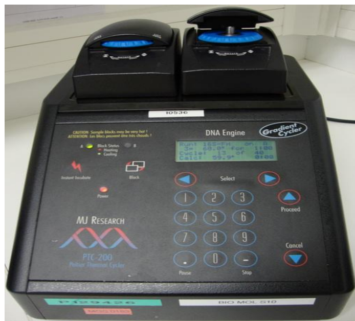
Photo II-6. PTC 200 gradient thermocycler (MJ Research)
