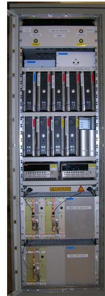
Fig. 3: Photograph of the fully equipped 19" cabinet especially developed for the IRINA project final qualification in the OSIRIS reactor.
