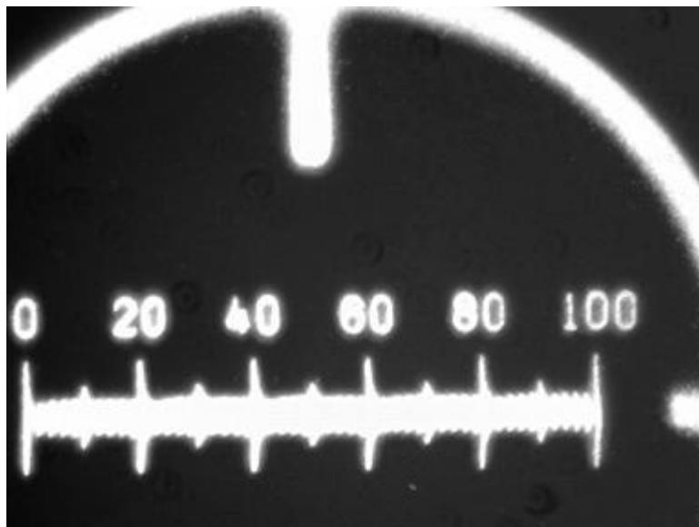
**Figure 24** *100 micrometer scale seen by the CCD camera in the objective focal plan.*
