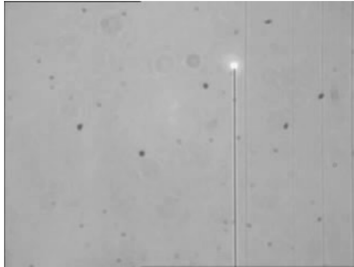
Figure 25 Example of spot visualisation of the laser spot on the material surface during laser nanostructuring.
