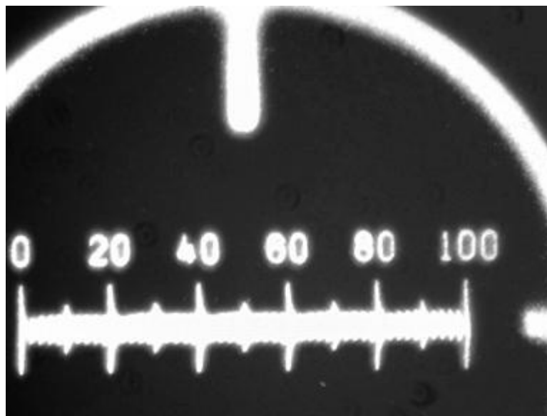
Figure 24 100 micrometer scale seen by the CCD camera in the objective focal plan.
