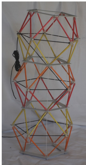
Fig. 5.7: Deployment control by one single cable (black stream: active cable, white strings: passive cables)
