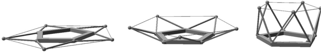
Fig. 4.8: Post-packed phenomenon: flipping up the bracings
