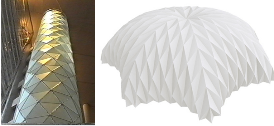
Fig. 2.11: Foldable tube (exhibition object) and dome (paper model) with the Yoshimura pattern [Yoshimura]
