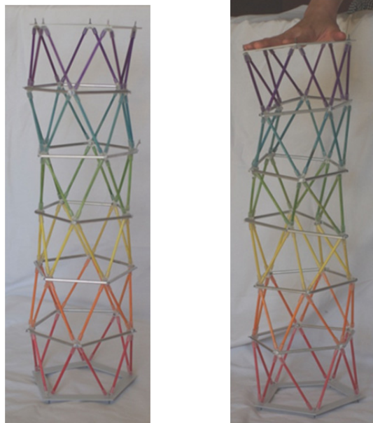
Fig. 5.4: Non-stiffened pentagonal structure — locking during packing
